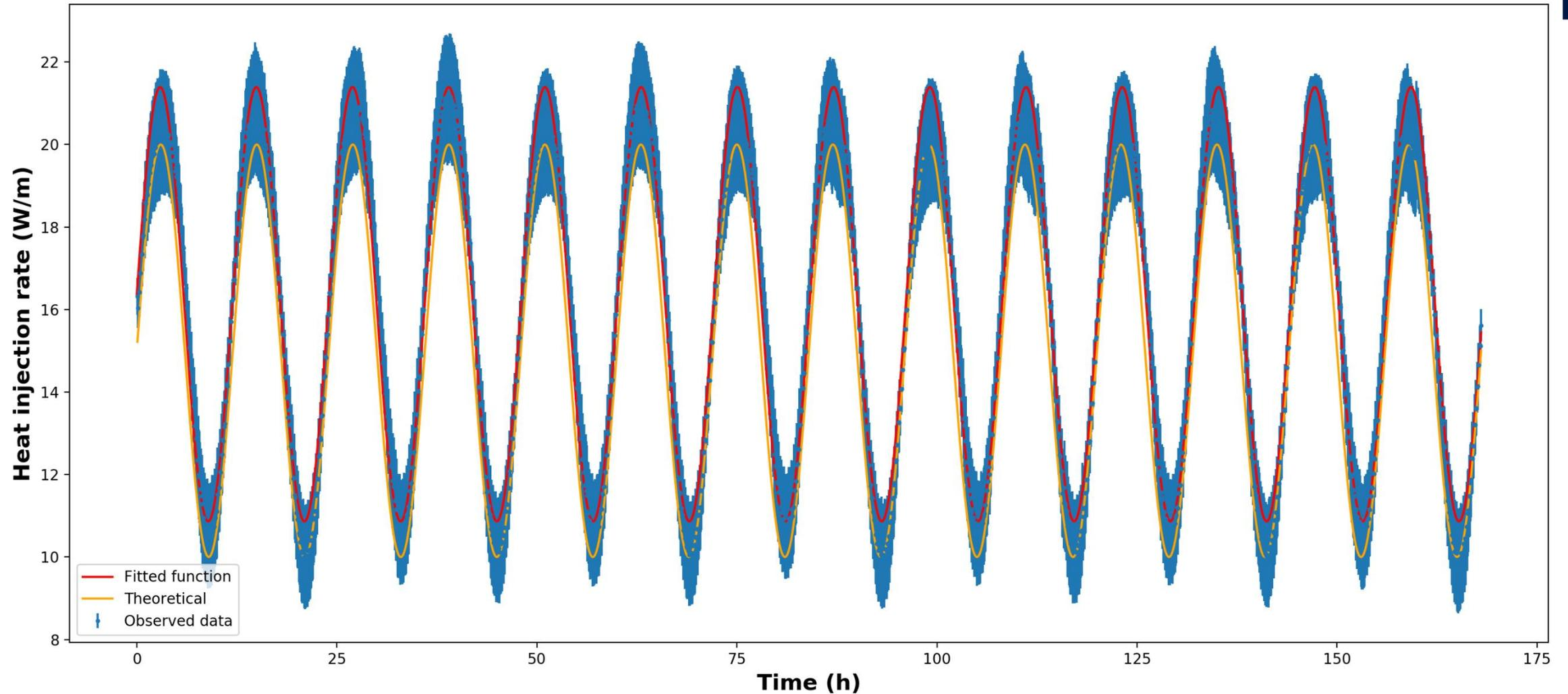
**Figure 12 – Heat injection rate of the OTRT with heating cable performed in the BHE. Comparison among observed data (blue), the mathematical fit following a perfect sinusoidal function (red), and the theoretical power imposed at the power controller.**
