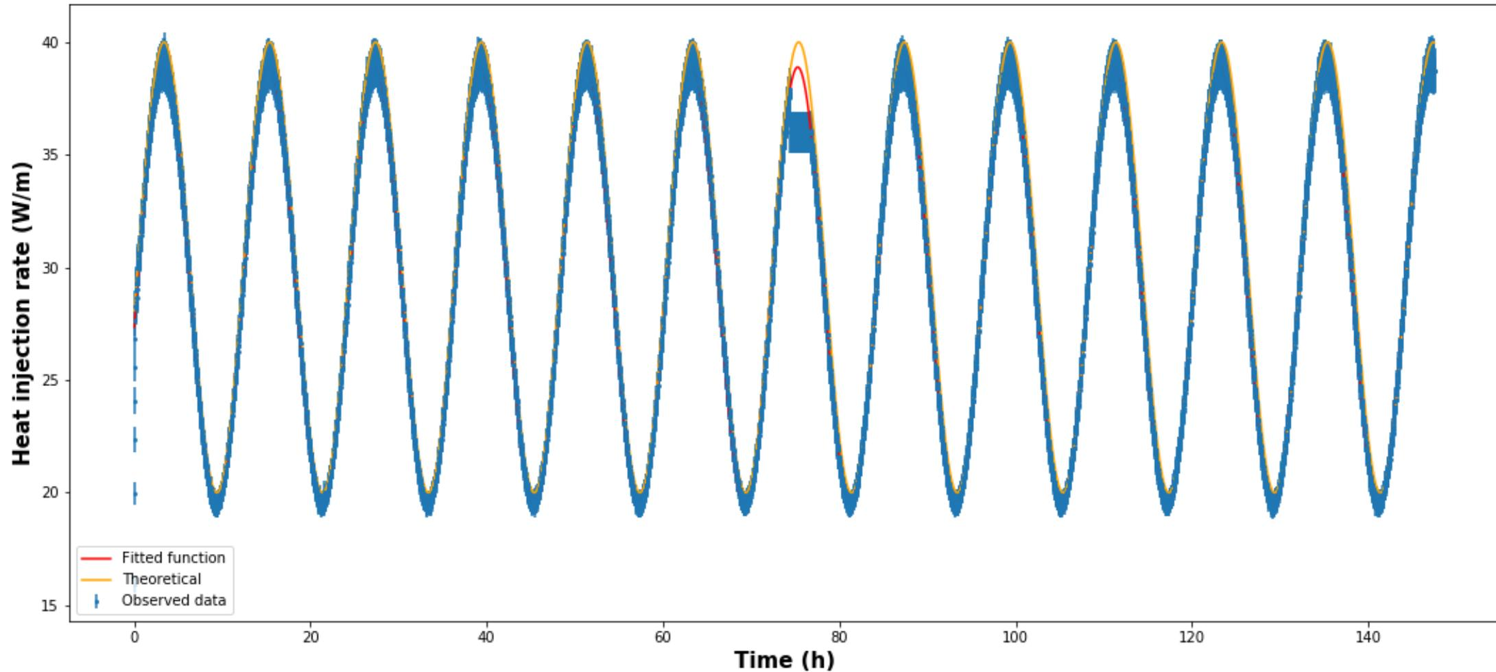
Figure 14 – Heat injection rate of the OTRT with water circulation. Comparison among observed data (blue), the mathematical fit following a perfect sinusoidal function (red), and the theoretical power we asked to Energie-Stat (yellow).
