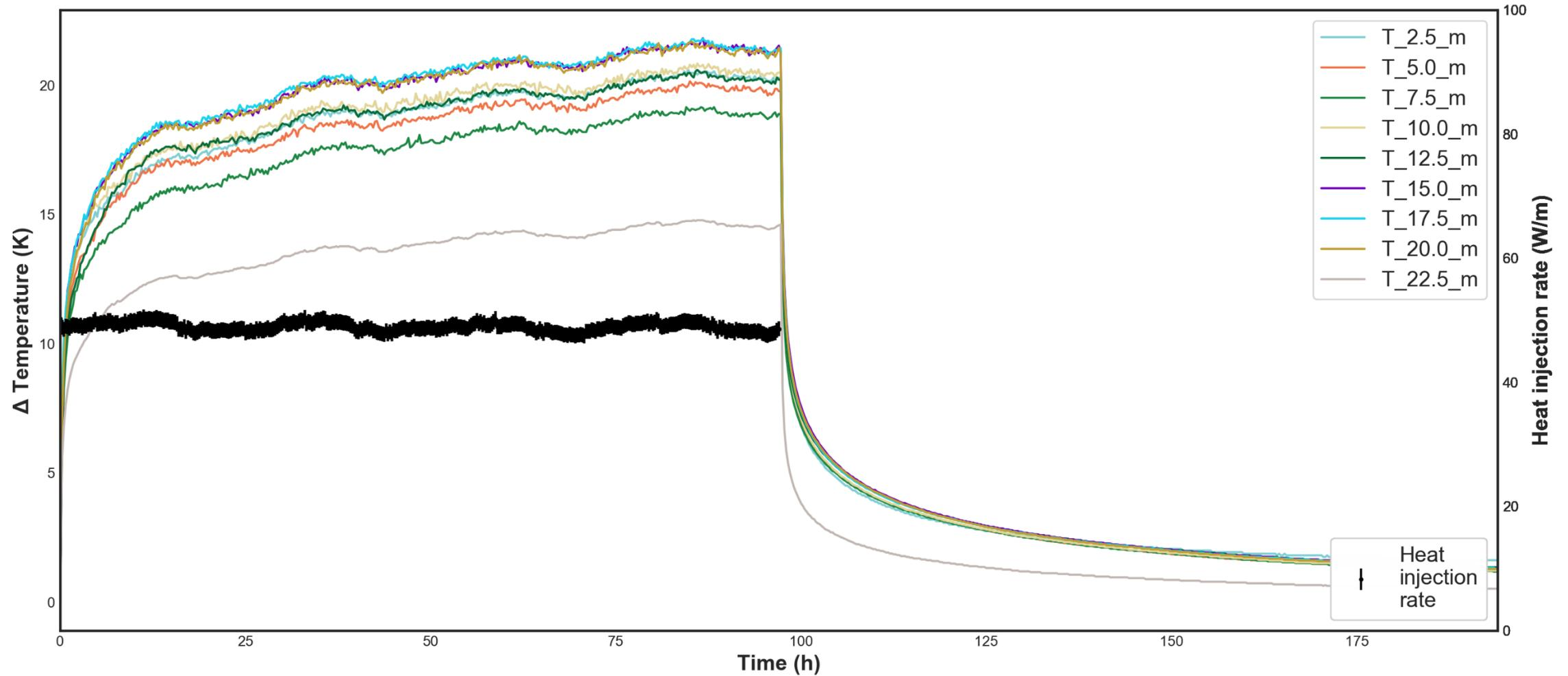
Figure 19 – Results of the conventional TRT with heating cable in the 1-U BHE.
