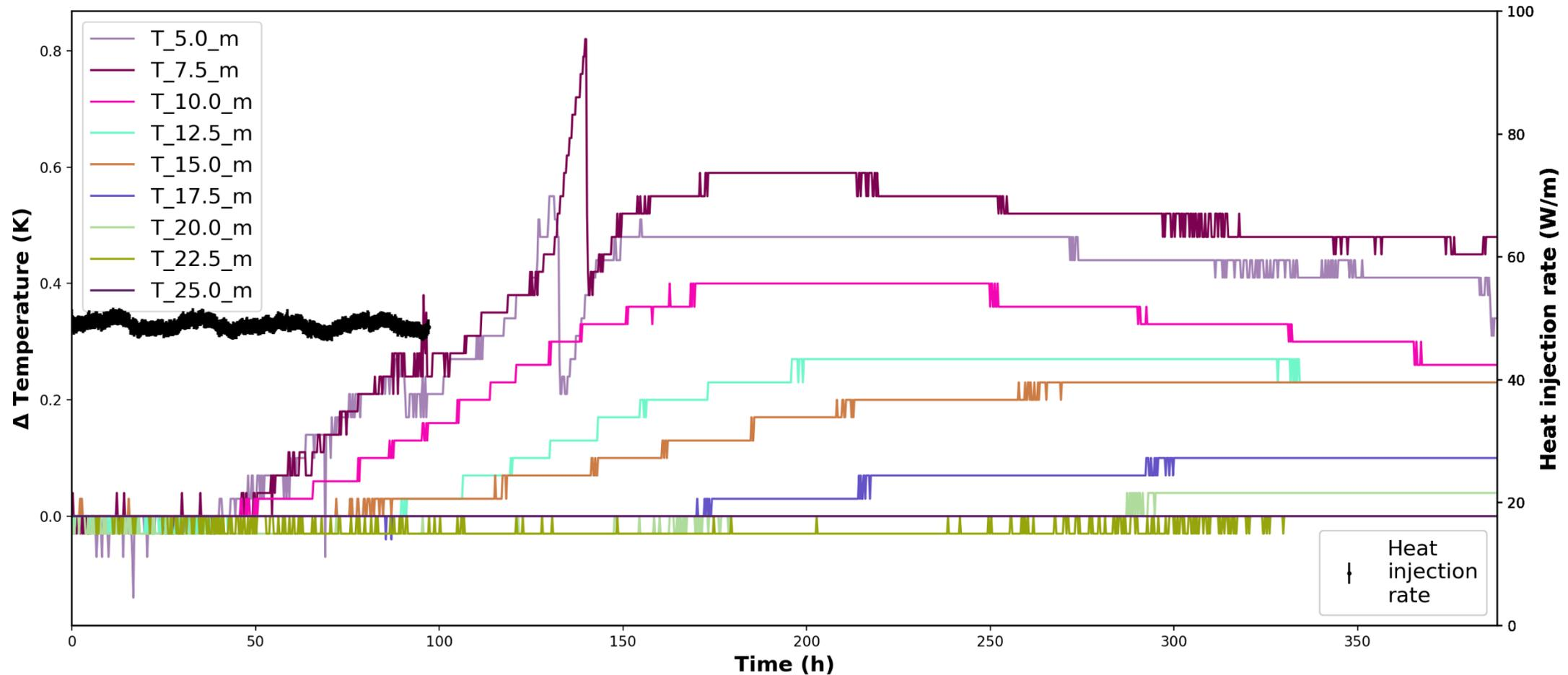
**Figure 21 – Temperature response in the observation well obs4. The black line shows the duration and magnitude of the power injection, same as in Figure 17.**
