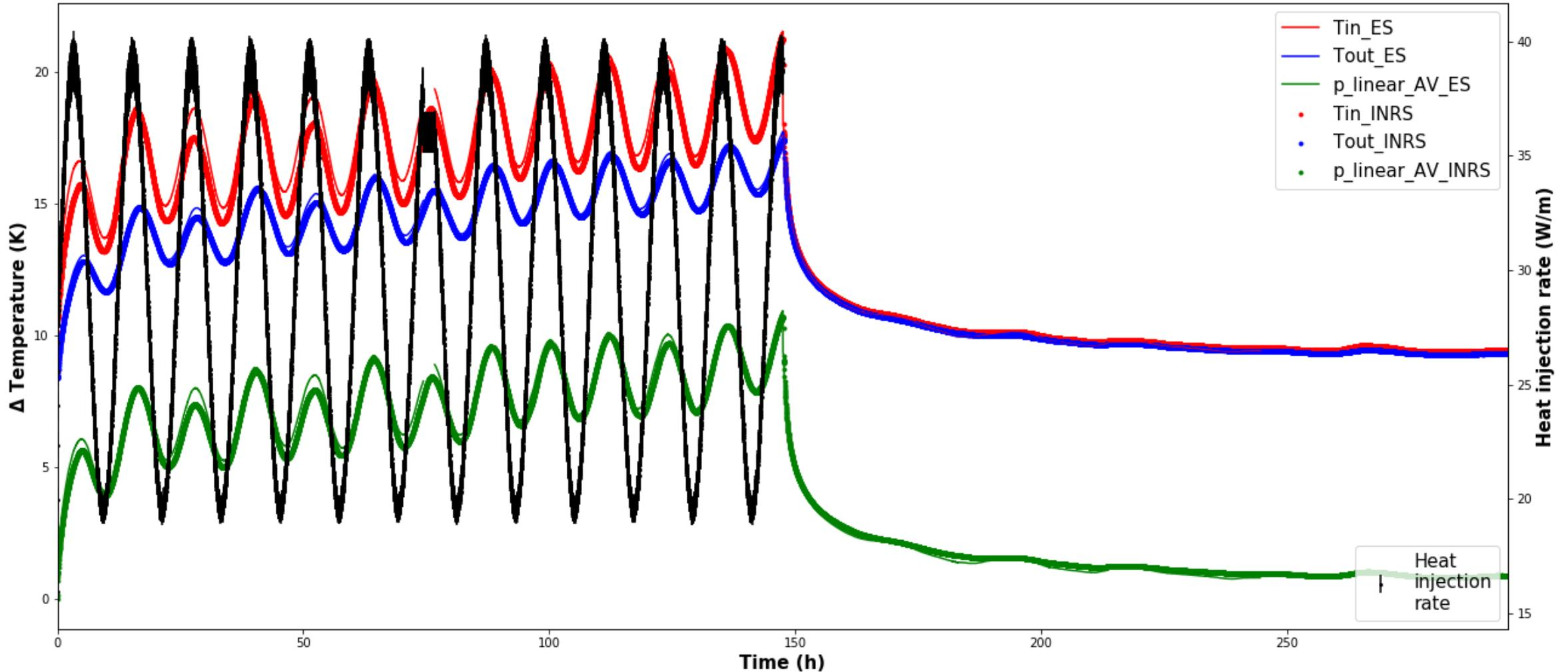
Figure 29 – OTRT analysis of the test with water circulation
