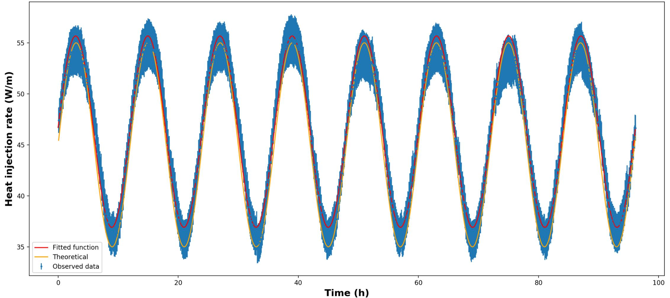
**Figure 11 – Heat injection rate of the OTRT with heating cable performed in open well obs2. Comparison among observed data (blue), the mathematical fit following a perfect sinusoidal function (red), and the theoretical power imposed at the power controller.**
