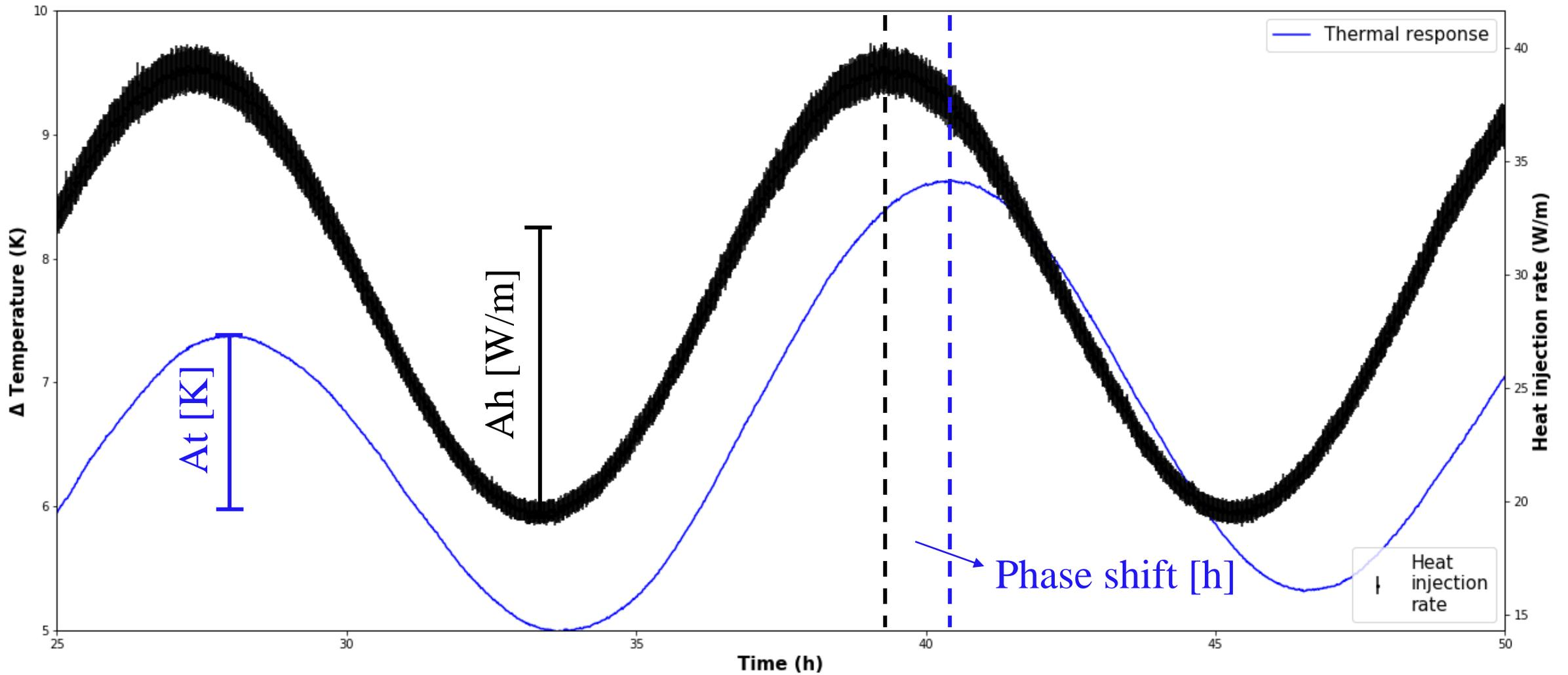
Figure 5 – Oscillatory heat injection (black line) and thermal response (blue line).
