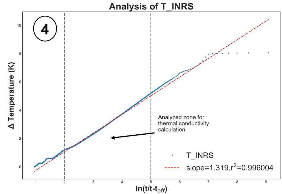
Figure 31 – OTRT analysis of the test with water circulation. Example from INRS sensors. Figure 3 is cut at ca. 60 h.
