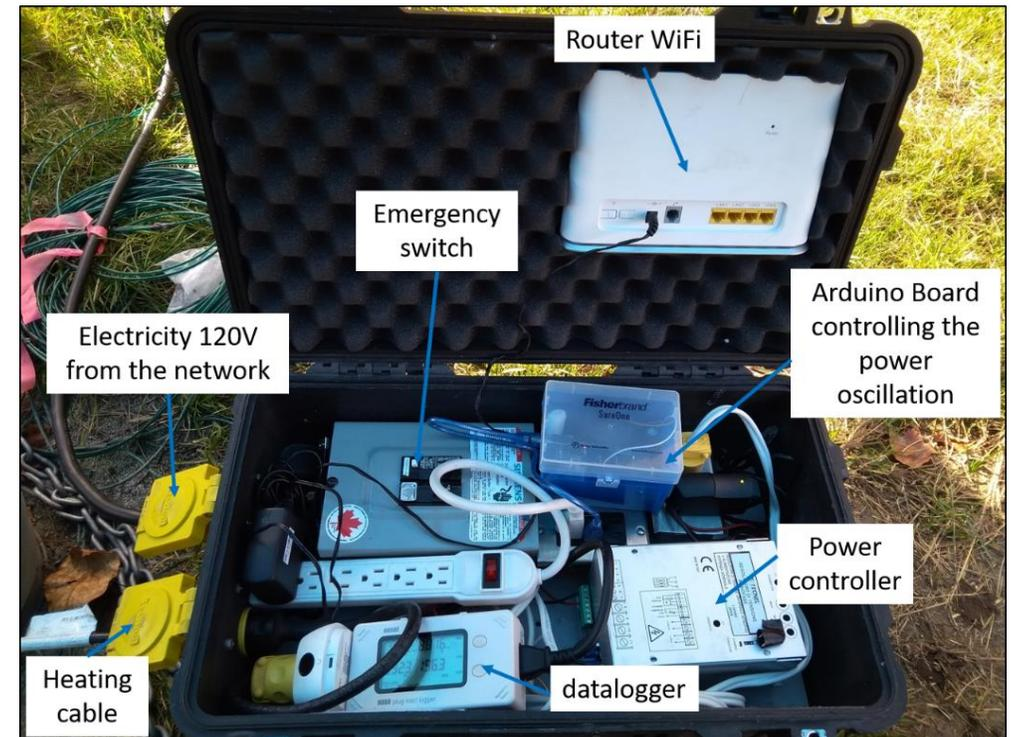
Figure 8 – Pictures of the field site during the TRT (left) and details about the heat injection unit (right).
