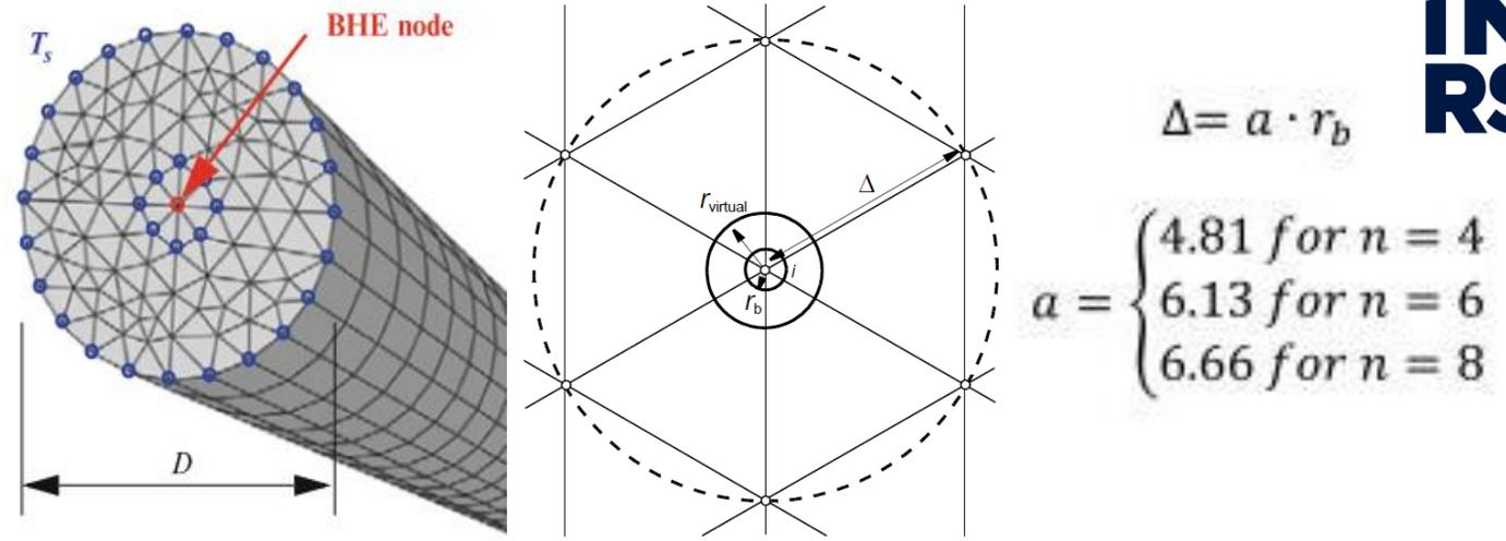
Figure 17 – Critical radius and mesh refinement criteria for BHE (modified from Diersch et al., 2011)
