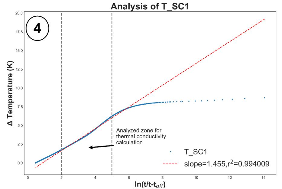
Figure 34 – OTRT analysis of the numerical simulations. Example from Scenario 1. Figure 3 is cut at ca. 70 h.
