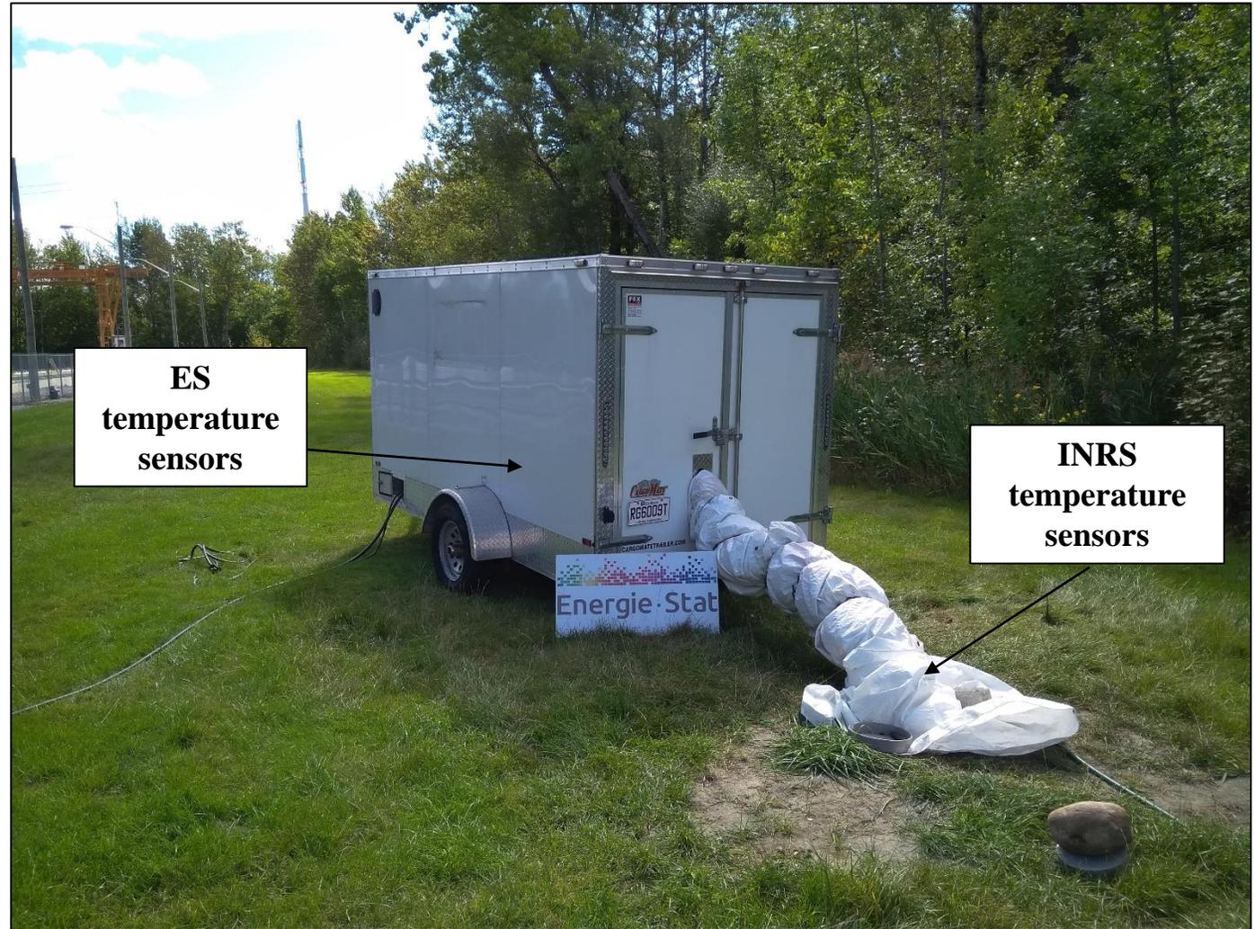
**Figure 13 – Picture of the instrumentation of the partner Energie-Stat.**
