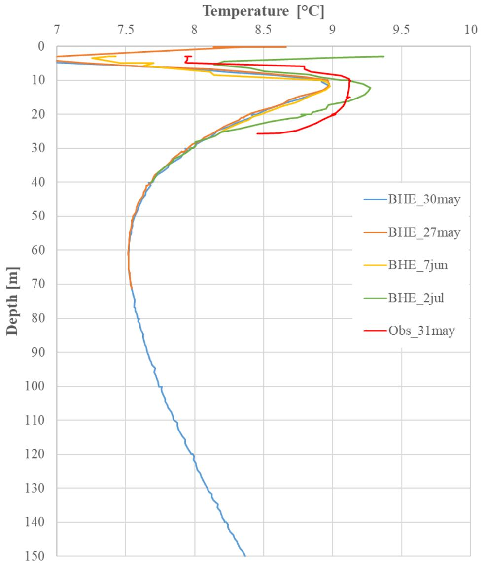
Figure 10 – Temperature profile in the BHE before (27 May) and after the drilling (30 May, 7 June) of the observation well, and after the TRT (2 July). In red the temperature profile made in the observation well few days after the drilling.
