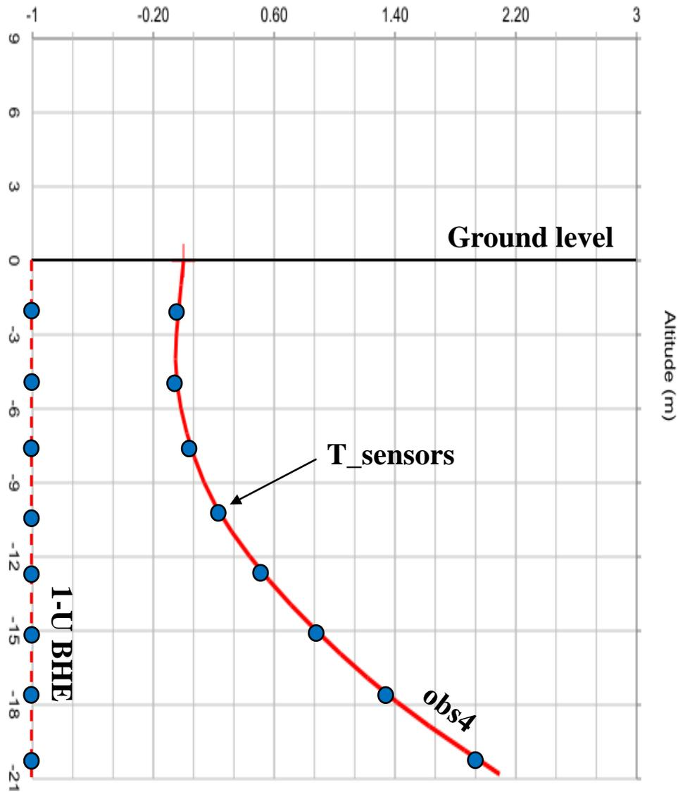
Figure 9 – Location of the BHE, the observation well and the temperature sensors within them down to 21 m.
