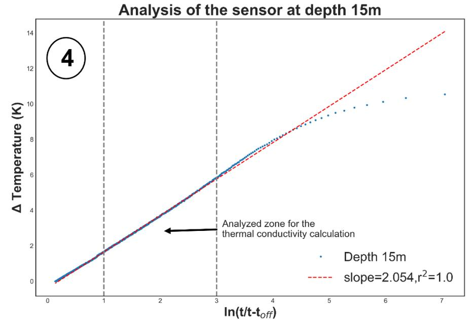
**Figure 25 – OTRT analysis of the test in the open well obs2. Example from sensor placed at a depth of 15 m. Figure 3 is cut at ca. 50 h.**
