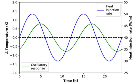
**Figure 1 – Comparison between conventional and oscillatory TRT (modified from Oberdorfer, 2014)**
