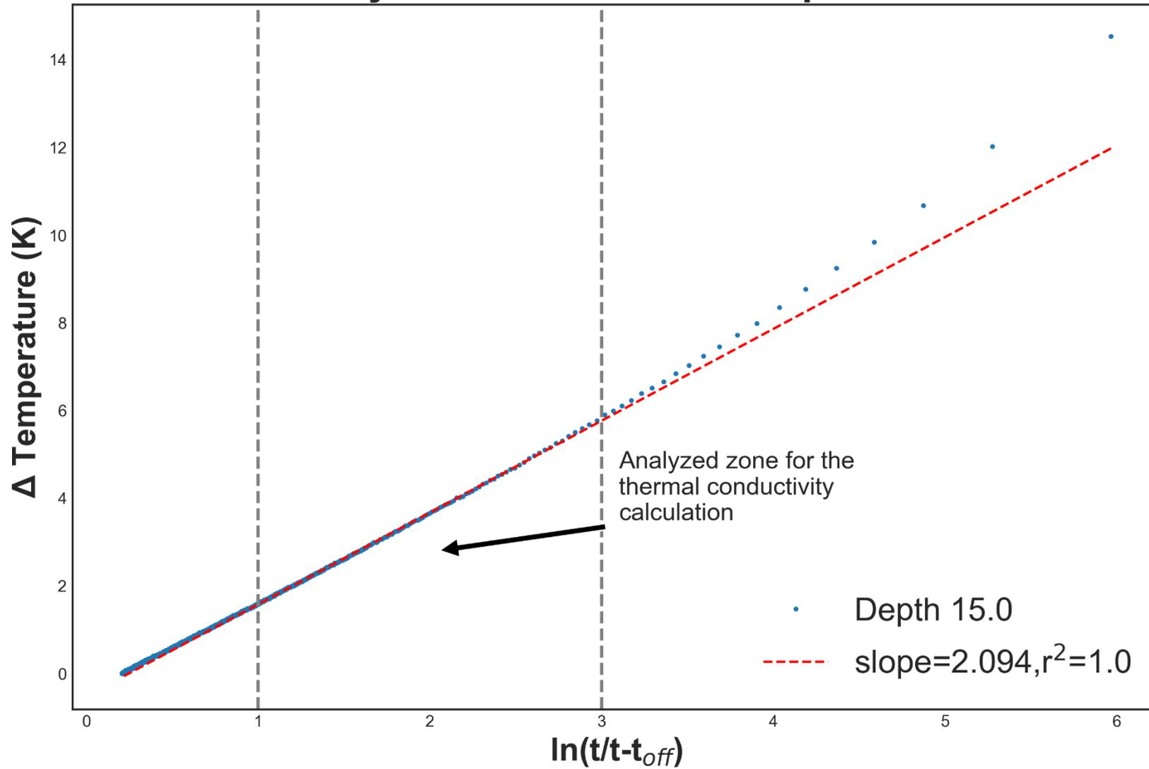
**Figure 20 – Recovery period analysis for thermal conductivity estimation.**
