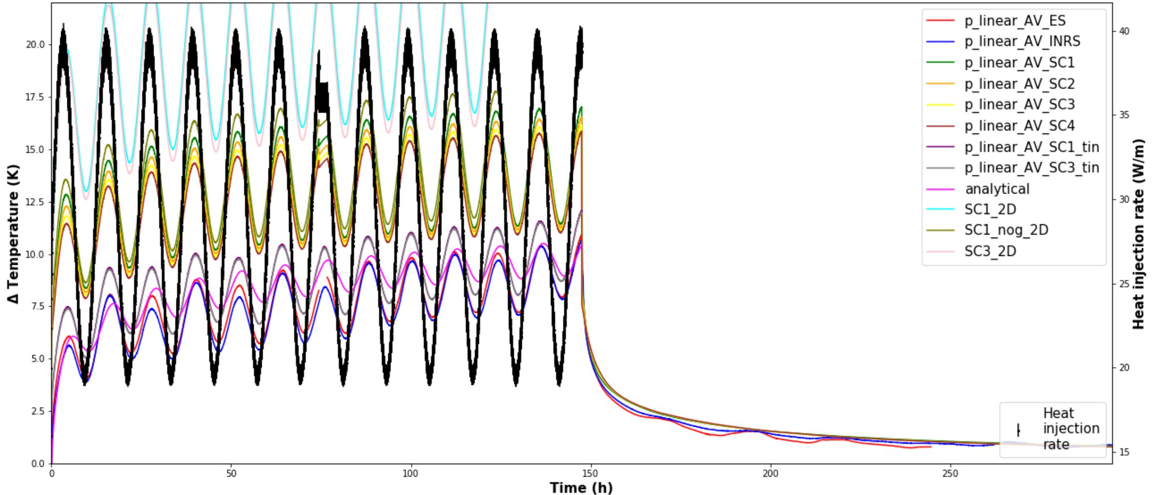
Figure 32 – OTRT numerical simulations compared to experimental water circulation OTRT.
