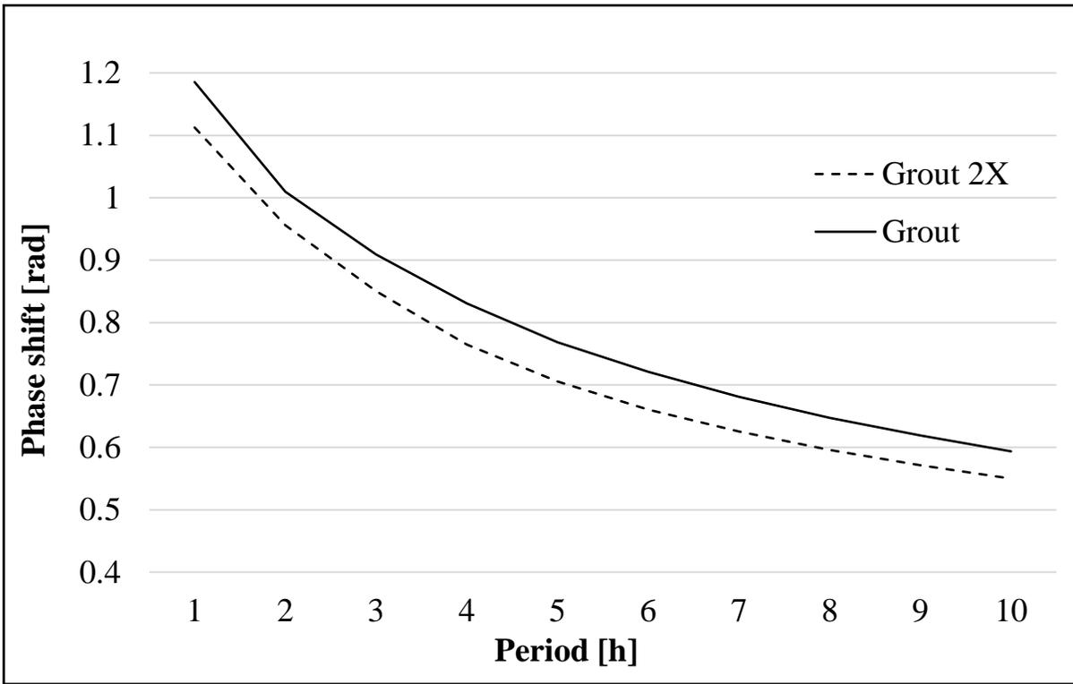
**Figure 7 – Comparison between the phase lag of the thermal response when doubling the heat capacity of the BHE grout (upper-left graph) and the subsurface (lower-right graph)**
