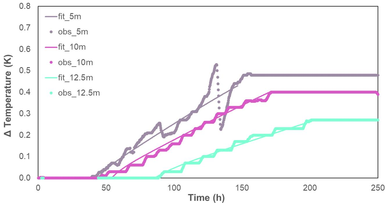
**Figure 22 – Thermal response analysis fit in the observation well obs4.**
