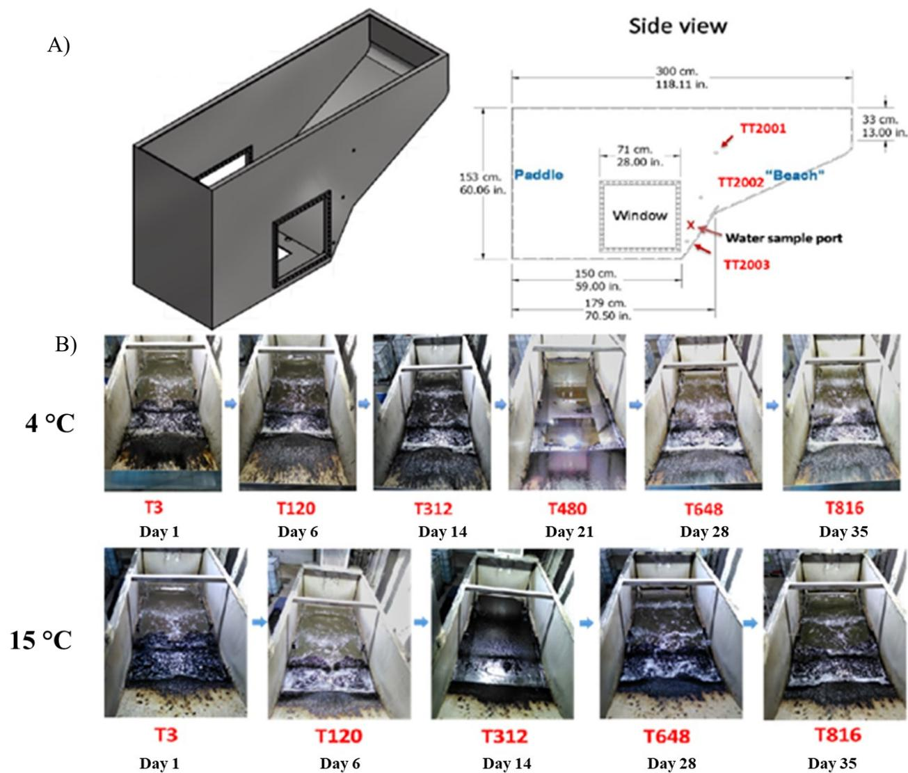
**Figure S4.1** (A) Schematics of the spill tank (B) Time evolution of oil appearance on the water surface.
