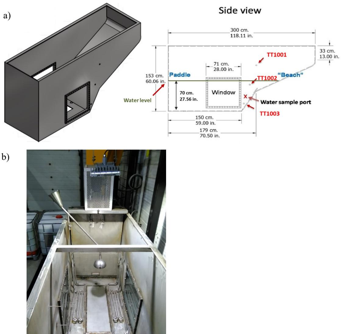
**Figure S3.1.** Spill test tank schematic (a); and, picture including pouring device attached to tank wall on left-side (b).
