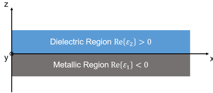
Figure 2.2 Sketch of a 2D plane interface between dielectric and metallic regions.
