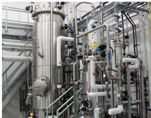
150- and 2000-litre capacity hydrolyzers
