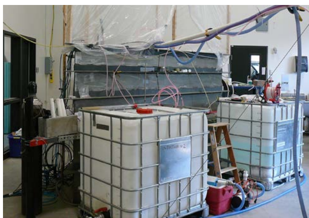
Multiphase extraction and soil washing test
