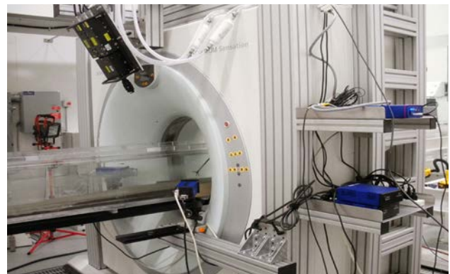
SOMATOM Sensation CT scanner (with mini-flume in bottom image)
