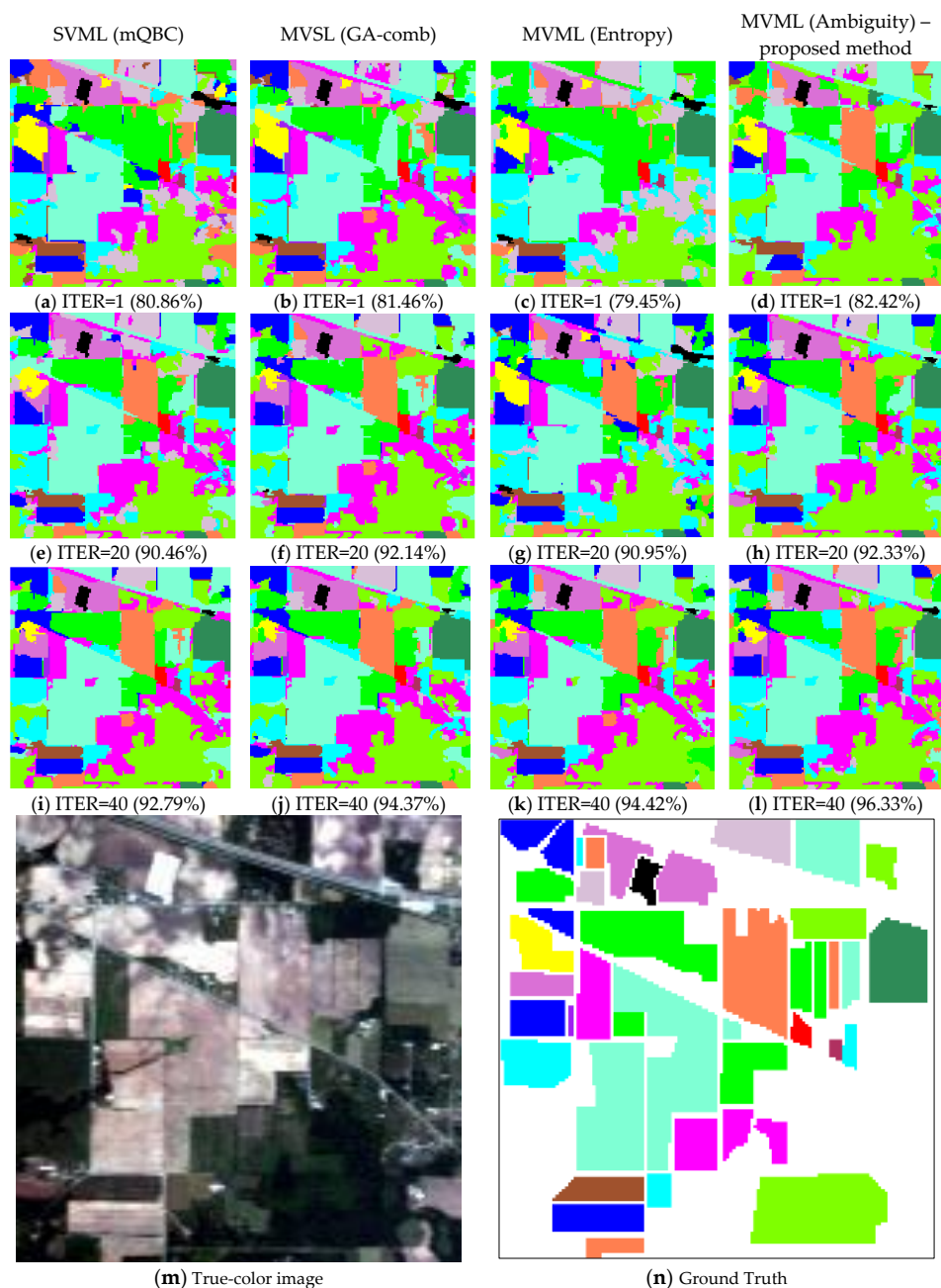
Figure 7. Classification maps of AVIRIS Indian Pines image. Each column represents the different AL method, and each row shows the different iteration of the algorithm. The overall accuracies in percent are reported below the maps.
