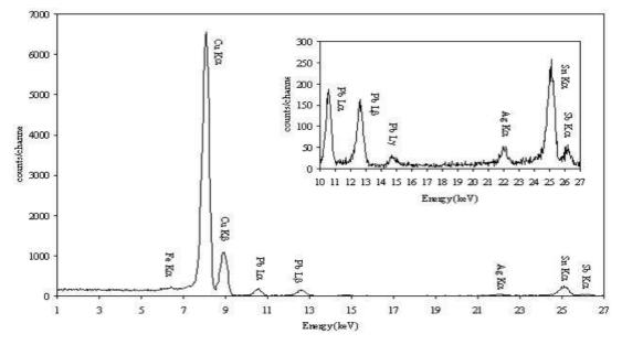
Figure 6 - XRF spectrum of a bronze statue
