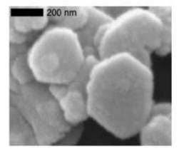
Figure 1 - SEM image of Ca(OH)<sub>2</sub> nanoparticles
