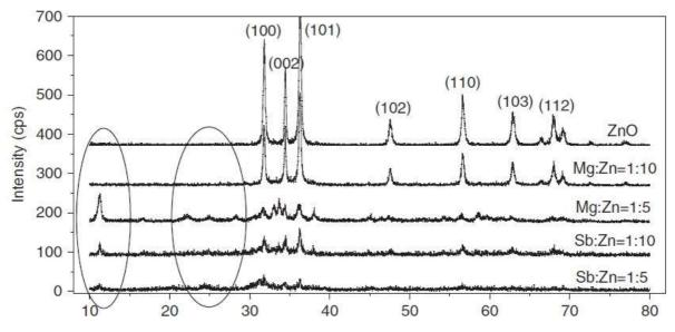
Figure 22 - XRD patterns of a ZnO nanoparticle doped with SB3+ or Mg2+ under heavy doping
