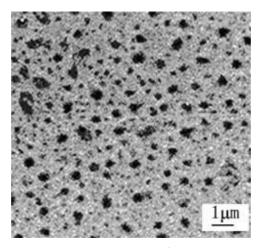
Figure 13 - SEM image of  $Fe^{3+}$  doped  $TiO_2$  film
