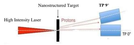
Figure 13 - Experimental setup used for nanostructured target tests
