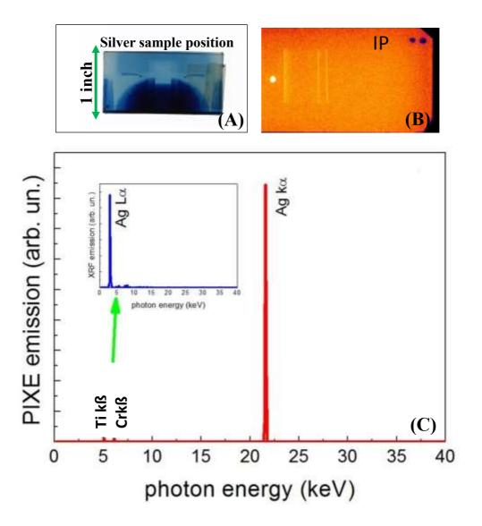
Figure 8 - A) Silver sample mounted in front of the RCF (shown below) indicating the footprint of the laser-generated proton beam; (B) Image Plate (IP) positioned behind the X-ray spectrometer showing the different lines and the zero-order; (C) Convoluted PIXE spectrum obtained by Bragg analysis on the IP shown in (B)
