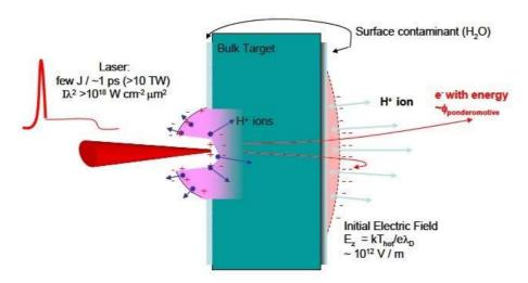
Figure 1 - Basic scheme for the TNSA acceleration process from the rear surface of a solid target. Electrons from the bulk are accelerated and create a strong electric field on the rear surface that ionizes water contaminants and accelerates them orthogonally from the back side of the target. Extracted from the PhD thesis of P.
