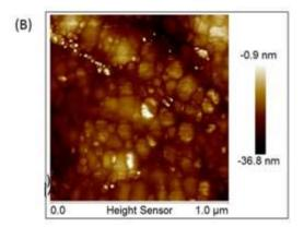
Figure 11 - (A) SEM image of Au NPs deposed on a Silicon substrate and EDX analysis on a NP; (B) AFM Image of a Nanostructured Film on aluminum (Au NP/Al)
