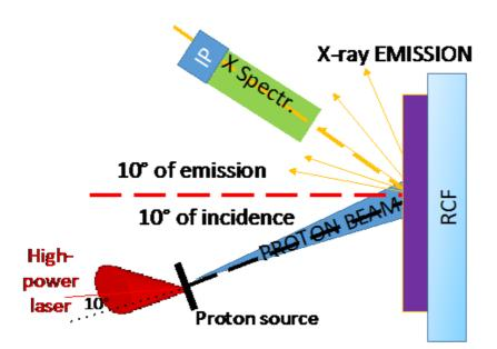
Figure 2 - Experimental Setup used for the one-shot PIXE
