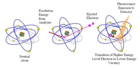
Figure 5 - Sketch of X-ray Fluorescence spectroscopy
