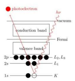
Figure 4 - Sketch of electron photoemission
