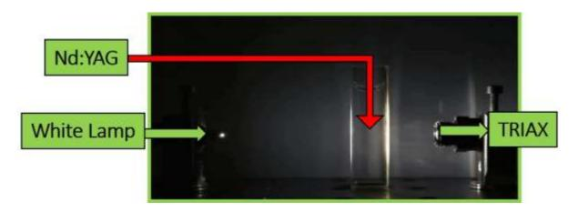
Figure 10 – Sketch of LASiS setup
