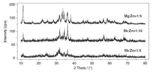
Figure 23 - XRD patterns of a ZnO nanoparticle doped with Sb31or Mg21under heavy doping
