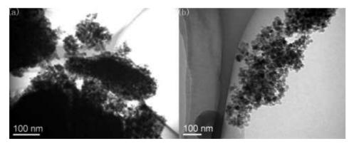
Figure 20 - TEM images of TiO<sub>2</sub>(a) and B/TiO<sub>2</sub>(b)
