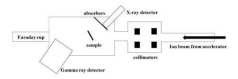
Figure 12 - Typical experiment arrangement for routine PIXE, with detectors for x-rays and  $\gamma$ -rays
