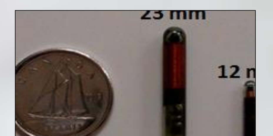
Figure 4 HDX Passive Integrated Transponder used to mark the fish
