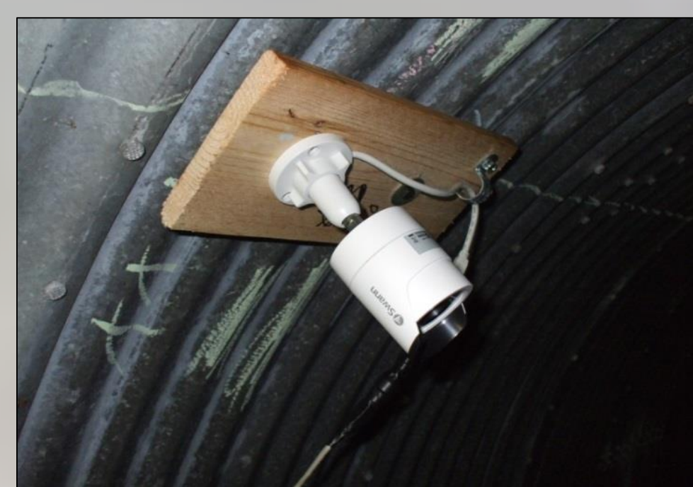
Figure 1: One of the 12 IR video cameras installed on the ceiling of the culvert. Infrared illumination allowed day and night recordings.
