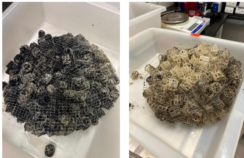
Figure 15) top zone of biocarriers after 4 months of experiment for each reactor (RFK – black vs. HF – white)
