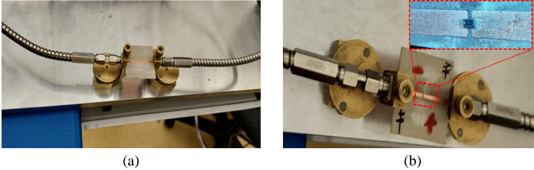
FIGURE 4.14 : (a) microstrip line with gap, (b) micro stripline with diode installed.
