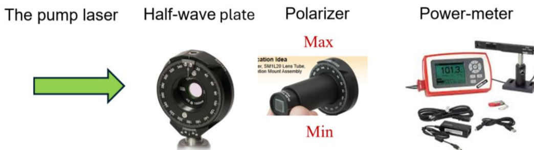
Figure A.13. Schematic diagram illustrating the experimental setup used to evaluate the linearity of the pump laser [145].
