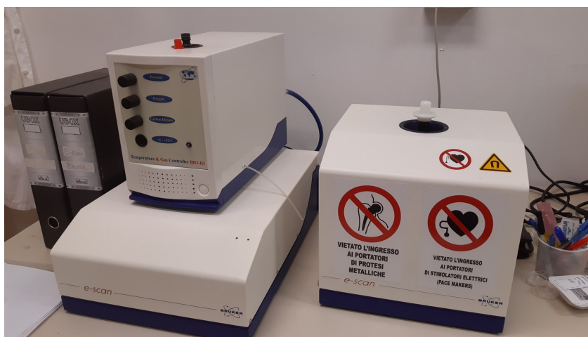
Figure 4.2. Bruker e-scan EPR spectrometer.
