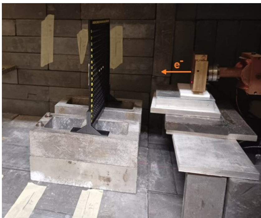
Figure 4.7. Electron irradiation setup of alanine pellets at the REX facility.
