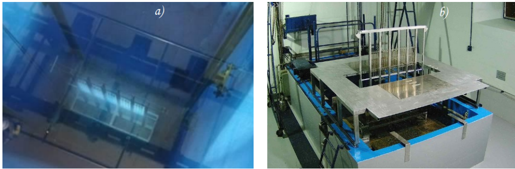
Figure 3.9. a) Calliope source rack in the pool and b) source rack within the irradiation cell (picture acquired by remote camera).
