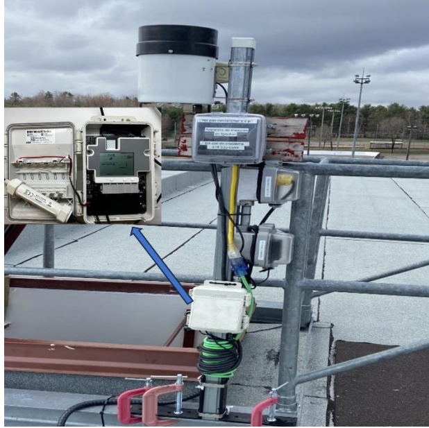
Figure 3-6 ONSET S-RGB-M002 heating tipping bucket rain gauge and the HOBO micro station data logger installed on the roof of the Le Tournesol library
