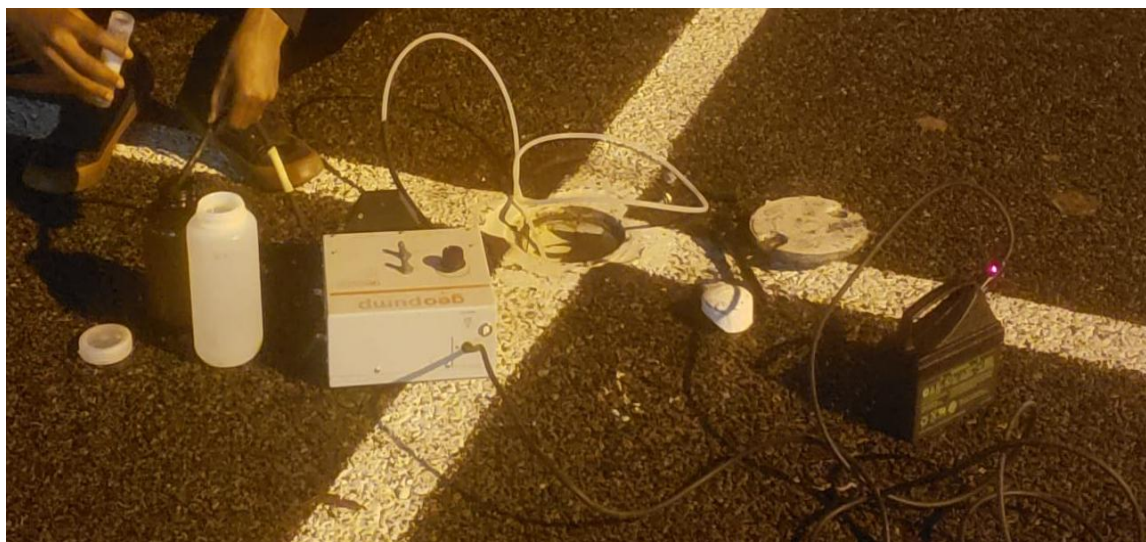
Figure 3-15 Sampling from the observation well (piezometer PZ-2) using a Geopump peristaltic pump from Geotech Environmental Equipment Inc
