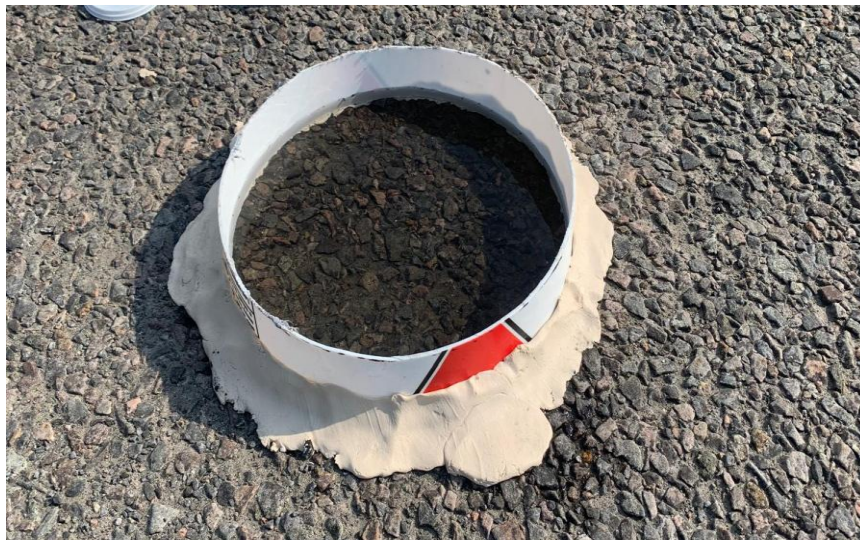
Figure 3-5 Measurement of infiltration rate of the porous asphalt according to ASTM C1781/C1781M-17a method
