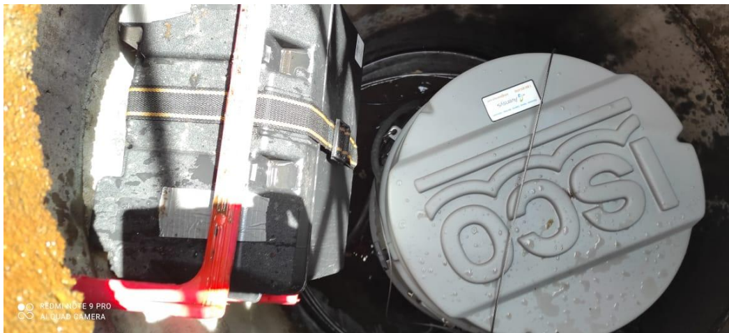
Figure 3-12 Autosampler installed in catch basin PU-2
