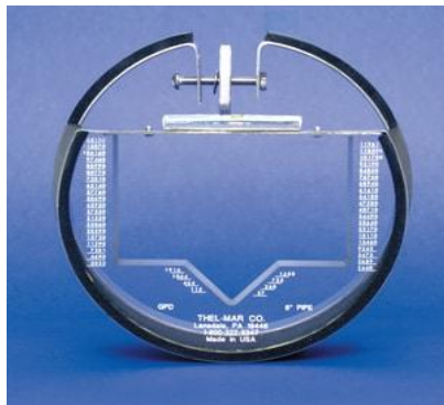
Figure 3-9 Thel-Mar weir (left) and HOBO MX2001 pressure probes (right) for flow monitoring
