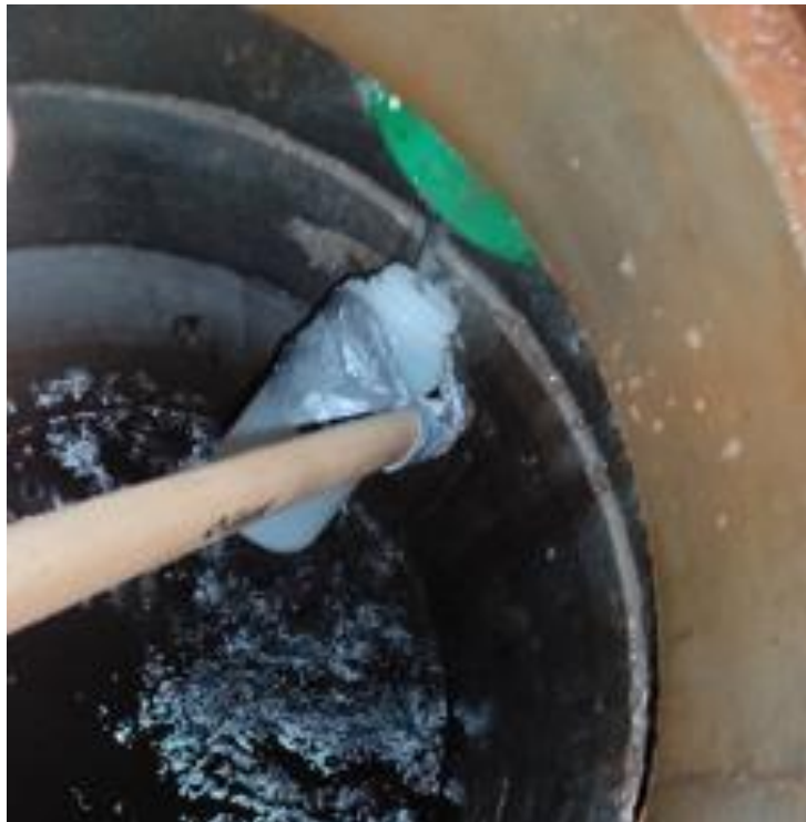
Figure 3-14 Manual sampling of water from the underdrain
