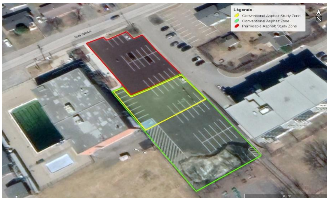
Figure 3-1 Parking lot specification: porous asphalt (red), conventional asphalt (yellow), and conventional asphalt not considered in this study (green)
