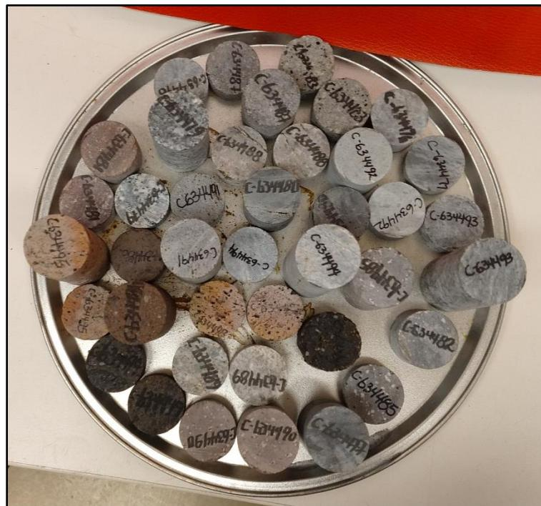
Each sample was measured with an electronic calliper and scale to determine their length, diameter, volume, and weight. Then, the grain volume measurement system of Coretest's AP-608 Permeameter-Porosimeter was used to calculate their density and porosity at room pressure (**Table 1**).
