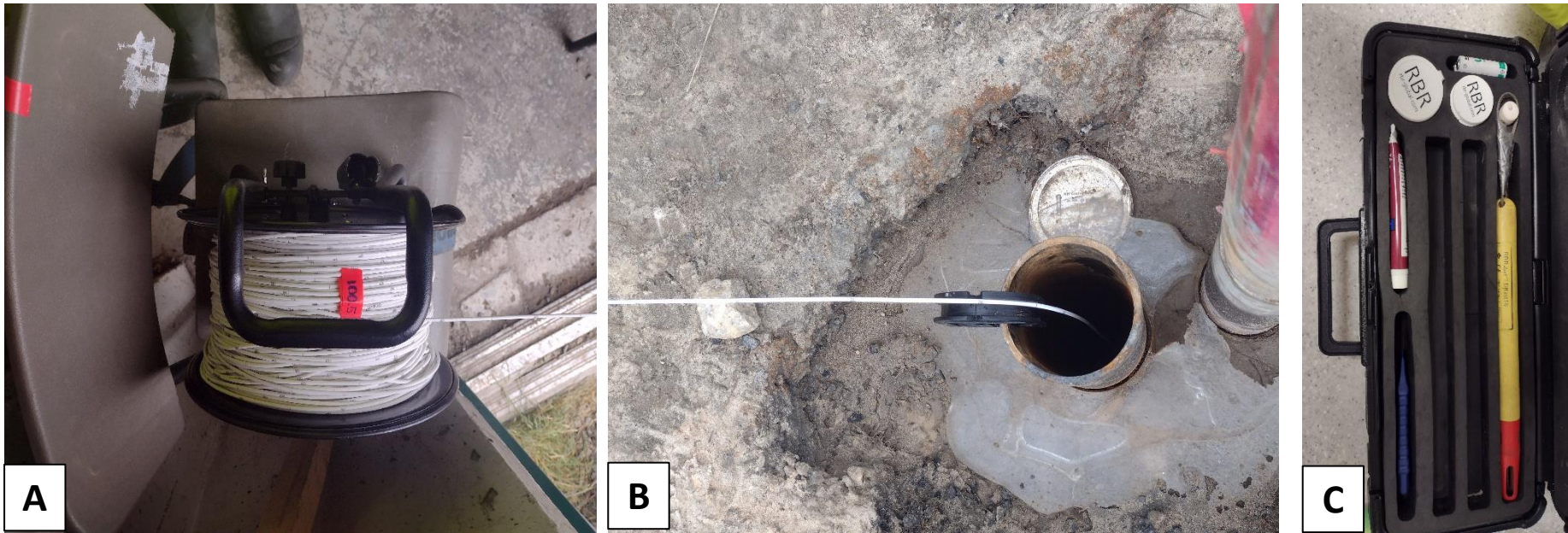
Figure 10 –Temperature depth profile measurement. A-B- cable placed inside well ; C-RBR duet probe.
