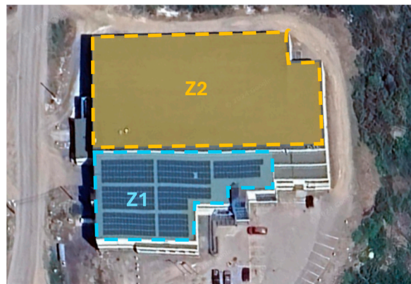
Figure 8. Aerial photograph of Kuujuaq Forum. Z1 is dedicated zone for current solar panels system and Z2 is remaining available roof surface.
