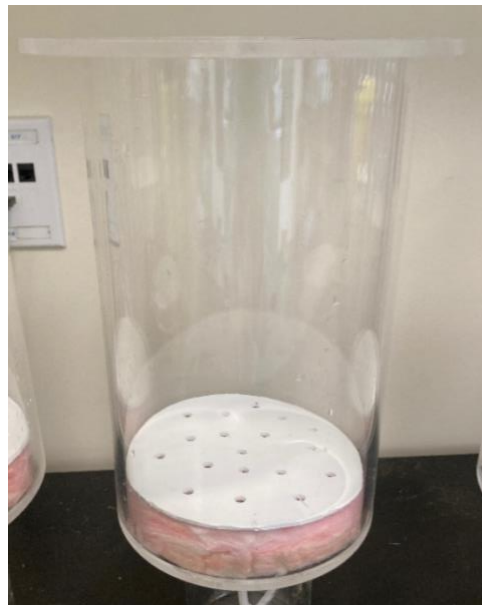
Figure 8 Empty column with fibreglass and plexiglass filter
