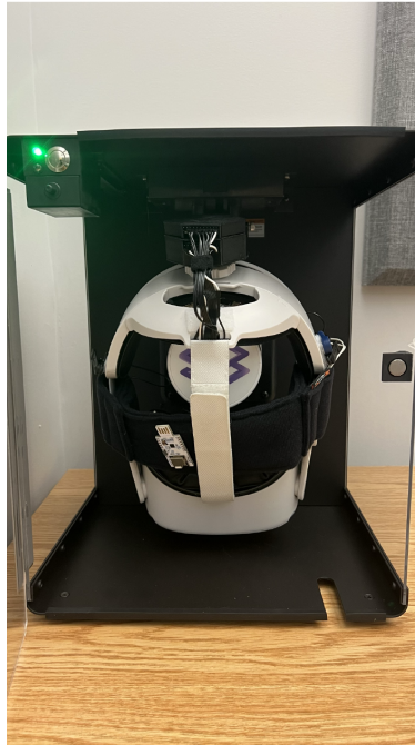
Figure 5.5: An illustration showing the HMD system positioned inside a Cleanbox UV-C chamber.
