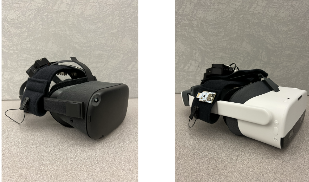
Figure 3.9: Instrumented Quest VR headset (left) and Pico Neo 3 (right), showcasing the integration of multimodal physiological sensors.
