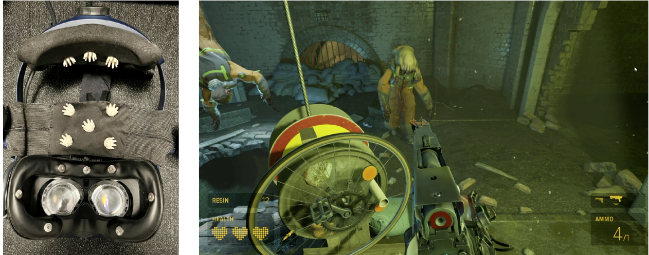
Figure 6.1: On the left: 16 ExG biosensor-instrumented VR headset used to collect data. On the right: participant’s view of a scene played in the VR game Half-Life: Alyx.
