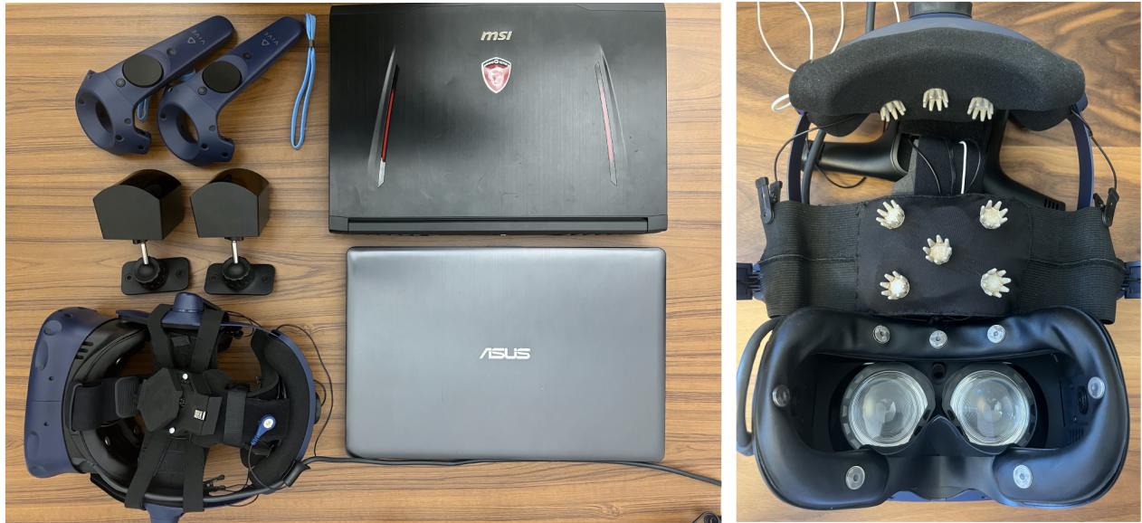
Figure 5.3: On the left: entire equipment drop off at participant’s home including 2 laptops, base stations, controllers and the instrumented HMD; on the right: 16 ExG sensor-equipped VR headset.
