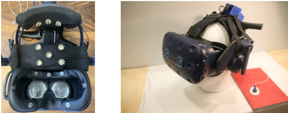
Figure 3.6: Instrumented HTC Vive Pro Eye VR headset featuring CGX dry rigid EEG electrodes, flat EOG electrodes, and a single-channel disposable ECG electrode
