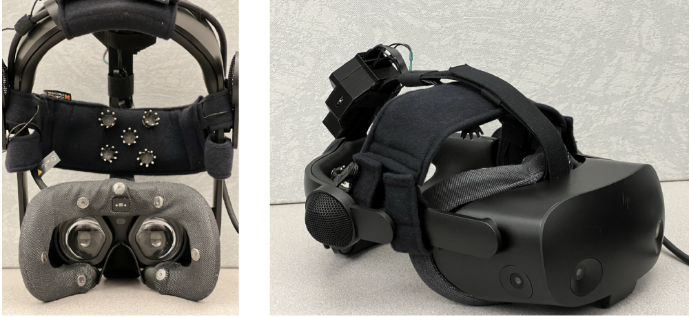
Figure 3.7: Instrumented HP Reverb G2 VR headset featuring dry EEG electrodes from Cognionics and flat EOG electrodes
