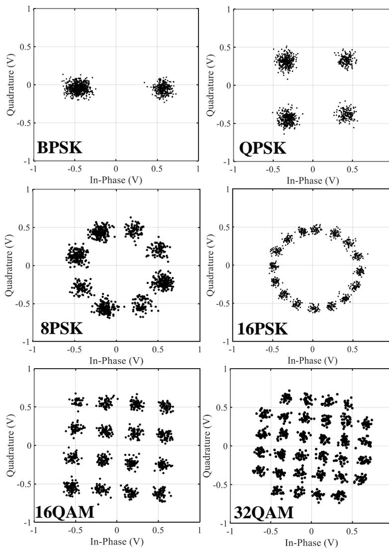
**Figure 5.29** Measurement constellation results of the demodulated PSK/QAM signals for different symbols.
