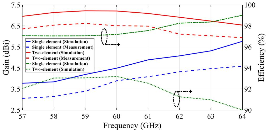
**Figure 2.4** The gain and efficiency of the single-element and two-element DRAs.
