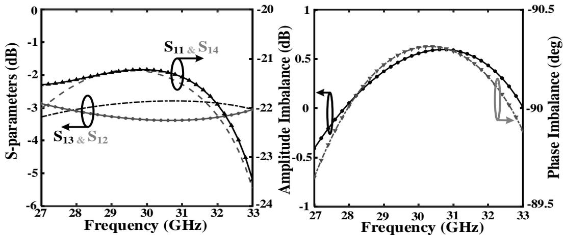
Figure 5.4 (a) Frequency response of the s-parameters belongs to the proposed hybrid coupler and (b) the amplitude and phase imbalance response of the proposed hybrid coupler.
