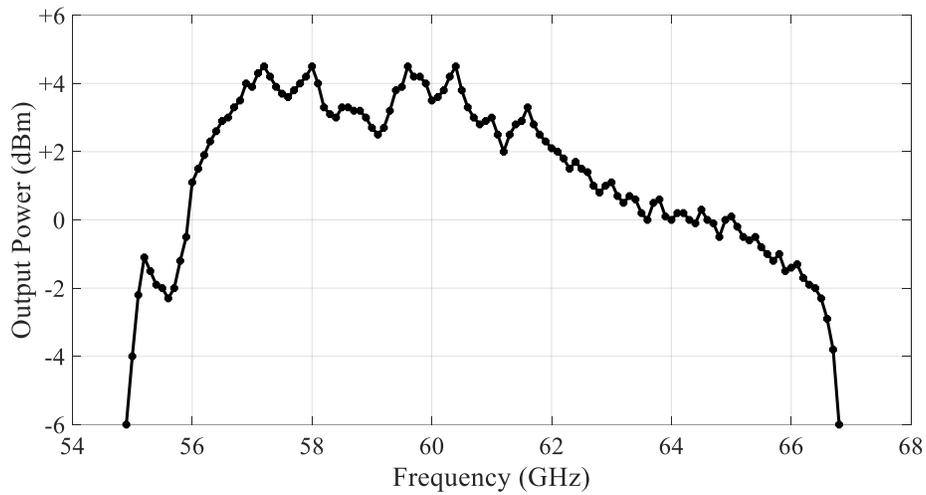
**Figure 2.9** The measured output signal of the fabricated LO chain module.
