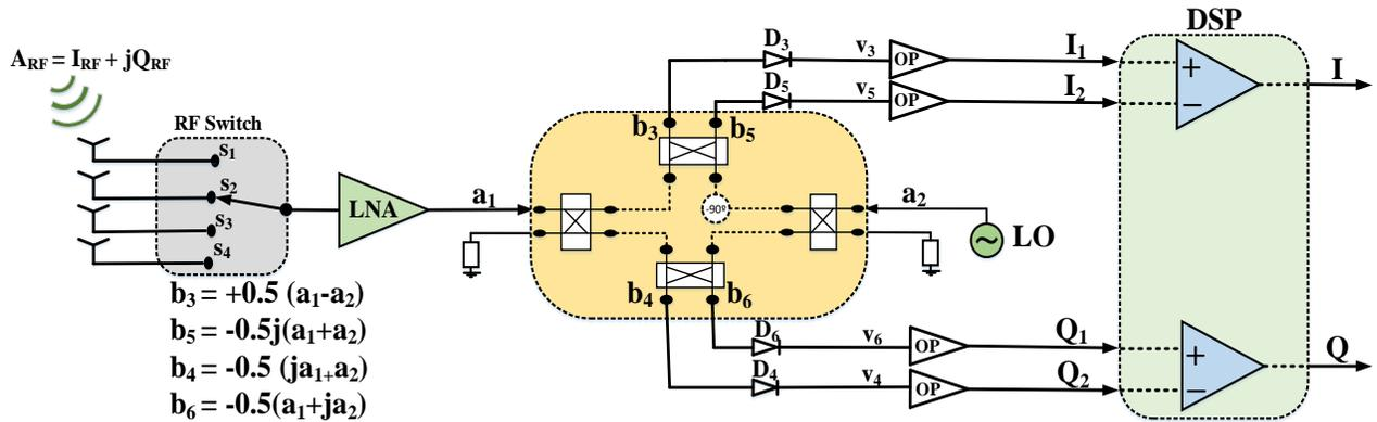
Figure 5.13 Block diagram of the analog front-end for down-conversion.
