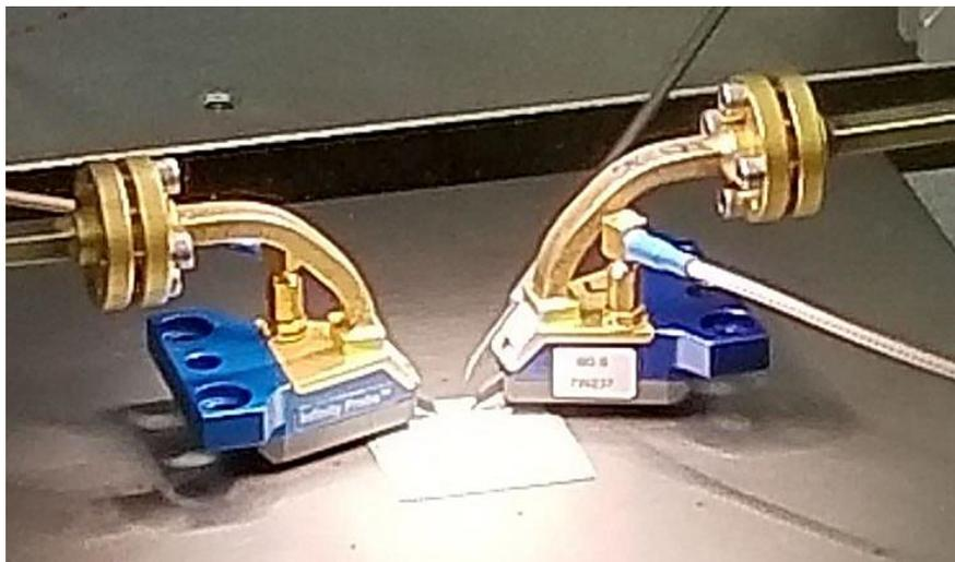
Figure 2.10 A photo of a circuit under test using GSG coplanar probes.
