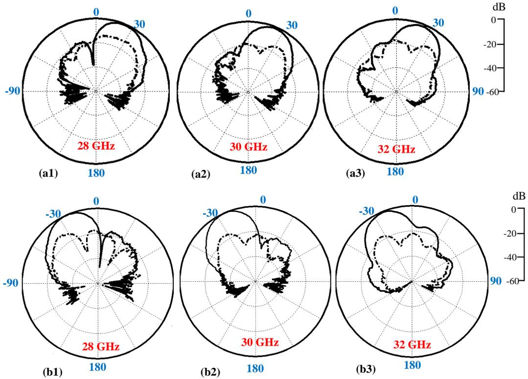
Figure 5.12 Measured radiation patterns of the proposed BSAN at frequencies of 28, 30, and 32 GHz when the BSAN is excited by (a) port 2 (up) and (b) port 1 (down). Note that solid and dashed lines represent the co- and cross-polarized results, respectively.
