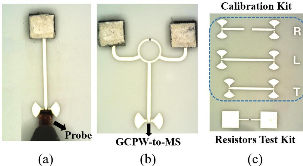
Figure 2.2 The photo of fabricated (a) single-element DRA, (b) two-element DRA array, (c) TRL calibration and resistor test kit.
