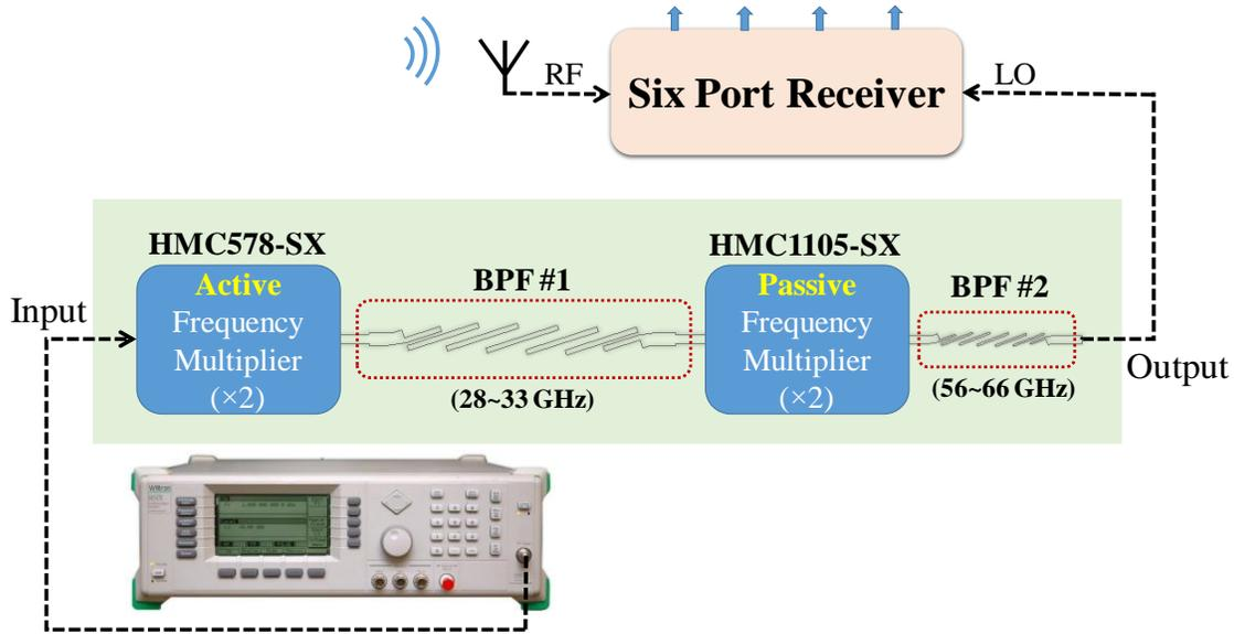
Figure 2.6 Block diagram of the proposed LO chain module used for six-port receivers.
