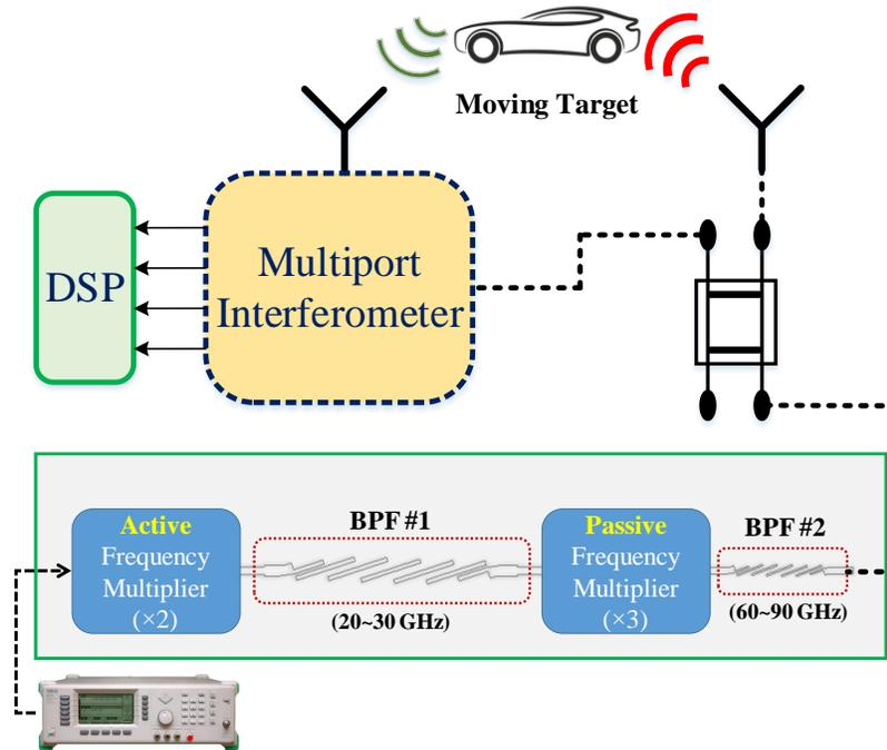
**Figure 4.13** Block diagram of a sample of the homodyne radar system and the role of BPFs in their applications.
