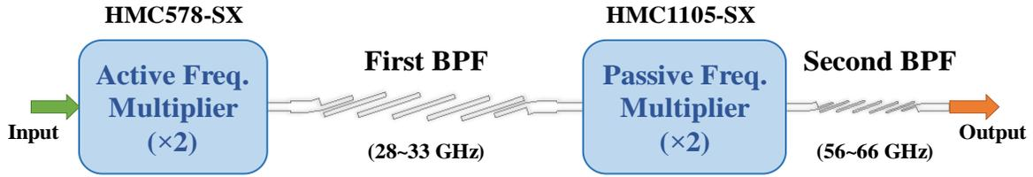
Figure 3.6 Block diagram of the designed frequency multiplier module.
