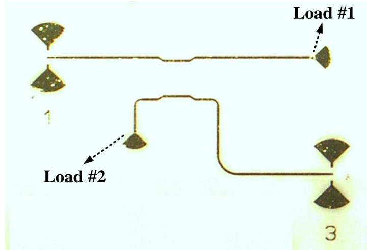
Figure 2.12 A microphotograph sample of the fabricated directional coupler for measuring the coupling ( $S_{13}$ ) value.
