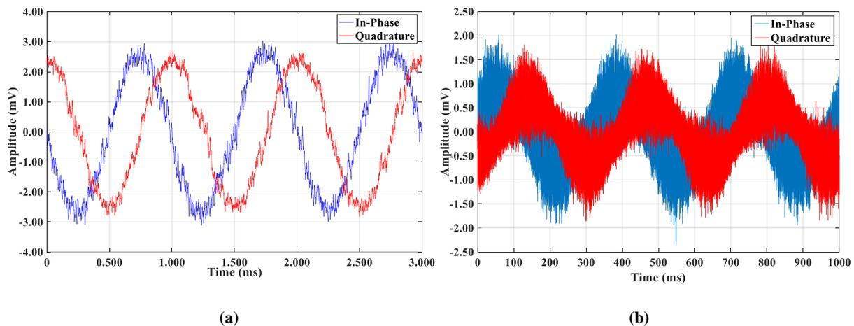
**Figure 4.7** The measured results of I and Q output signals for (a) 1 kHz, and (b) 3 Hz CFO between two input ports of the front-end module.
