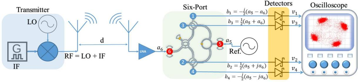
**Figure 4.1** The block diagram of the proposed front-end in a communication link.
