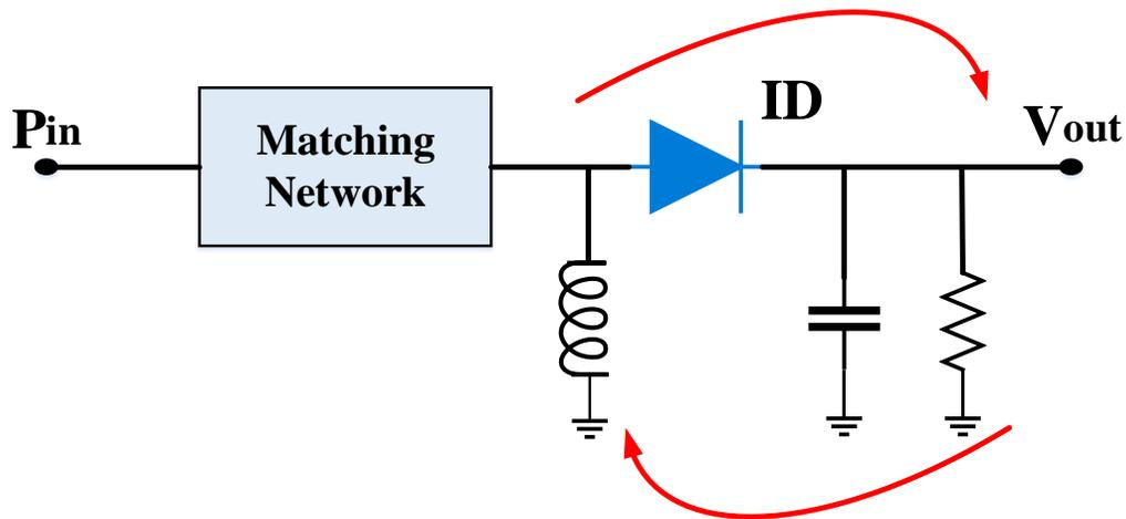
Figure 1.7 Diode detector circuit schematic.
