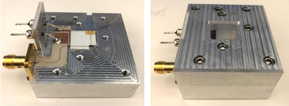
**Figure 2.8** The assembled frequency multiplier module based on MHMIC technology (left), and with aluminum case (right).
