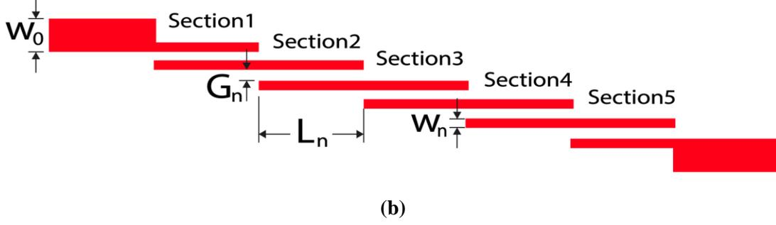
Figure 4.14 (a) The  $n$ -th coupled stage and, (b) the topology of 5<sup>th</sup>-order parallel coupled line BPF.
