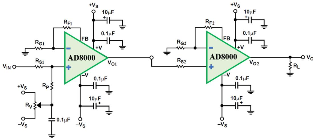
Figure 3.4 Block diagram of the baseband circuit using AD8000 op-amps.
