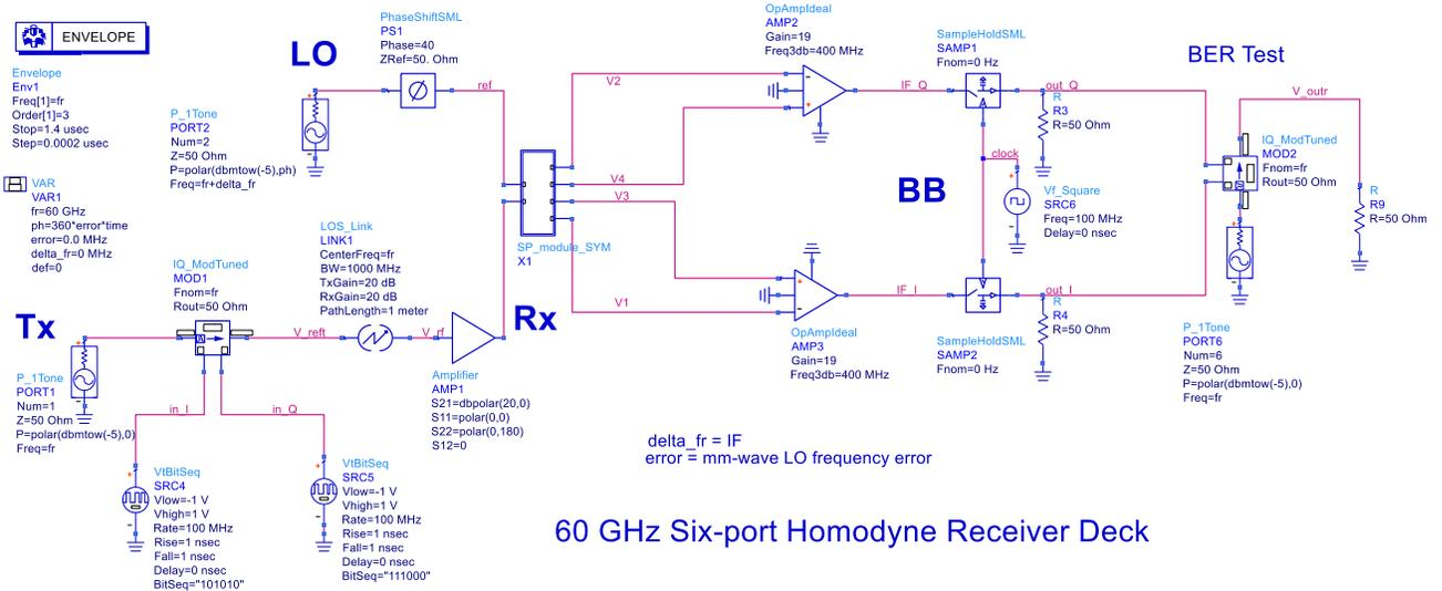
Figure 3.9 The ADS simulation deck of the proposed system (4-QAM pseudo-random modulation at 200 Mb/s).
