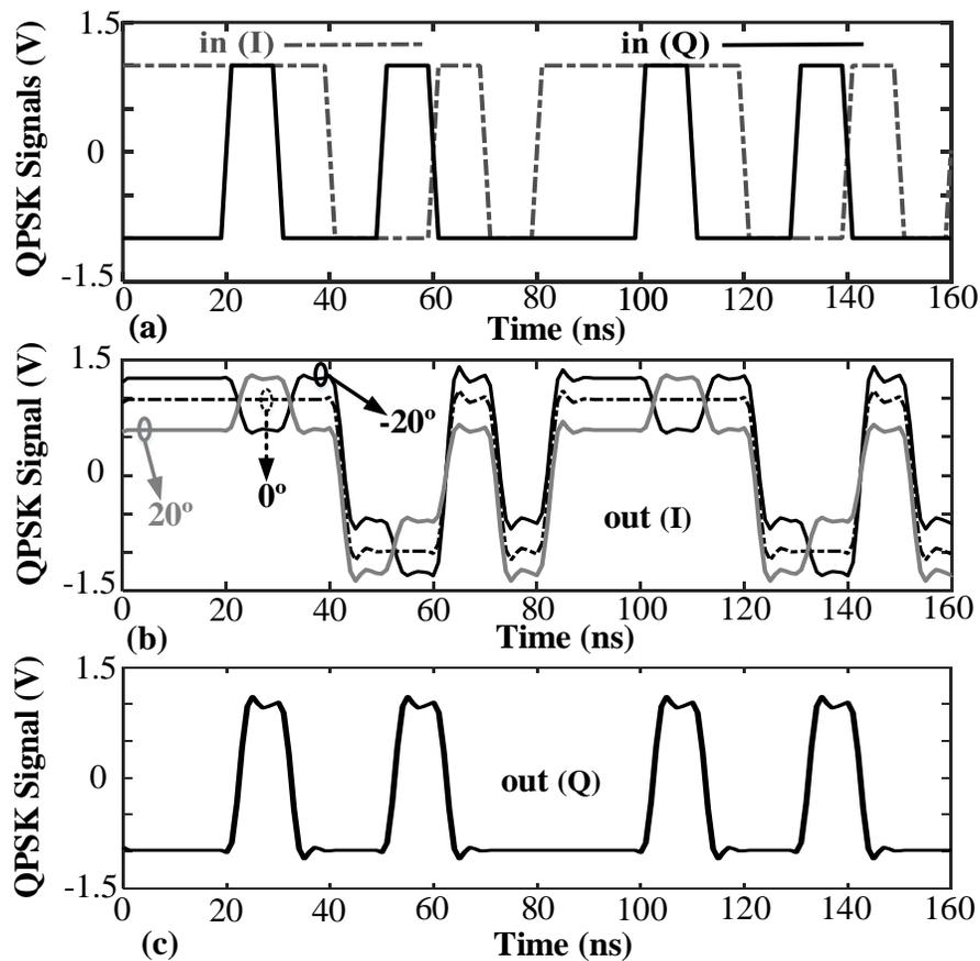
**Figure 5.19** Simulated signals of QPSK versus the time, (a) input I and Q, (b) output I, and (c) output Q. Note that output I is changing with phase variation of phase shifter while output Q remains without change.
