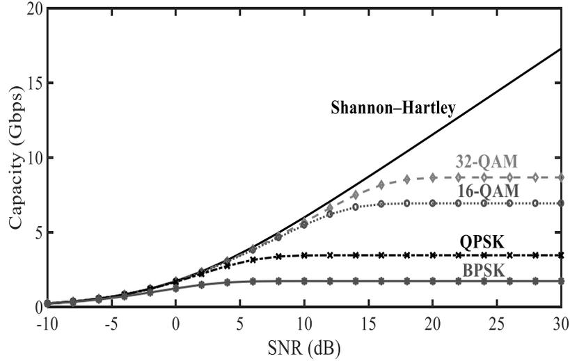
**Figure 5.24** Channel capacity for the proposed developed system associated with the BPSK, QPSK, 16QAM, and 32QAM modulations.
