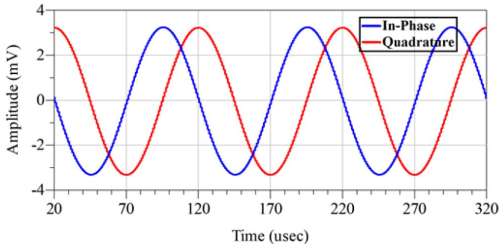
Figure 4.3 The simulation results of quadrature output signals for 10 kHz CFO.
