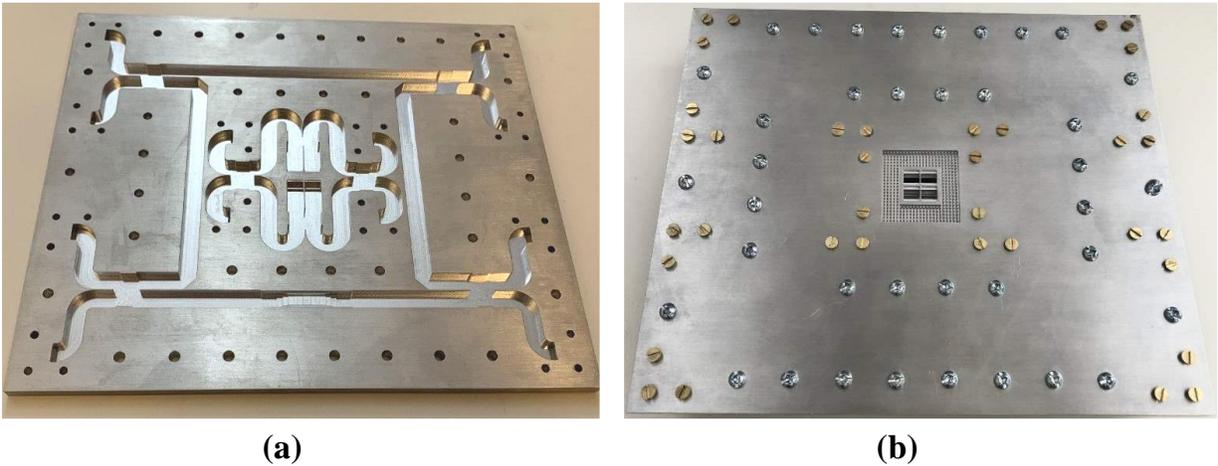
**Figure 5.22** Fabrication photo of the two-layer proposed design (a) the bottom layer including the waveguide feeding network for the BSAN and SPN and (b) the top layer including the radiating antenna elements.
