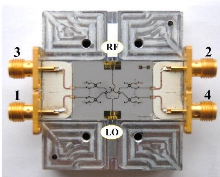
Figure 4.5 The fabricated V-band front-end module based on MHMIC technology.
