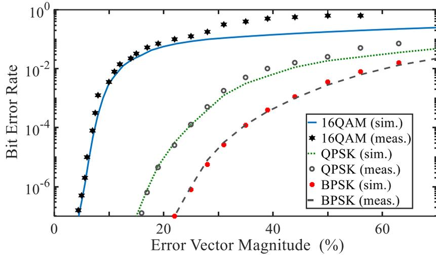
Figure 3.16 Stylized BER versus EVM Performance Curves for the proposed SPI receiver.
