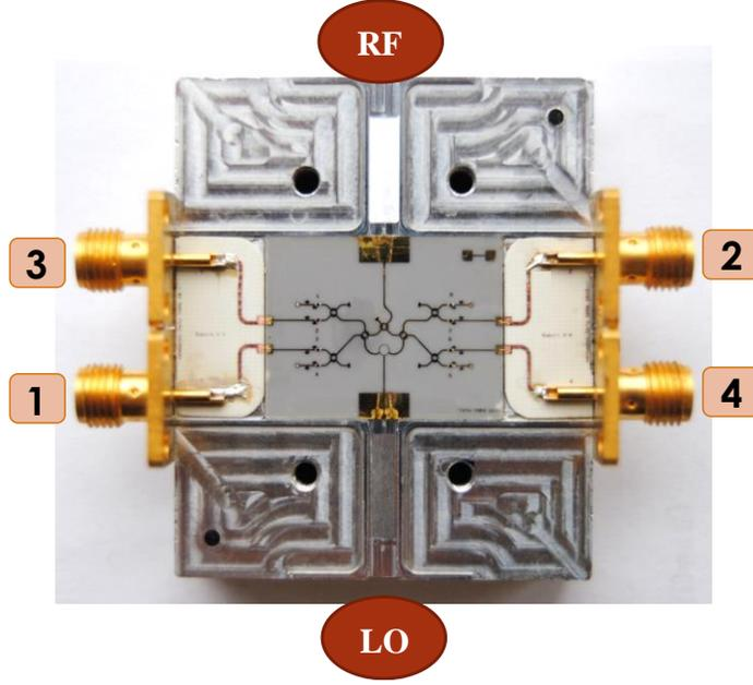
**Figure 3.3** The fabricated V-band front-end module, including SPI and power detectors [58].
