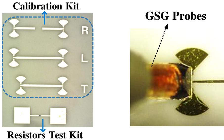
Figure 2.11 A photo of the fabricated TRL calibration kit and the coplanar waveguide to microstrip line transition.
