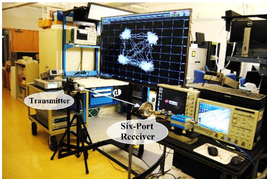
Figure 4.6 A photo of the V-band wireless link experimental setup.
