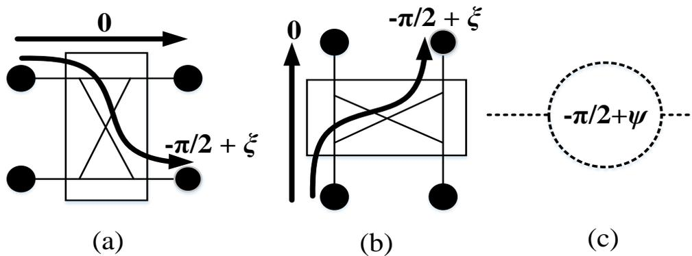
Figure 5.18 Phase errors in the SPN including four  $90^\circ$  hybrid couplers and one  $90^\circ$  phase shifter; (a) phase errors in horizontal couplers terminated to the input ports, (b) phase errors in vertical couplers terminated to output ports, and (c) phase error in a  $90^\circ$  phase shifter (see the SPN topology in Figure 5.14). Note that due to the identical hybrid couplers, the phase error in the two couplers is the same ( $\xi$ ).
