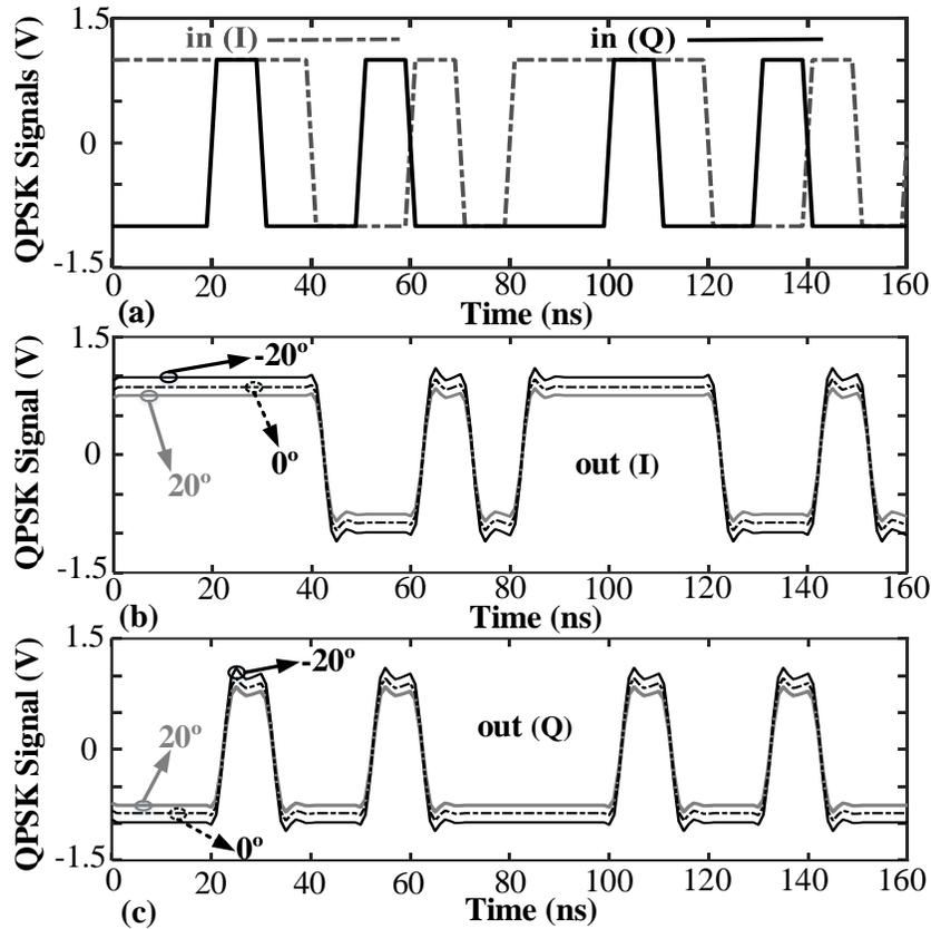
Figure 5.20 Simulated signals of QPSK versus the time, (a) input I and Q, (b) output I, and (c) output Q. Note that both outputs of I and Q are changing with phase variation of hybrid couplers.
