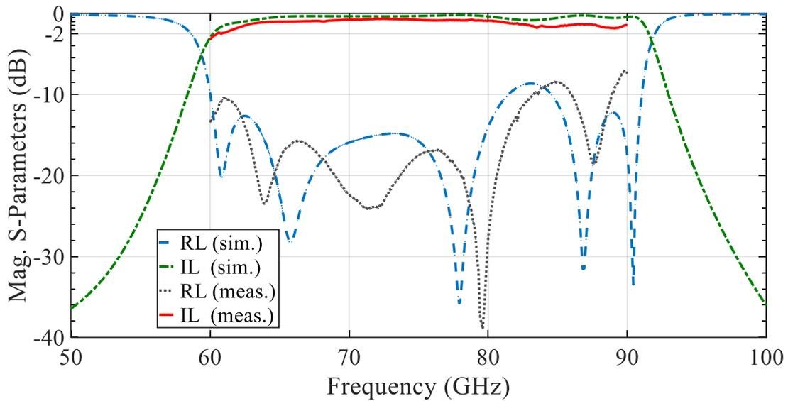
**Figure 4.16** The simulation and experimental results of S-parameters for the bandpass filter (RL: Return Loss, and IL: Insertion Loss).
