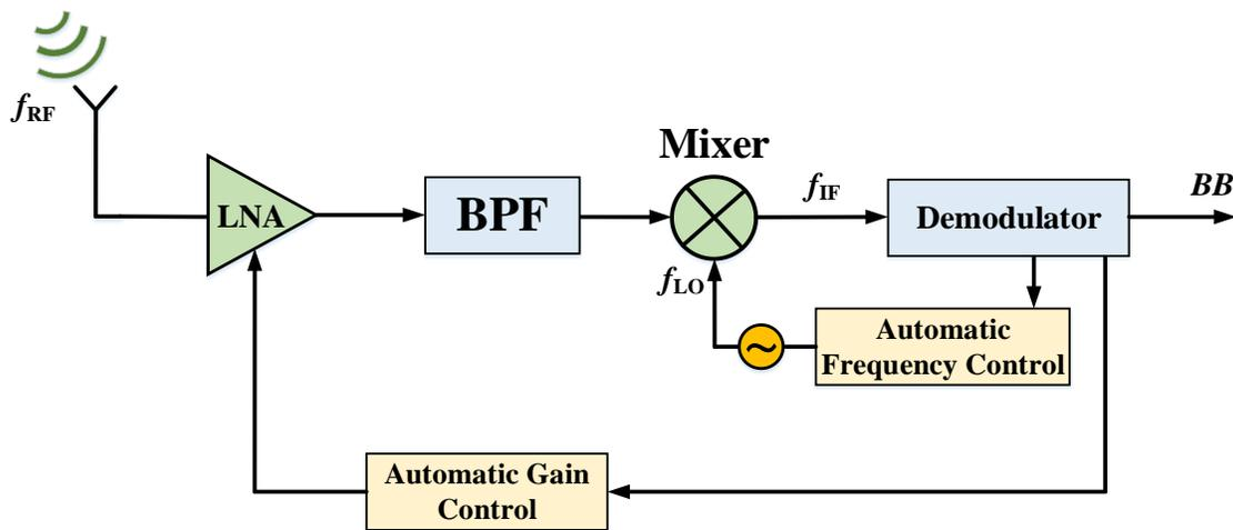
Figure 1.1 Overall structure of a receiver.
