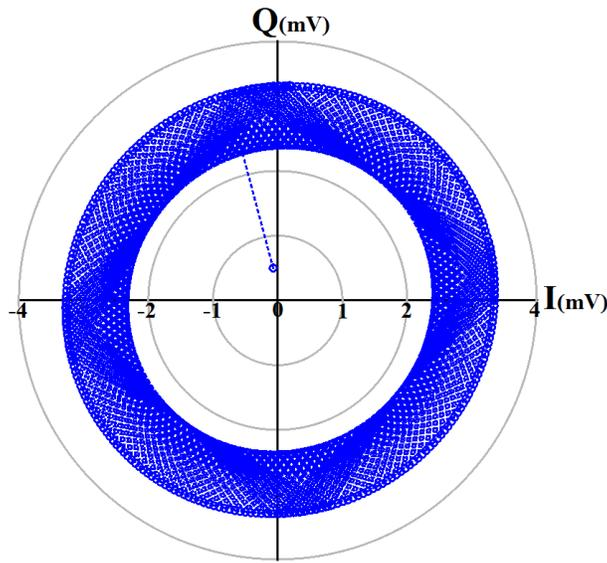
Figure 4.4 The demodulated QPSK constellation for a 10 kHz CFO (simulation).
