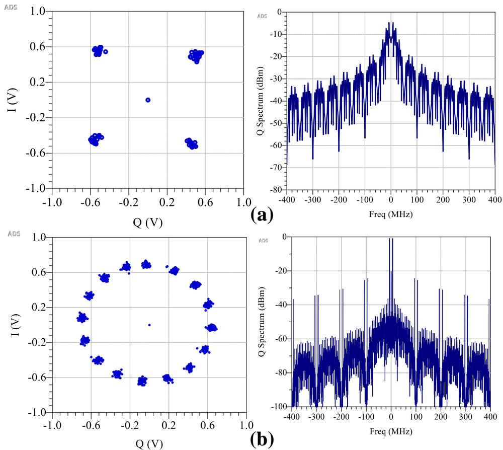
**Figure 3.10** Simulation results of demodulated data for (a) 4QAM, (b) 16PSK signals.
