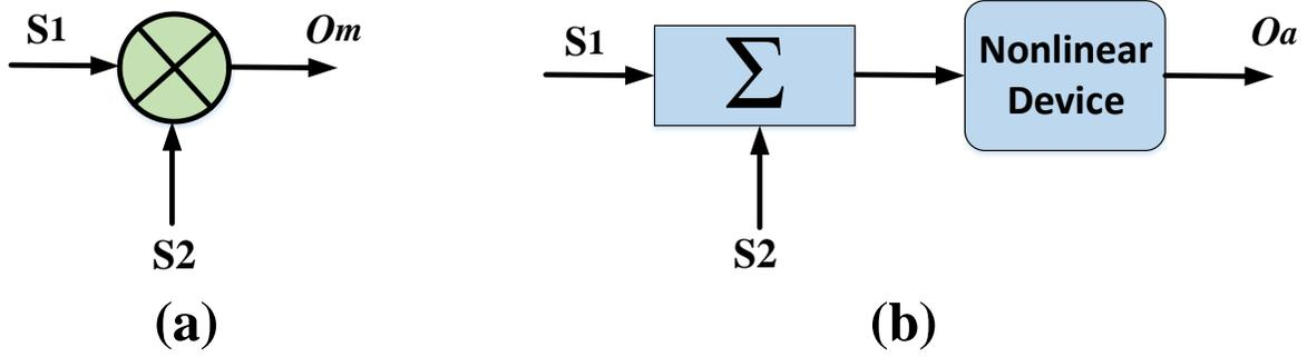
Figure 1.4 Two different mixing processes (a) Multiplicative mixing, and (b) Additive mixing.
