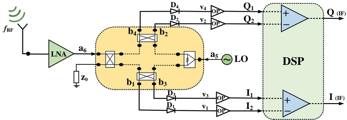
Figure 3.1 The block diagram of the designed front-end based on the six-port interferometer (SPI).
