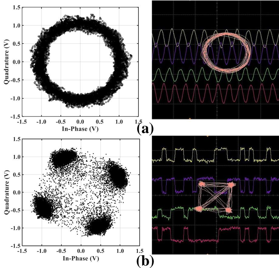
Figure 3.17 A QPSK constellation signal (a) with CFO effect (b) after the compensation for CFO.
