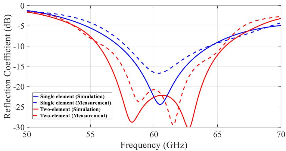
**Figure 2.3** Simulation and measured reflection coefficients of single-element and two-element DRAs.
