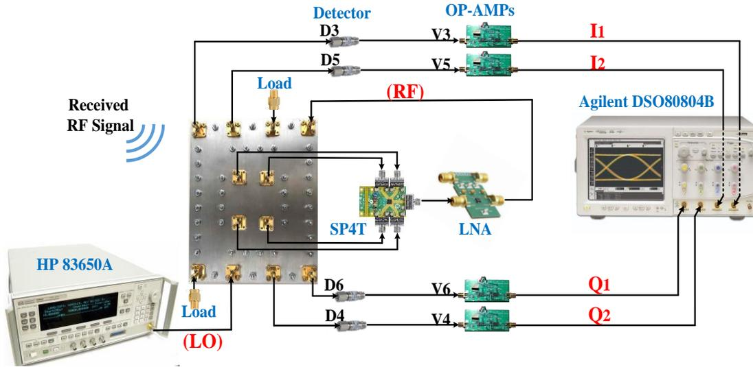
Figure 5.27 Full test setup for the proposed broadband zero-IF receiver.
