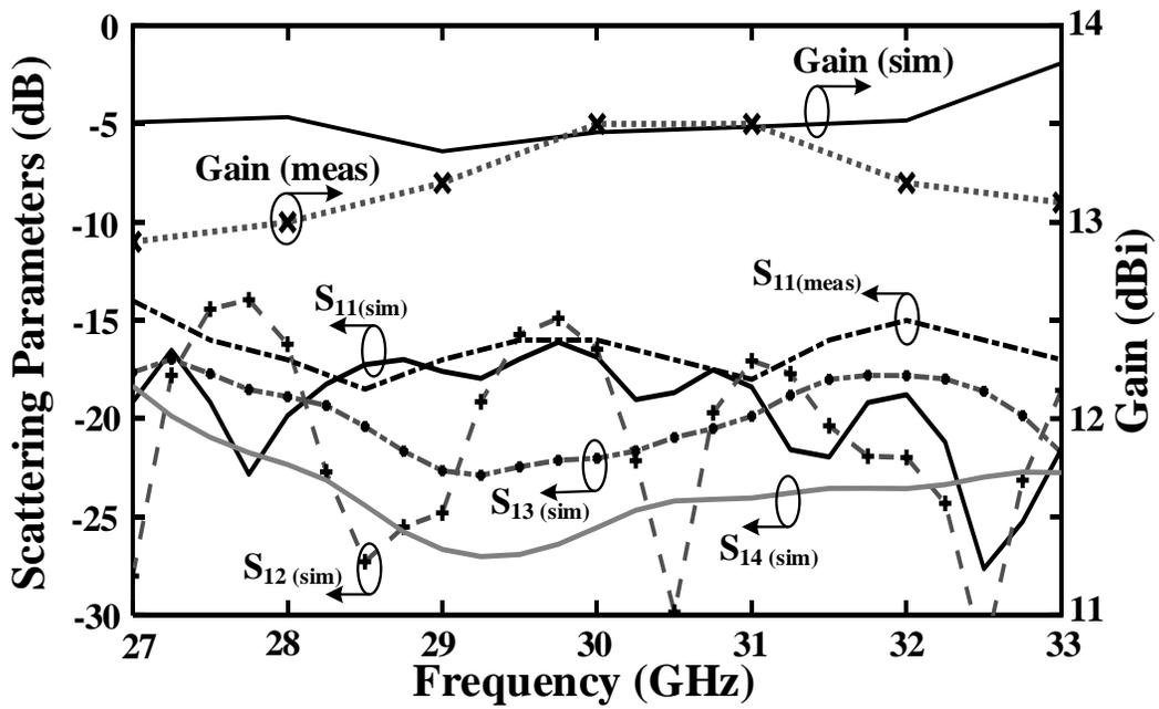
Figure 5.11 Measured and simulated results of the scattering parameters and gain of the proposed BSAN when it is excited by port 1.
