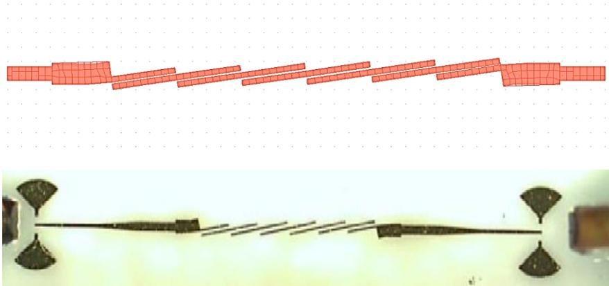
**Figure 4.15** The designed layout of BPF in ADS Momentum (top), and the fabricated BPF including coplanar ports for the measurement (bottom).
