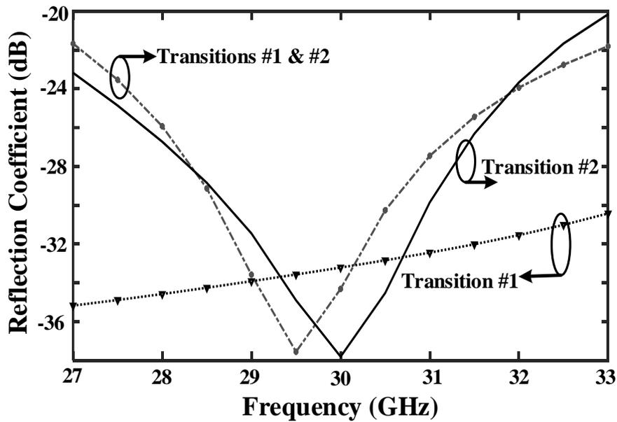
Figure 5.7 The frequency response of the reflection coefficient of the transitions shown in Figure 5.5 (b) and Figure 5.6.
