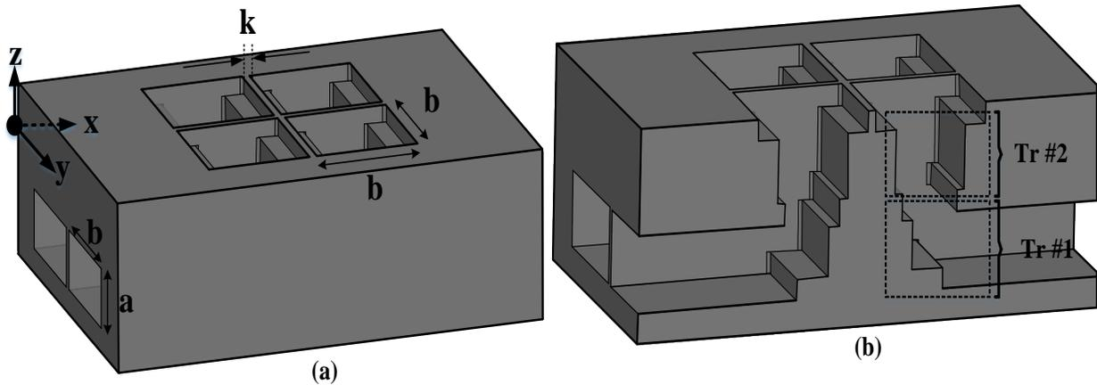
**Figure 5.5** (a) 3-D view of the  $2 \times 2$  open-ended waveguide antennas as radiating part of the proposed BSAN and (b) 3-D view of the  $2 \times 2$  antennas when the side layer is partly removed. ( $a=3.56 \text{ mm}$ ,  $b=7.11 \text{ mm}$ ,  $k=0.5 \text{ mm}$ ).
