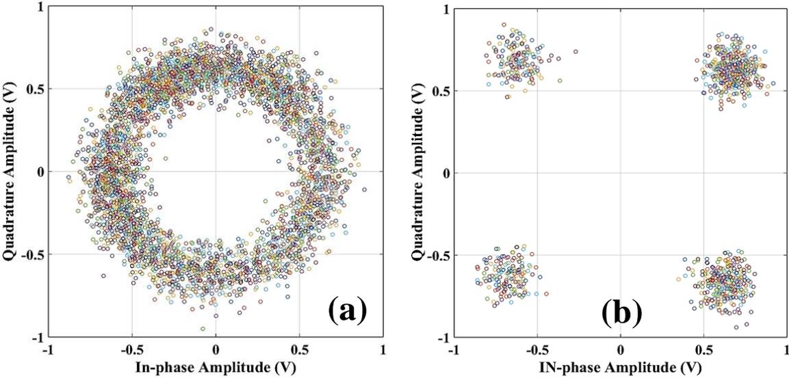
Figure 4.11 The QPSK constellation (a) with Doppler shift, (b) after Doppler frequency shift compensation.
