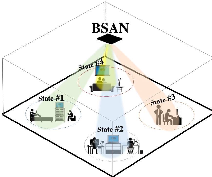
**Figure 5.1** Application of the proposed BSAN (beam-switching antenna network) for the wireless access point (WAP).
