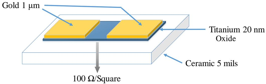
**Figure 3.2** The candidate topology for high-frequency broadband resistors.
