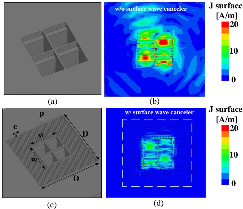
**Figure 5.8** (a) Primary design of the  $2 \times 2$  open-ended waveguide antenna aperture, (b) the simulation results of the induced surface current on the antenna aperture without the employment of surface wave canceler, (c) the proposed design for antenna aperture surrounded by the metal pins as surface wave canceler ( $e=0.6$  mm,  $p=1.43$  mm,  $D=30$  mm, and  $w=15.72$  mm), and (d) the surface current distribution on the proposed design (with surface wave canceler).
