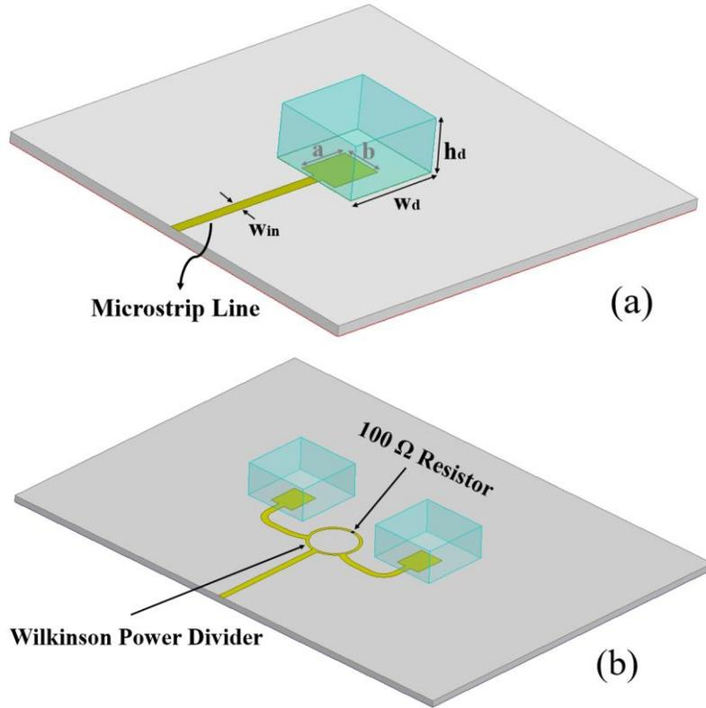
Figure 2.1 3D model of the proposed (a) single element, (b) Two-element DRAs fed by the microstrip line ( $a = 0.6$ ,  $b = 0.5$ ,  $w_d = 1.22$ ,  $h_d = 0.635$ ,  $w_{in} = 0.125$ , all units are in  $mm$ ).
