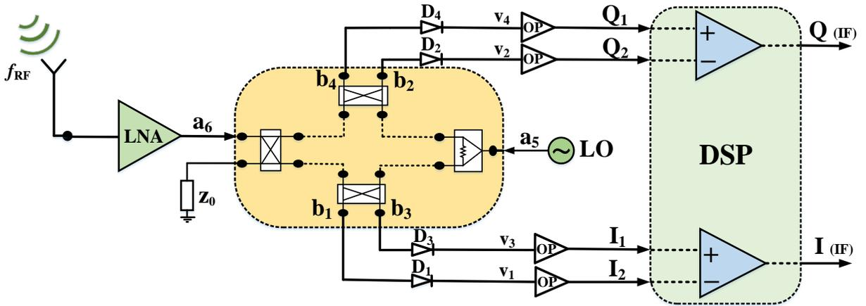
Figure 1.6 Schematic of six-port radio receiver.
