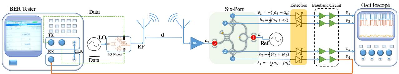
Figure 3.13 The block diagram of applied test setup for measuring BER parameter.
