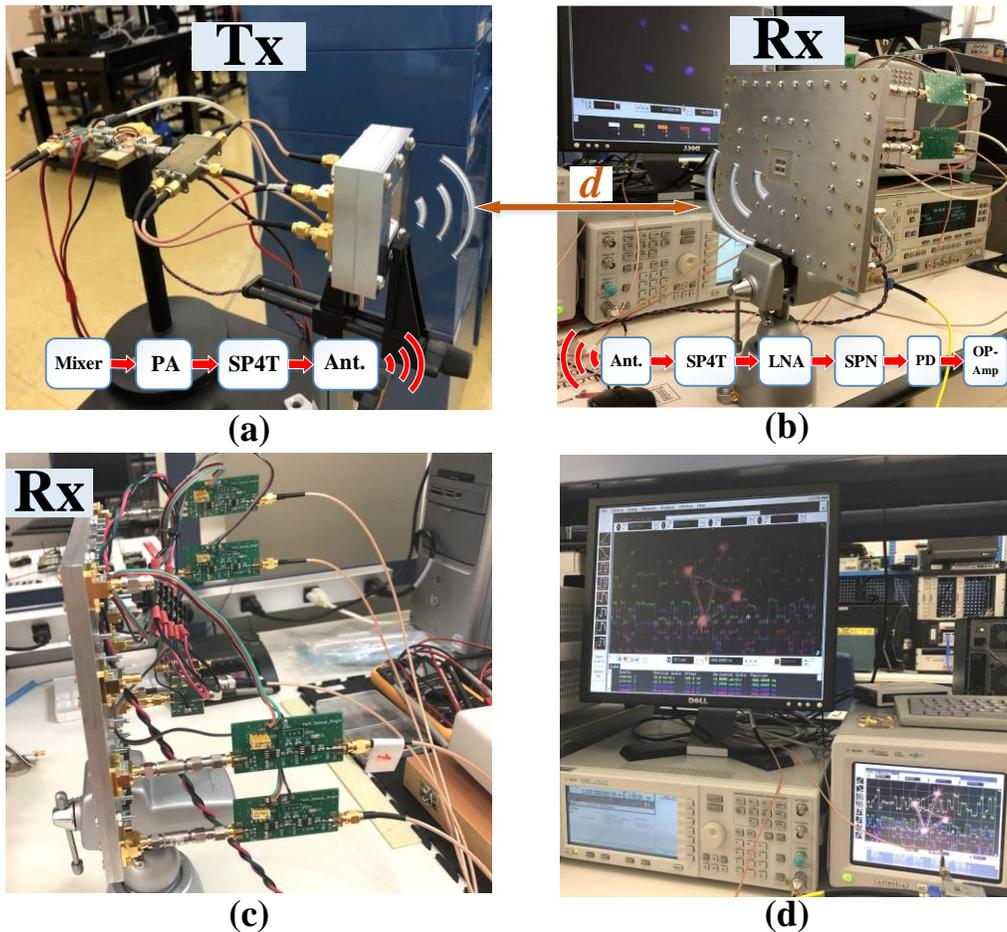
Figure 5.28 Digital photograph of the experimental test bench, (a) transmitter setup, (b) receiver setup, (c) side view of the fabricated design, and (d) demodulated signals on the oscilloscope. (d) the distance between transmitter and receiver antennas, PA: power amplifier, SPN: six-port network, and PD: power detector).
