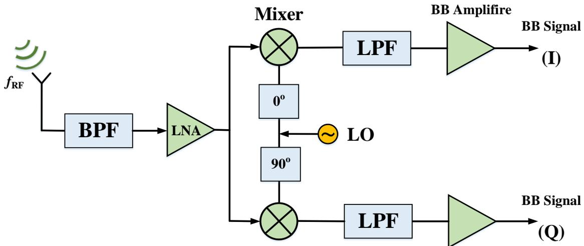
Figure 1.2 Architecture of a quadrature homodyne receiver.
