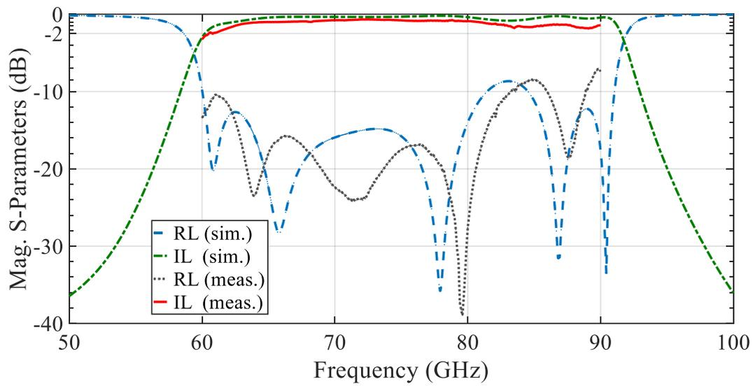
Figure 2.15 The simulation and experimental results of S-parameters for the bandpass filter (RL: Return Loss, and IL: Insertion Loss).
