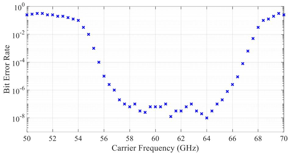
Figure 3.14 The operational bandwidth of the SPI network defined by measured BER.
