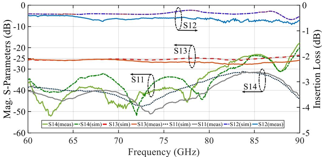
Figure 2.13 The simulation and measurement results of S-parameters for the directional coupler with 25 dB coupling value.
