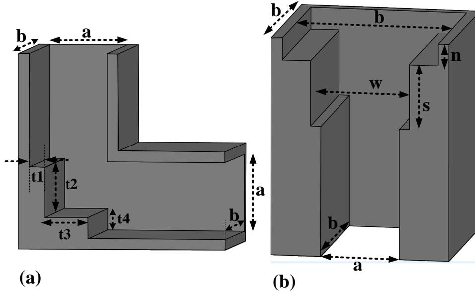
Figure 5.6 Two types of transitions; (a) Transition #1 for converting the horizontal WR28 to vertical WR28 and (b) Transition #2 for converting the WR28 (3.5 mm × 7.11 mm) to the antenna aperture size (7.11 mm × 7.11 mm). (a=3.56 mm, b=7.11 mm, t<sub>1</sub>=0.7 mm, t<sub>2</sub>=2.3 mm, t<sub>3</sub>=2mm, t<sub>4</sub>=1 mm, w=4.5 mm, s=3 mm, n=1 mm).
