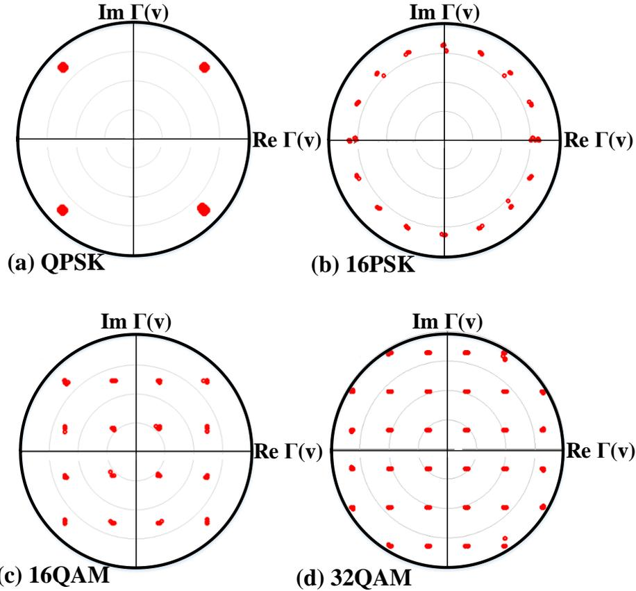
Figure 5.23 The simulated constellation of the demodulated PSK/QAM signals without noise.
