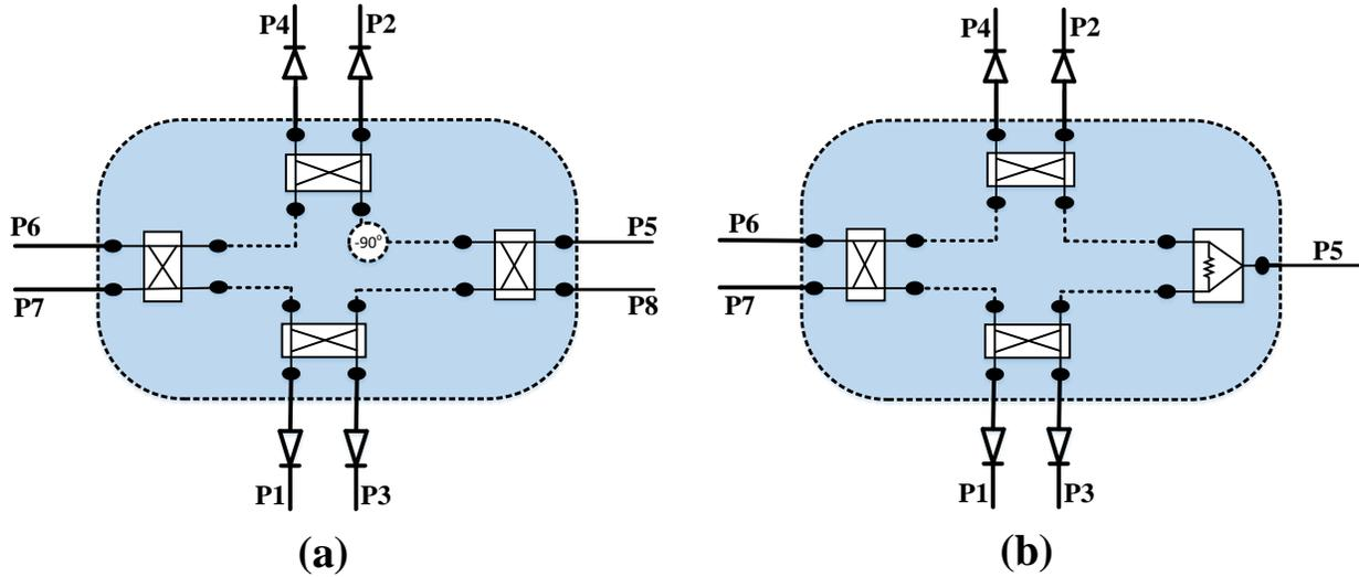
**Figure 1.5** Two common topologies of passive junction for six-port receivers (a) Quadrature hybrids and phase shifter, (b) Quadrature hybrids and power dividers
