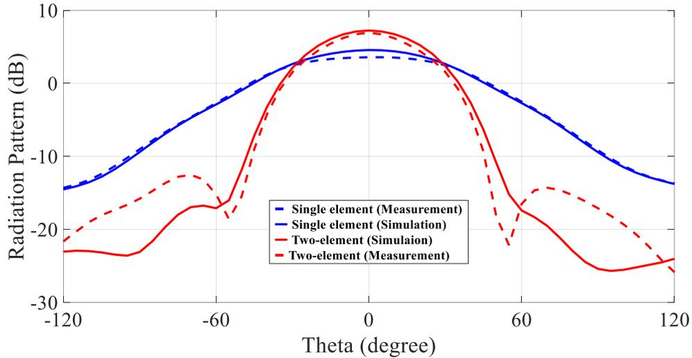
**Figure 2.5** Measured and simulated results of the radiation pattern at 61 GHz regarding to single and two-element DRAs.
