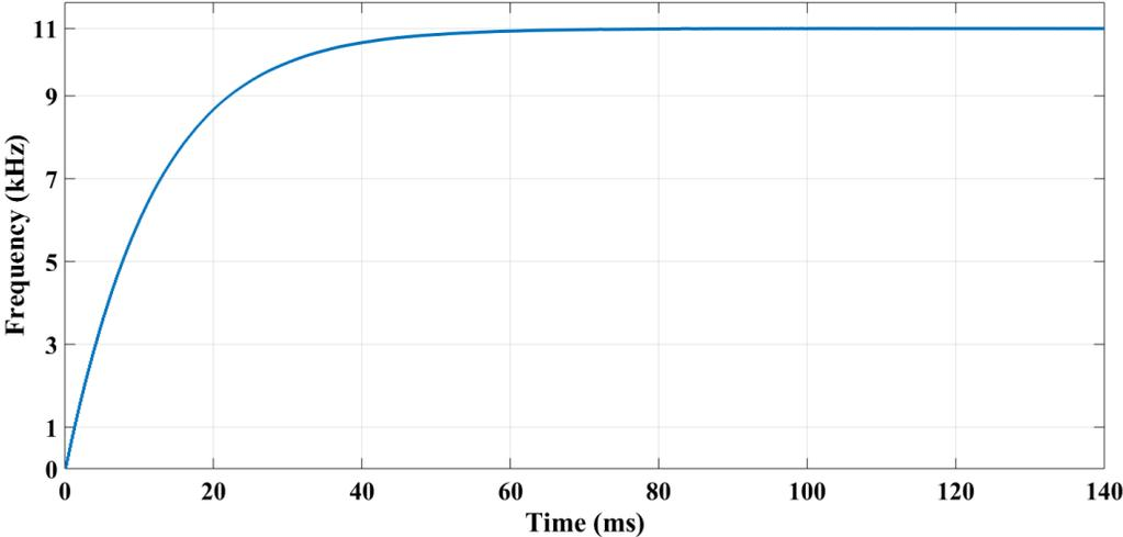
Figure 4.12 Carrier recovery integrator output with 11 kHz Doppler shift.
