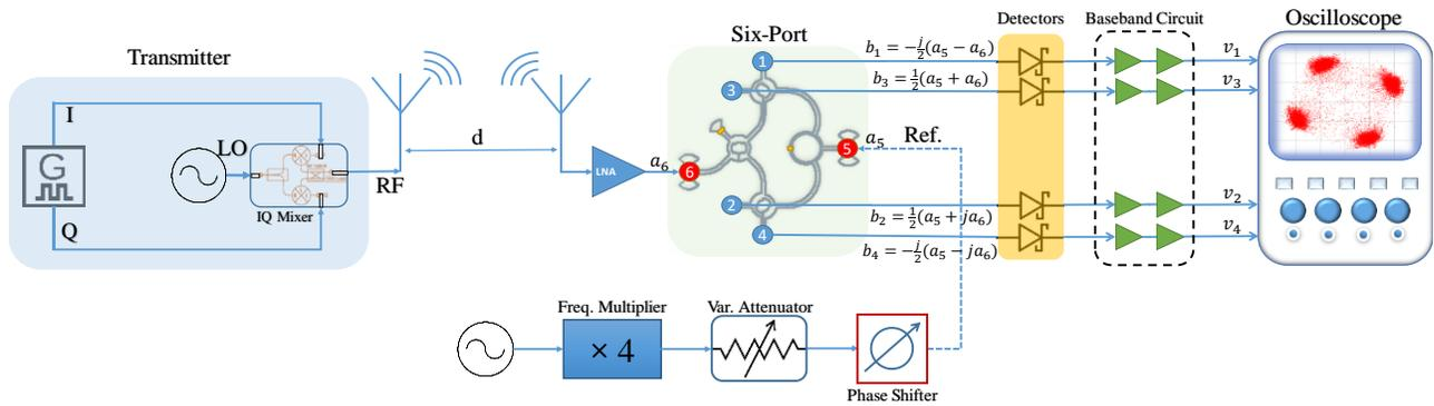
Figure 3.8 The block diagram of the proposed system setup including SPI for measurement of high data rate demodulation signals.
