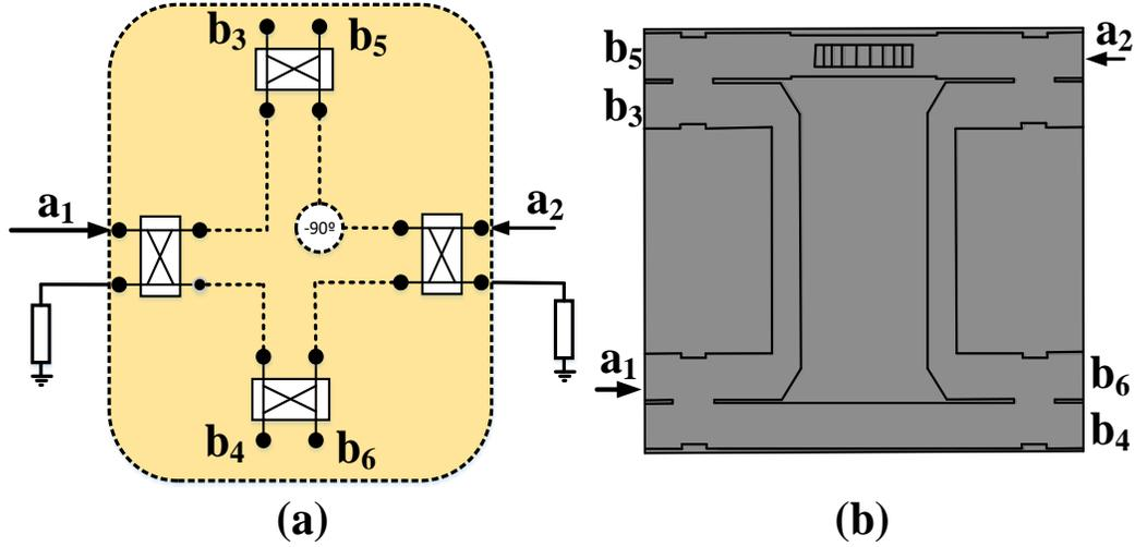
Figure 5.14 (a) The block diagram of the SPN including four 90° hybrid couplers and a 90° phase shifter and (b) the proposed design based on a hollow waveguide showing all ports.
