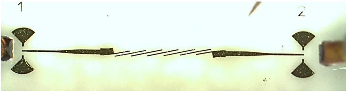
Figure 2.14 A photograph of the fabricated *E*-band bandpass filter.
