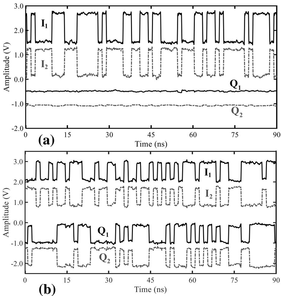
Figure 5.30 Measured demodulation signals of I and Q versus time. (a) BPSK, and (b) QPSK.
