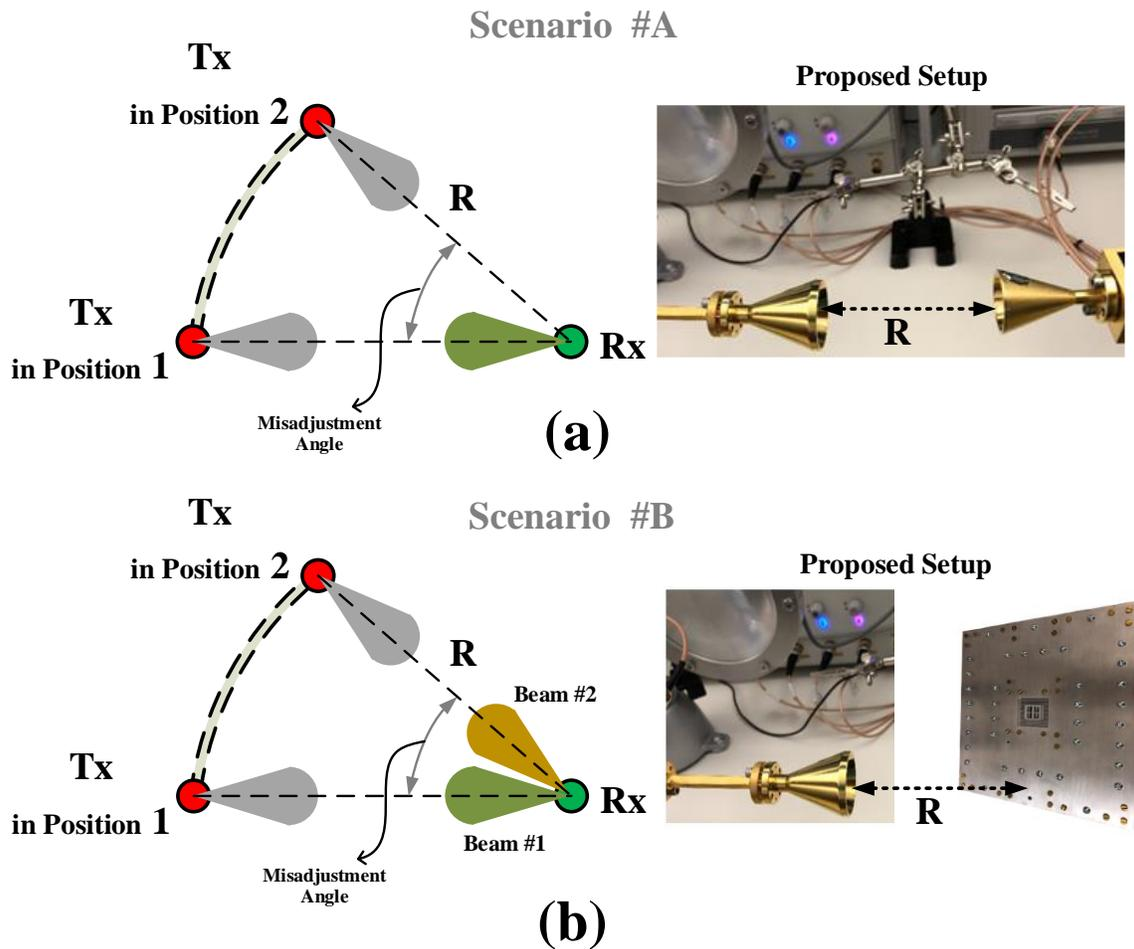
Figure 5.25 Defined scenarios to investigate the beamformer capability for improving link performance. (a) The proposed system with directive horn antenna with  $8^\circ$  beamwidth. (a) The proposed system with the proposed beamformer. Scenario #B is given for the rotated  $xz$ -plane, where beam #1 and beam #2 are radiated.
