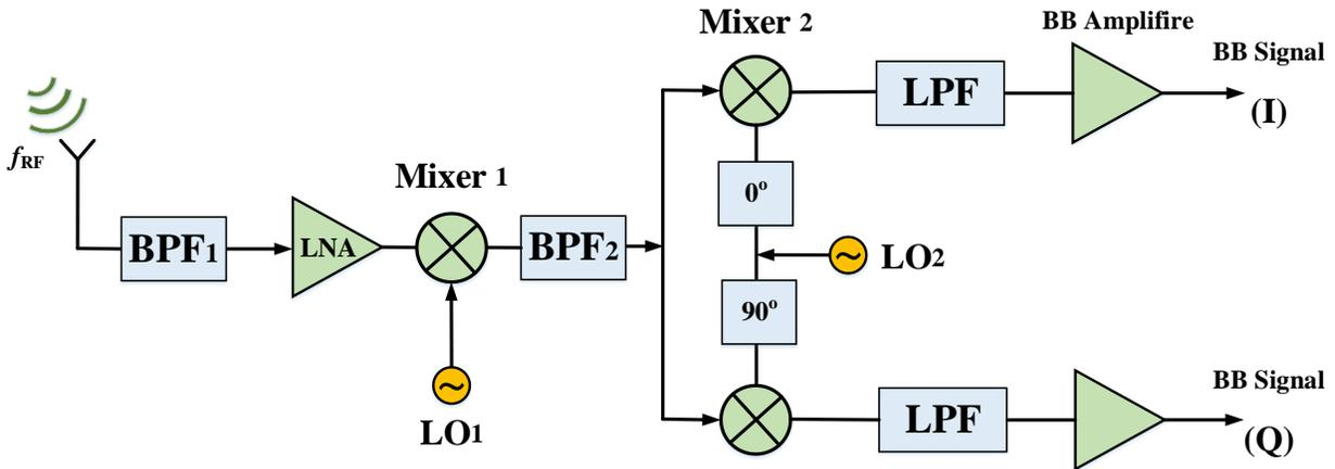
Figure 1.3 Architecture of a heterodyne receiver.
