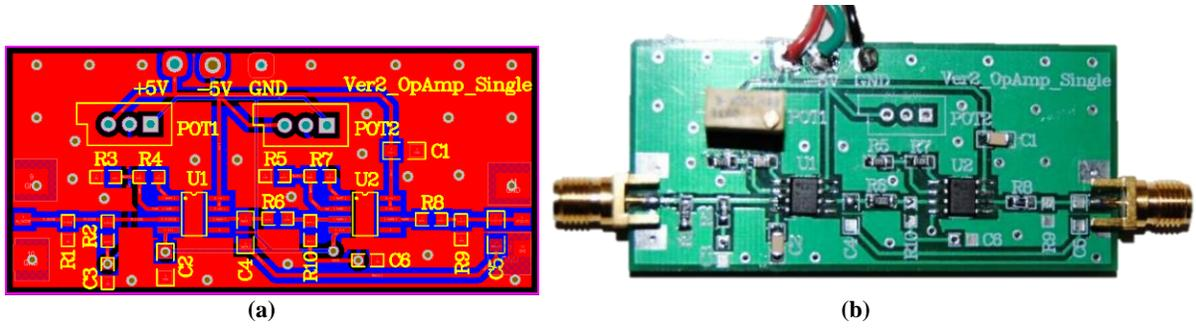
Figure 3.5 (a) The designed layout and, (b) a photo of the fabricated baseband circuit using two cascade op-amp stages.
