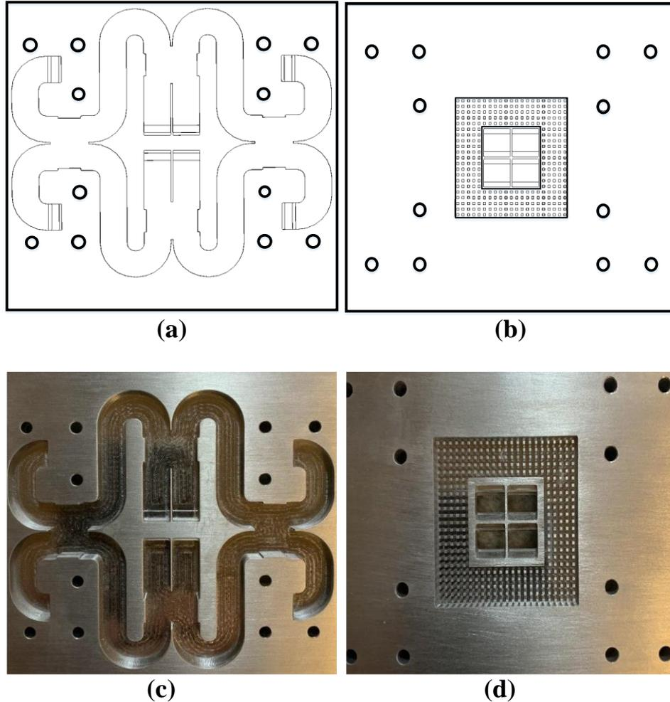
**Figure 5.10** Proposed design of the BSAN; (a) a cut of the middle including the feeding network based on the hollow waveguide, (b) the top view of the structure including the radiating part, (c) the feeding network in the first layer, and (d) photo of the second layer showing the 2×2 open-ended waveguide antenna.
