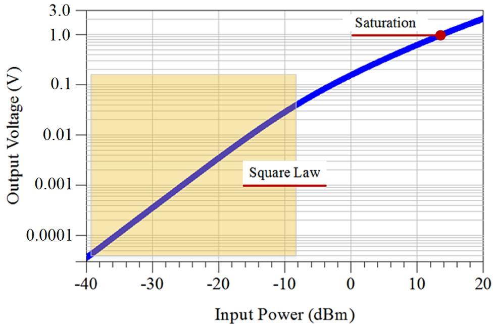
**Figure 1.8** Simulated (V-P) transfer function of the Schottky diode in ADS using the developed HSCH-9161 zero-bias Gallium-Arsenide (GaAs) beam lead diode model.
