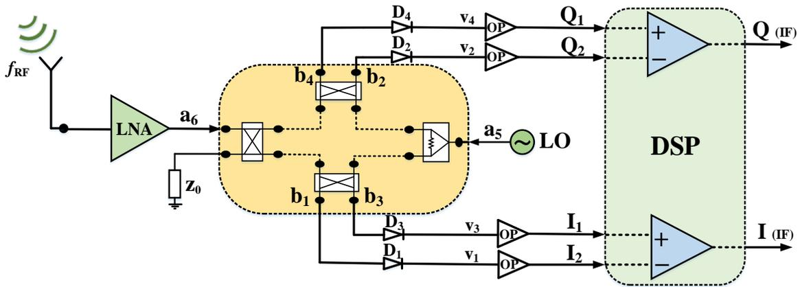
Figure 4.9 The block diagram of the designed six-port receiver.
