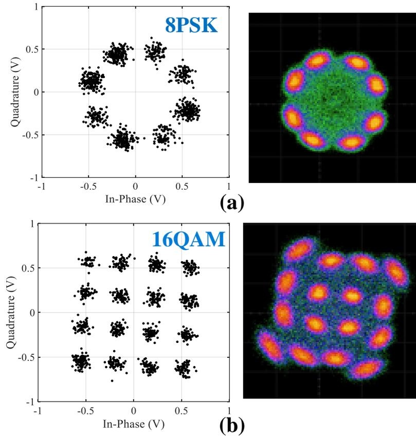
Figure 3.11 Measured I-Q constellation of demodulated high-rate data for selected modulation (a) 8PSK, (b) 16QAM.
