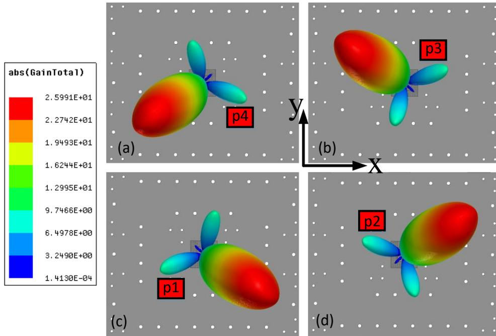
Figure 5.9 Simulated radiation patterns of the proposed BSAN at 30 GHz with respect to the exciting ports; (a) Port 4, (b) Port 3, (c) Port 1, and (d) Port 2.
