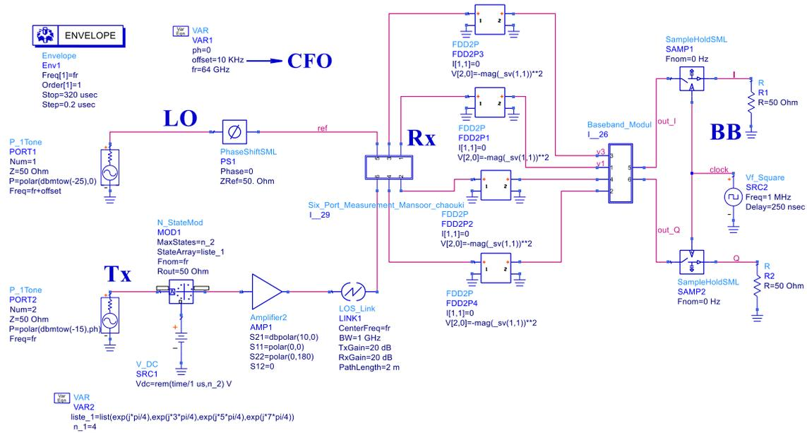
Figure 4.2 The ADS simulation deck of the proposed system for CFO investigation.
