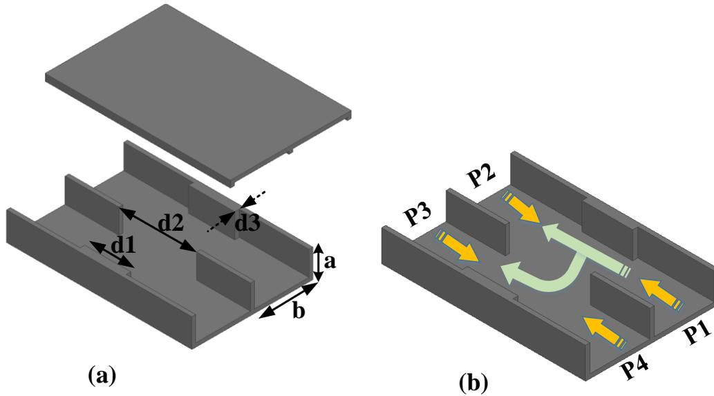
Figure 5.3 Proposed coupler composed of two hollow waveguides with a coupling aperture in the common wall and two distracting appendages. ( $d_1= 6$  mm,  $d_2= 10.1$  mm,  $d_3= 0.6$  mm,  $a=3.56$  mm, and  $b=7.11$  mm). (a) design of the proposed coupler and (b) the sketch of input ports.
