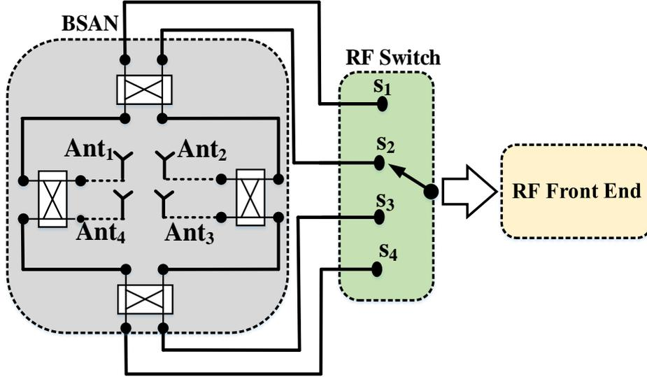
**Figure 5.2** A general sketch of the  $2 \times 2$  BSAN including four inputs connected to RF switch and four outputs as radiating antenna elements.
