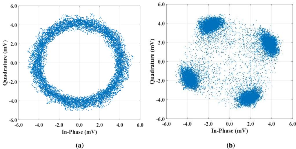
Figure 4.8 The baseband signal constellation (a) with Doppler effect, (b) after compensation for CFO.
