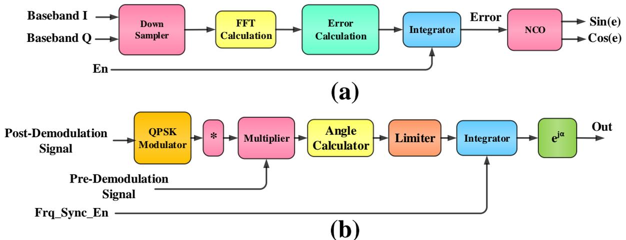
Figure 4.10 The structure of (a) Frequency, (b) Phase Recovery
