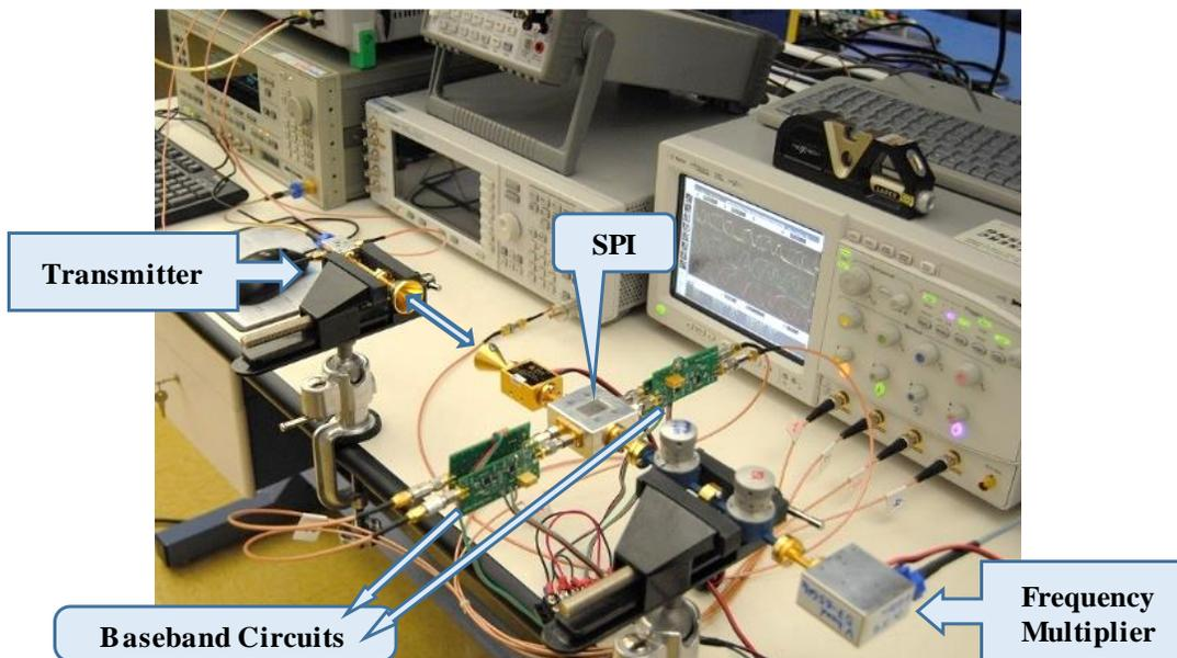
Figure 3.12 The V-band wireless link experimental setup for measuring demodulation results.
