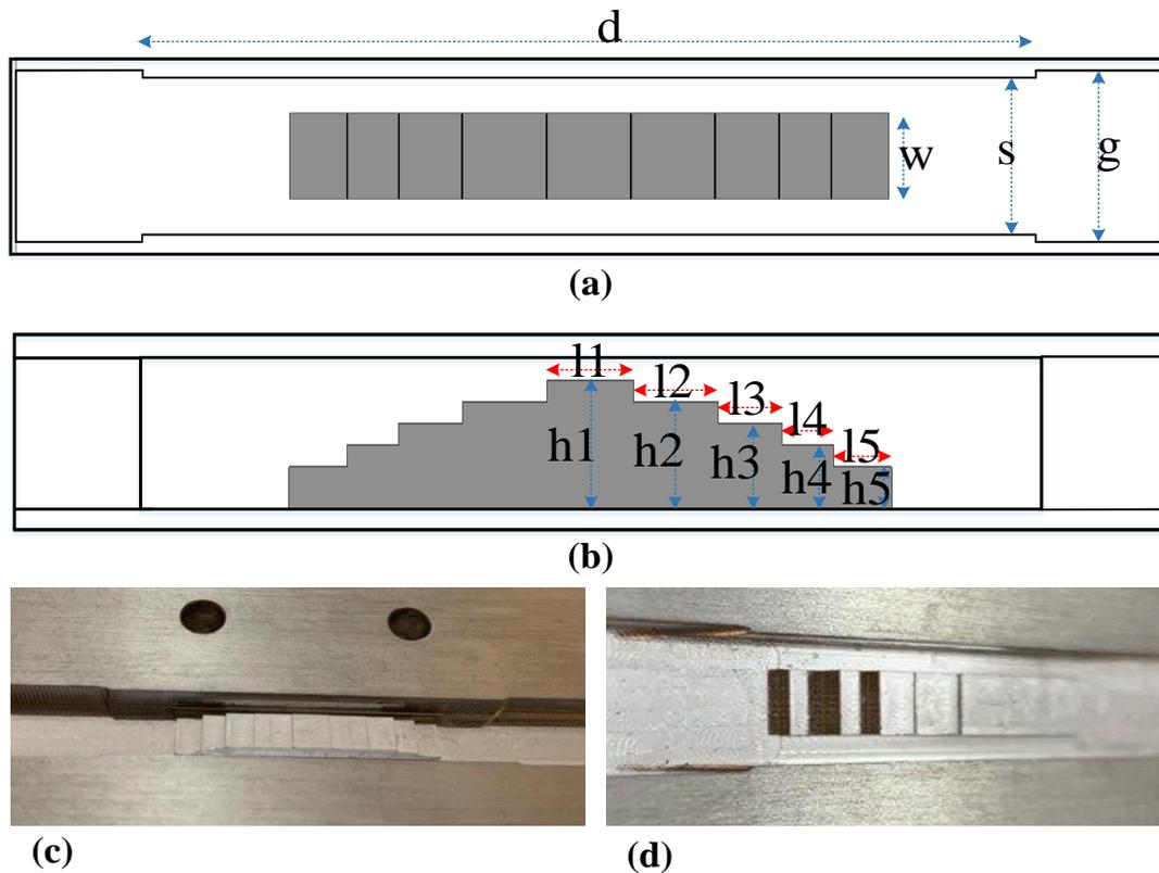
**Figure 5.16** A  $90^\circ$  phase shifter with the design parameters (a) the top view and (b) side view ( $w=3.56$ ,  $s=6.5$ ,  $g=7.11$ ,  $d=35.9$ ,  $l_1=3.44$ ,  $l_2=3.37$ ,  $l_3=2.55$ ,  $l_4=2.06$ ,  $l_5=2.3$ ,  $h_1=2.21$ ,  $h_2=2.1$ ,  $h_3=2.03$ ,  $h_4=1.48$ ,  $h_5=0.6$ ), units in mm.
