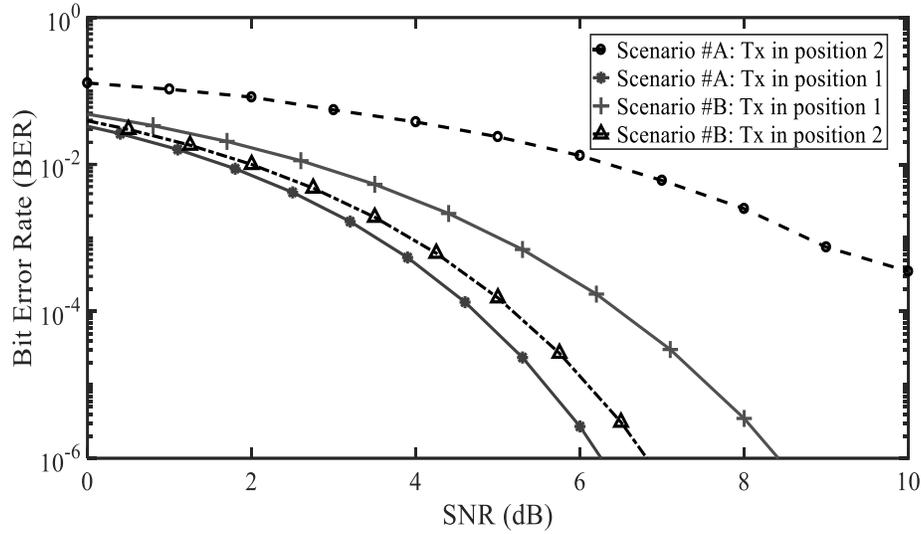
**Figure 5.26** Simulation BER performance for QPSK modulation with 6 GHz bandwidth and data rate of 1 Gb/s, concerning the defined scenarios in Figure 5.25.
