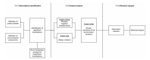
Figure 7.1 Schematic representation of the matrix approach methodology ([Consultants LEGOFF Groupe inc., 2005], p.179, simplified version)
