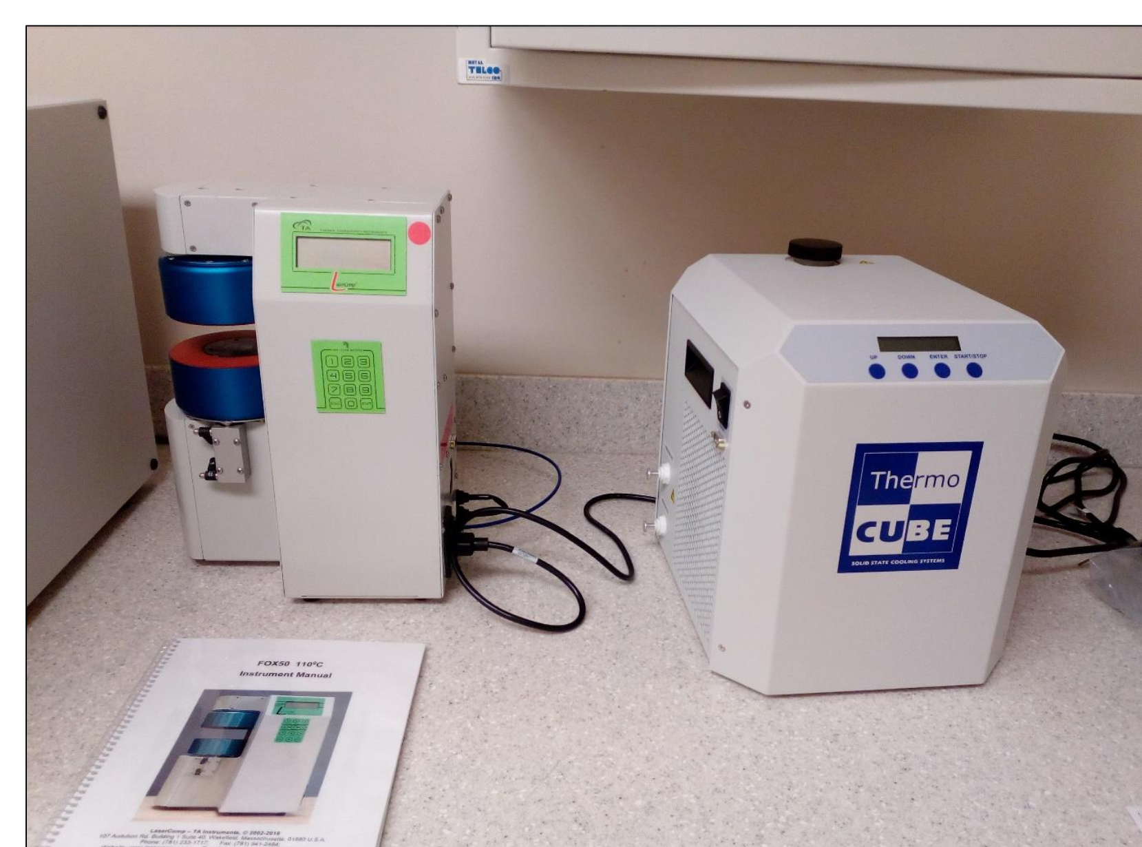
Fig. 5. FOX50 Heat Flow Meter – steady state guarded hot plate method. Measurements of thermal conductivity and heat capacity in the range -10 to 190 °C (Raymond et al., 2017).
