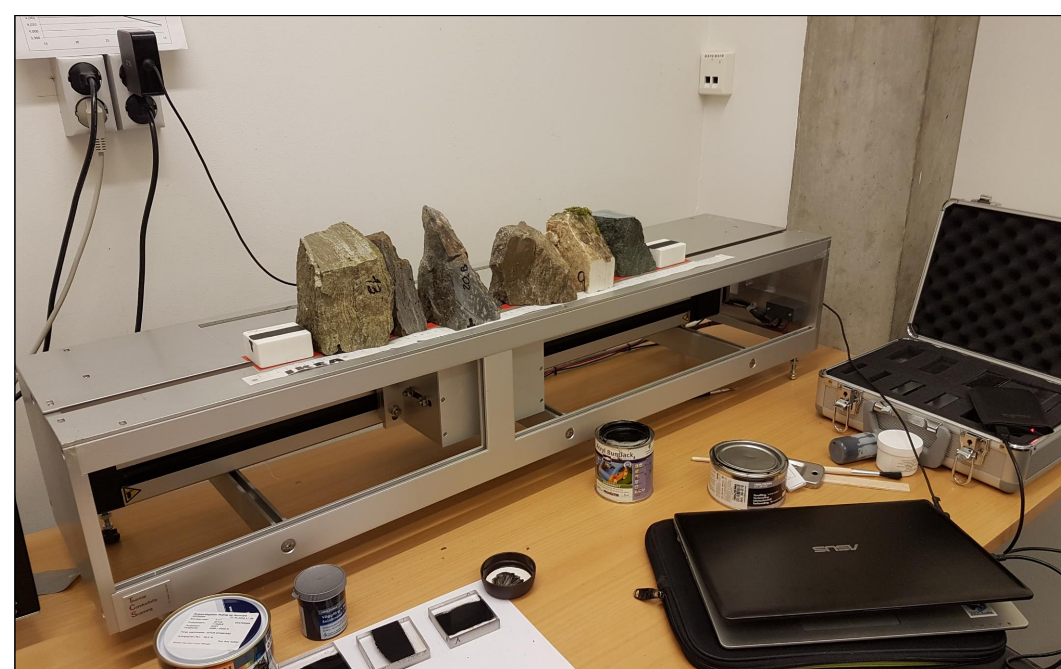
Fig. 4. TCS – optical scanning method (Popov et al., 2016). Measurements of thermal conductivity and diffusivity at room temperature.
