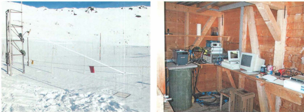
Figure 3 - The cable sensor system at Weissfluhjoch Davos (2550 m): the sloping flat-band cable (left), and the electronic devices in the shelter (right).
