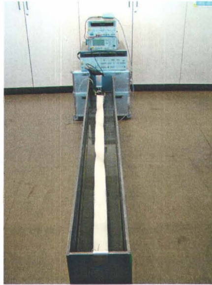
Figure 2 - Laboratory set-up and tank used for calibration
