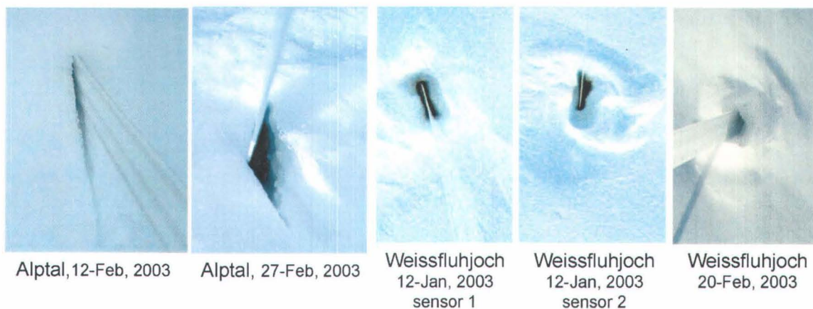
Figure 20 - Observations of air gaps at the snow surface in the vicinity of the snow cable sensor.
