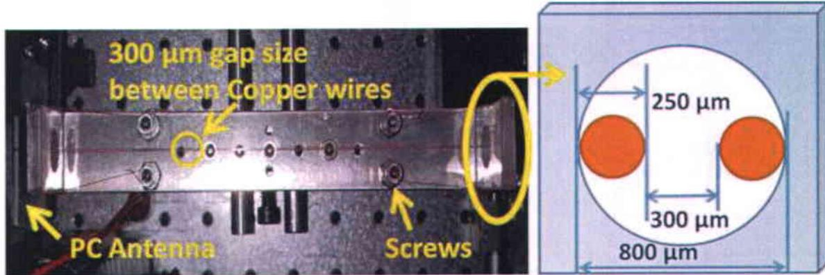
Fig. 2.5 Designed two-wire waveguide structure with the schematics of the arrangement used to keep the wire separated in air by  $300 \mu\text{m}$ .
