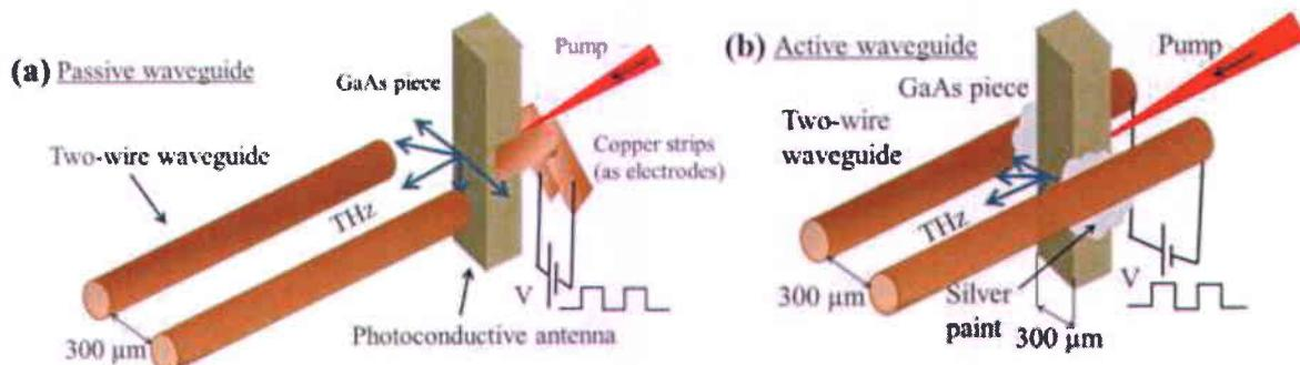
Fig. 4.1 Schematics of the (a) passive and (b) active waveguide. The arrows denote the direction of THz radiation emitted from the GaAs piece.
