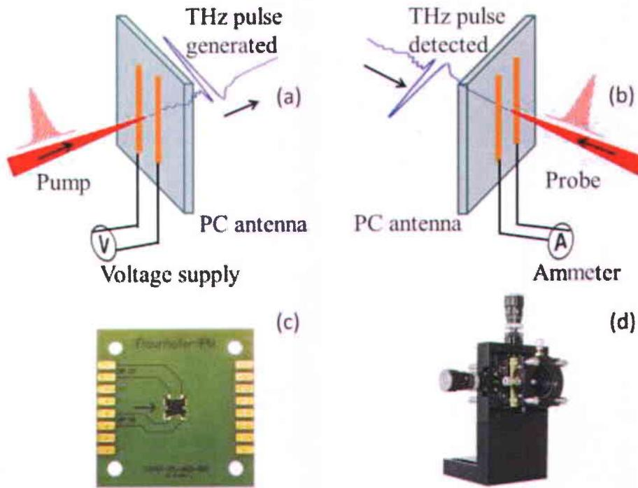
Fig. 1.2 (a) Terahertz PC (photoconductive) antenna as a source and (b) as a detector with arrows indicating the direction of propagation. (c) A commercially available PC antenna (Tera-8 from Menlo Systems) and (d) its mount.
