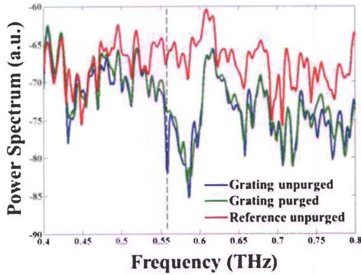
Fig. 3.6 Enhancement of water absorption at 0.557 THz (dashed line) as shown by the blue curve (grating spectrum in unpurged conditions). The red curve indicates the waveguide signal spectrum in ambient conditions (unpurged) and the green curve shows the grating spectrum in purged conditions.
