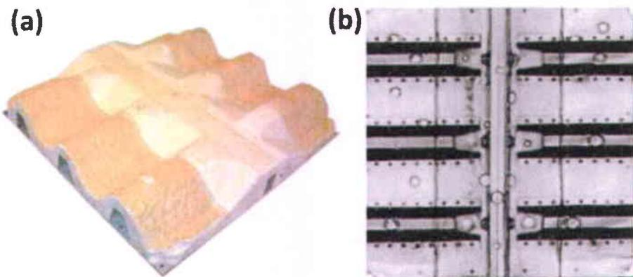
Fig. 1.5 (a) Optical photo of a  $2 \times 2$  panel sample and (b) its THz wave image [47].
