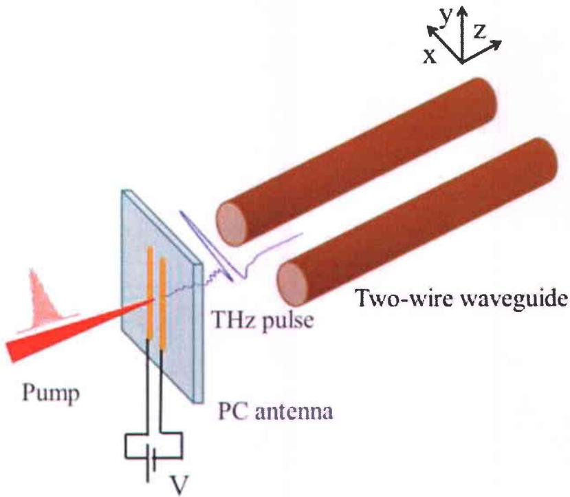
Fig. 2.6 Coupling scheme for the two-wire waveguide lying on x-z plane, with its transverse section perpendicular to z direction. The THz pulse is polarized in the x direction.
