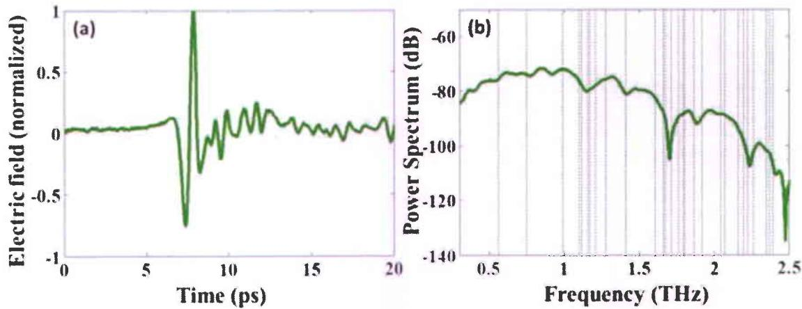
Fig. 2.8 (a) THz signal from the 20 cm long two-wire waveguide in ambient air and (b) its spectrum, where the dashed lines represent water absorption lines. All curves are normalized to their peak.
