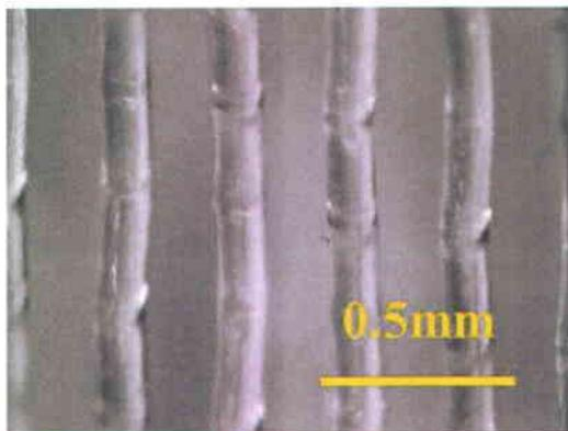
Fig. 3.2 Photograph of the polymer Bragg grating comprising of polymer rods used for achieving frequency filtering in the two-wire waveguide.
