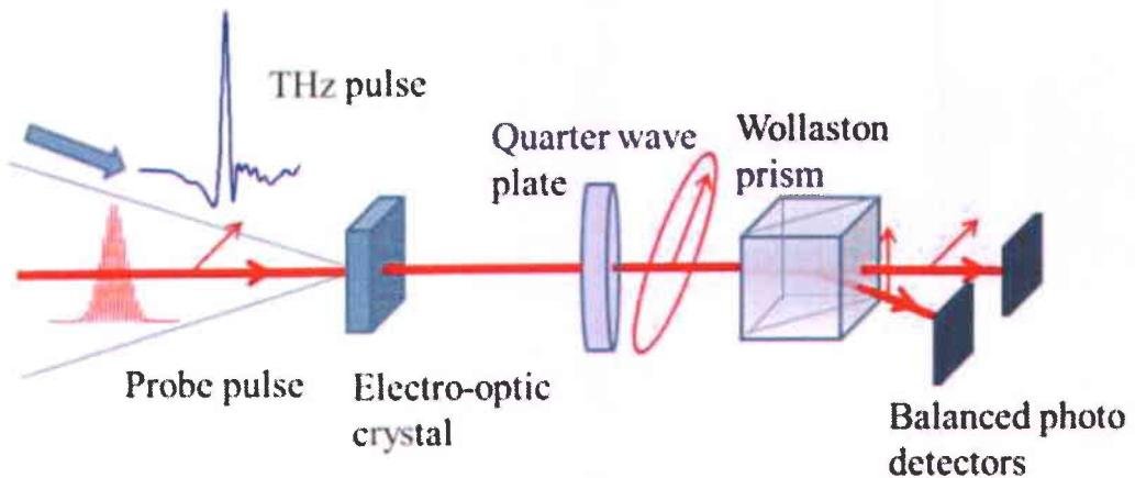
Fig. 1.4 Schematics of detection by electro-optical sampling technique. The THz radiation is focused on the electro-optic crystal where it modulates the polarization of the probe pulse. The arrows indicate the final polarization directions of the probe pulse.
