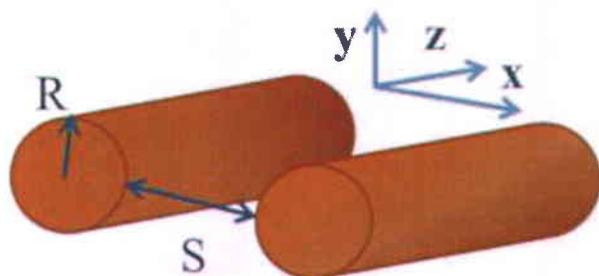
Fig. 2.1 Scheme of a two-wire waveguide with separation  $S$  and radius  $R$ . The two-wire mode lies in the  $x$ - $y$  plane and the mode propagates in the  $z$  direction.
