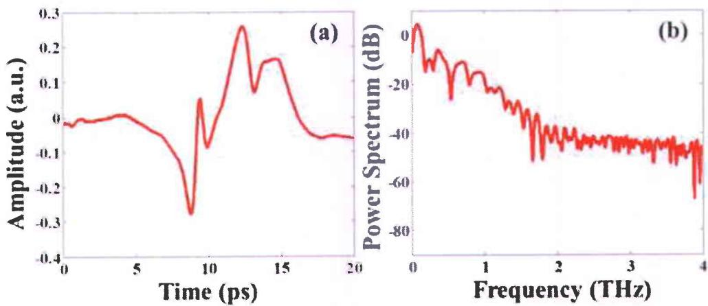
Fig. 4.4 (a) Signal from 10 cm waveguide with GaAs piece inserted between two wires (normalized to the peak of the PC antenna's signal) and (b) its power spectrum (normalized to the peak of the PC antenna's spectrum).
