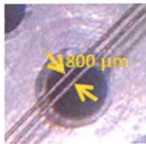
Fig. 2.4 Photograph of the two wire waveguide consisting of two copper wires of  $250 \mu\text{m}$  diameter separated by  $300 \mu\text{m}$  in free space.
