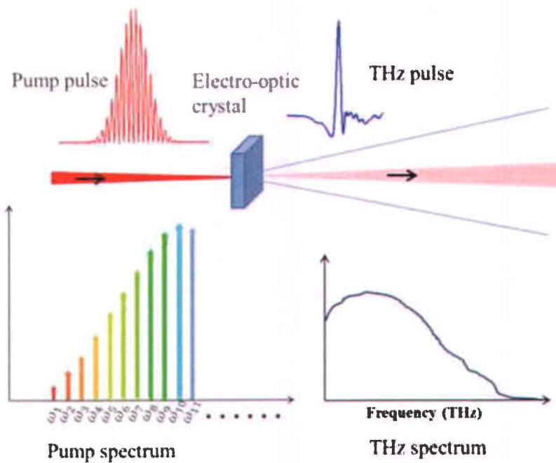
Fig. 1.3 Schematics of THz generation by optical rectification technique. The different frequency components of the mode locked laser beam ( $\omega_1, \omega_2, \omega_3, \dots$ ) undergo DFG to generate a broadband THz spectrum.
