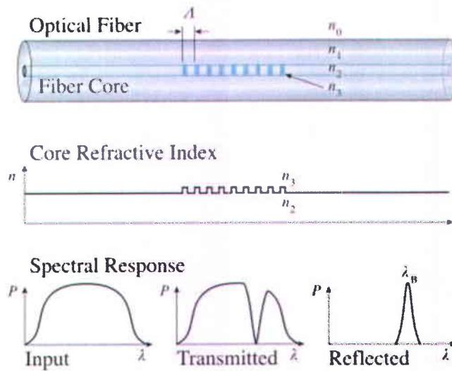
Fig. 3.1 Optical fiber based Bragg grating with the refractive index variation and spectral response (Figure source [88]).
