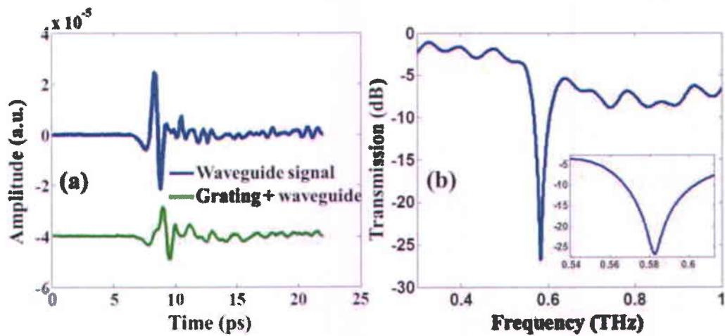
Fig. 3.3 (a) Signal from the waveguide (blue) and with the grating inserted in it (green) (b) Transmission Spectrum of the signal detected after inserting the grating in the waveguide with the inset showing a close view of the dip.
