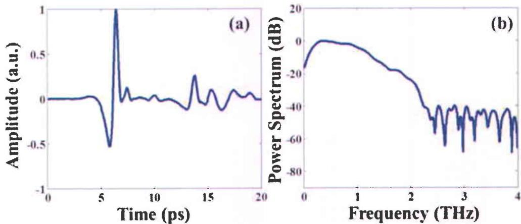
Fig. 4.2 GaAs piece used as a PC antenna: (a) signal, (b) power spectrum. All curves are normalized to their peaks.
