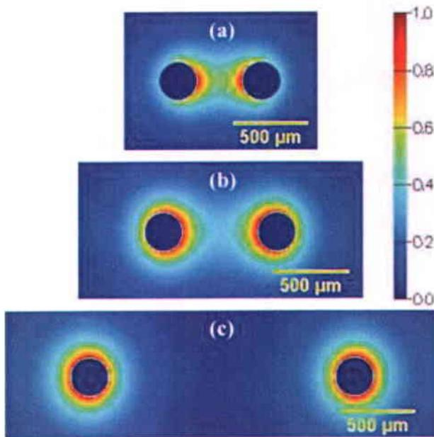
Fig. 2.2 Mode distribution of a 1 THz wave in a two-wire waveguide with a wire radius of 125  $\mu\text{m}$  and a wire separation of (a) 300  $\mu\text{m}$ , (b) 500  $\mu\text{m}$  and (c) 1500  $\mu\text{m}$ .
