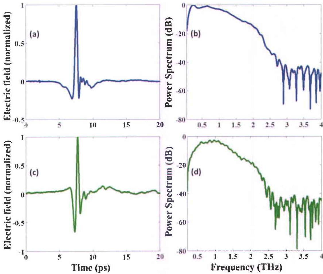
Fig. 2.9 (a) THz signal emitted by the PC antenna in a purged setup and (b) its spectrum. (c) THz signal from the 20 cm long two-wire waveguide in a purged setup and (d) its spectrum. All curves are normalized to their peak.
