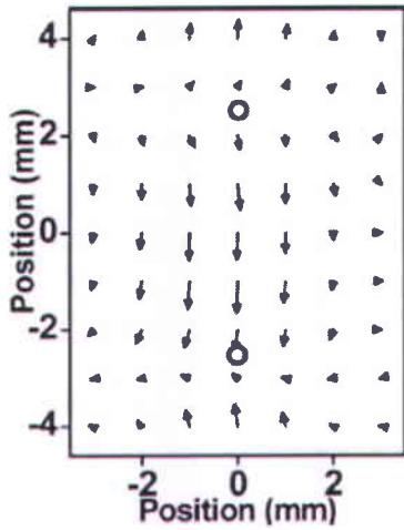
Fig. 2.3 Dipole like field distribution in the two-wire waveguide with distance between the two wires of 4.7mm [71].
