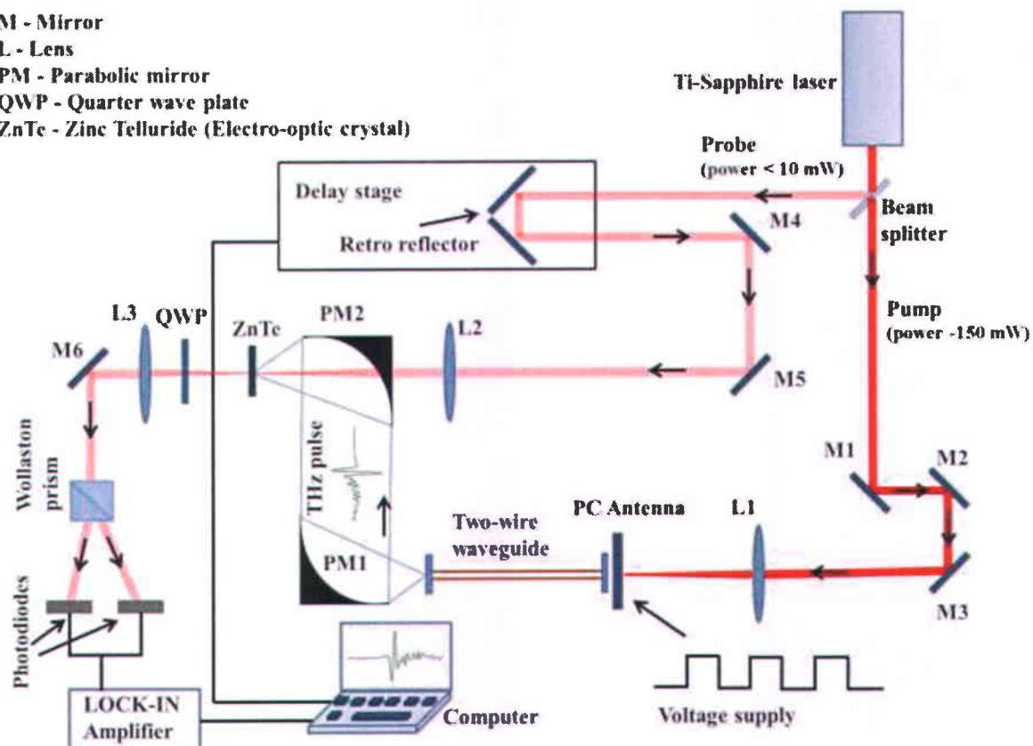
Fig. 2.7 Experimental scheme for the THz waveguide characterisation.
