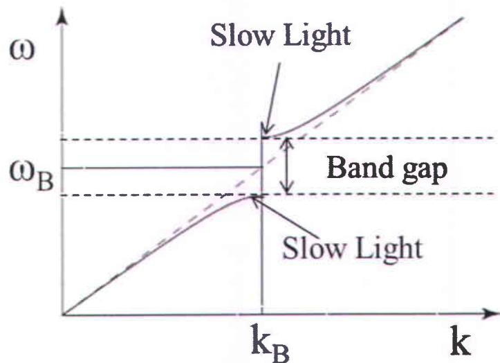
Fig. 3.5 Dispersion curve of a Bragg grating structure with Bragg frequency  $\omega_B$  showing its band gap and indicating the region of slow-light formation near its band edge (adapted from [109]).
