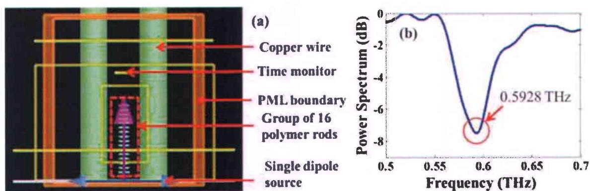
Fig. 3.4 (a) Snapshot of the FDTD simulation setup (top view) of the polymer Bragg grating inserted in the two-wire waveguide. (b) Power spectrum of the grating response recorded by the time monitor in the FDTD simulation with the dip at 0.5928 THz.
