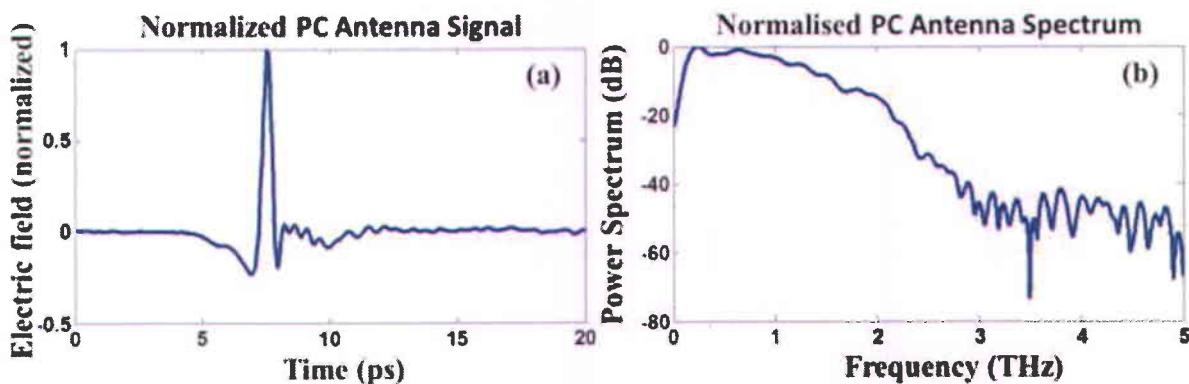
Fig. 1.1 (a) THz signal and (b) its corresponding spectrum generated by a PC antenna and detected via electro-optical sampling. All the curves are normalized.
