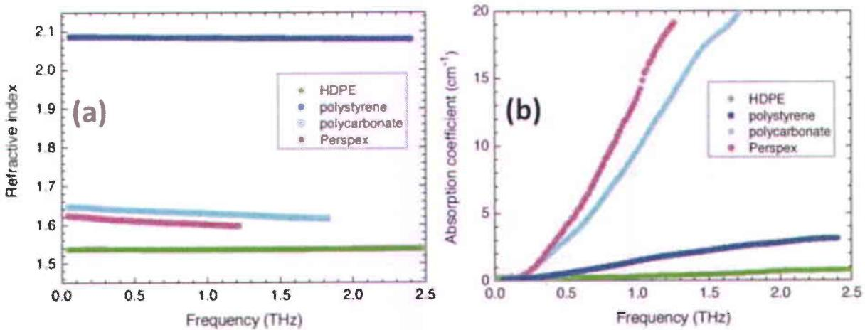
Fig. 1.11 (a) Refractive index profile and (b) absorption spectrum of some commonly used Polymers in the THz region (figure source [13]).
