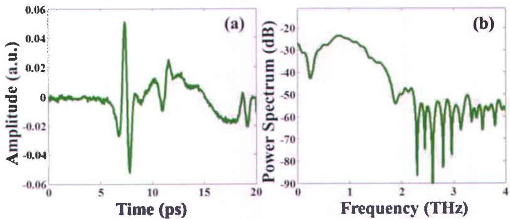
Fig. 4.3 (a) Signal from the 10 cm waveguide with GaAs piece being used as an external PC antenna (normalized to the peak of the PC antenna's signal) and (b) its power spectrum (normalized to the peak of the PC antenna's spectrum).
