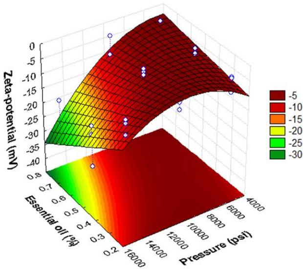
Figure 6.2. Combined effect of EO and pressure on the Zeta-potential of nanoemulsion (concentration of CNC was fixed at 7.5 % (w/w))
