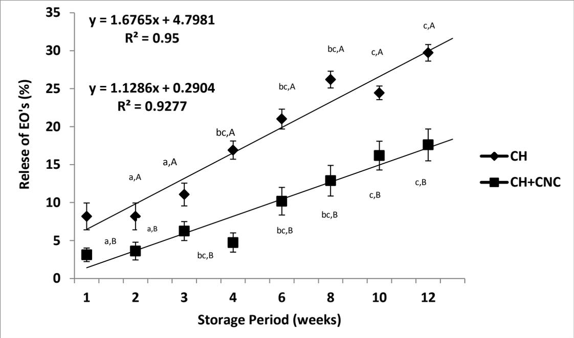
Figure 7.2. Release (%) of EO's from bioactive CH and CH+ CNC based films during storage.
