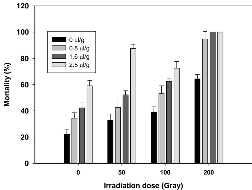
Figure 3.5. Effects of combined treatments with different concentrations of basil EO and gamma radiation on mortality of *S. oryzae* in (i) paper bag and (ii) plastic bag.
