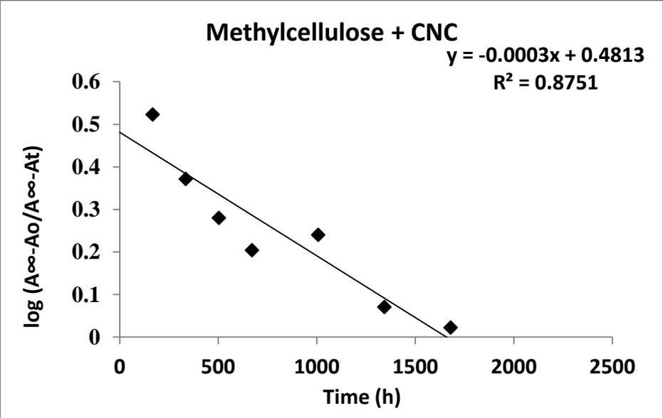
Figure 6.6. Kinetics for release study for i) MC ii) MC + CNC nanocomposite films containing EO nanoemulsion.
