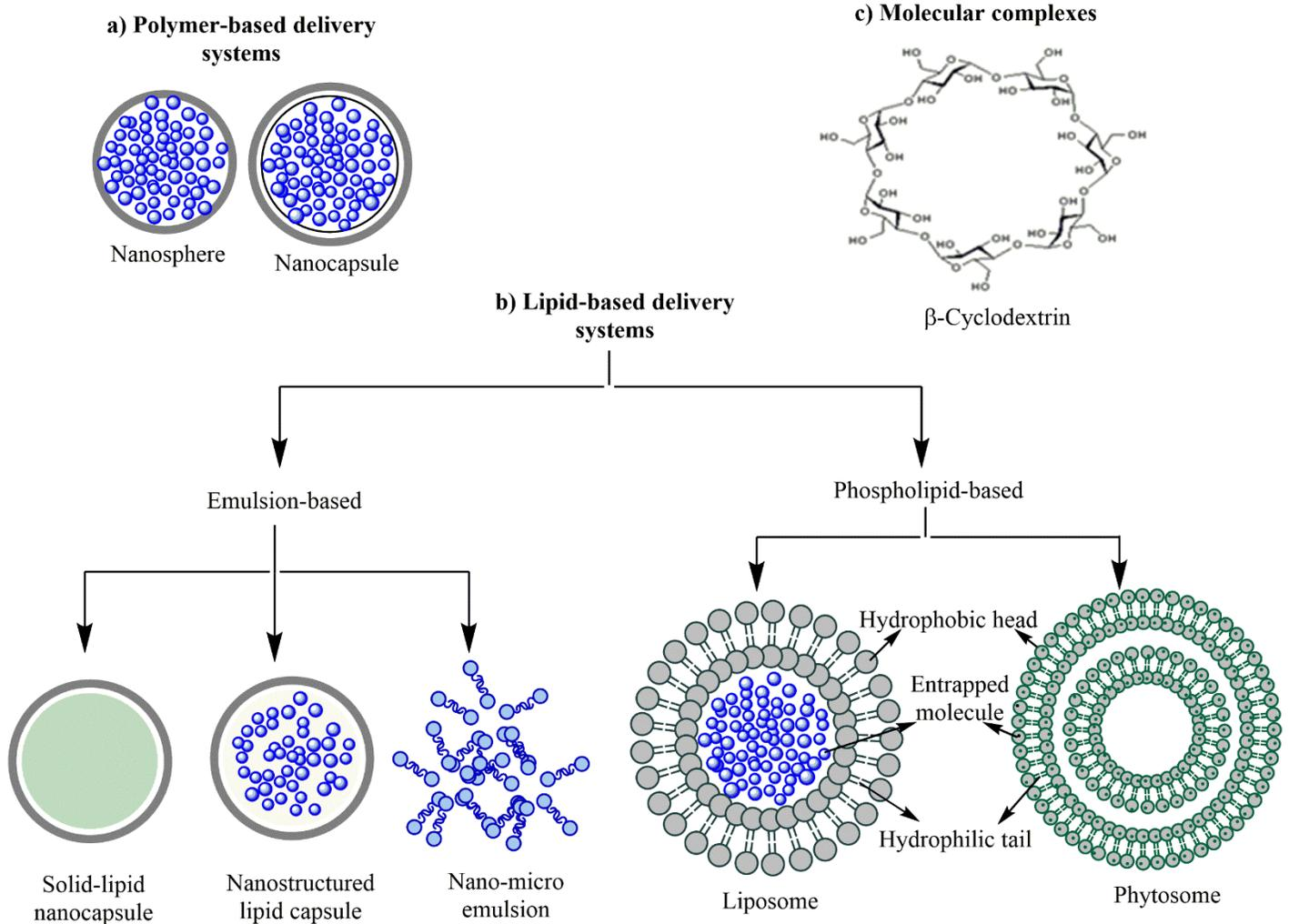
Figure 1.3. Schematic diagram showing nano-based strategies for EO entrapment. a) Polymer-based delivery systems, b) Lipid-based delivery systems, and c) Molecular complexes. Adapted from Bilia, et al. (2014); Ting, et al. (2014) with modifications.
