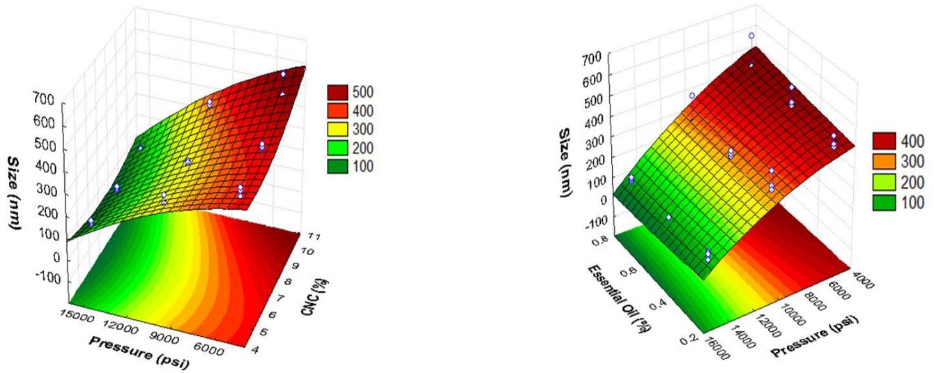
Figure 6.1. Combined effect of a) CNC and pressure (concentration of EO was fixed at 0.05 % (w/v)) and b) EO and pressure (concentration of CNC was fixed at 7.5 % (w/w)) on the particle size of nanoemulsion
