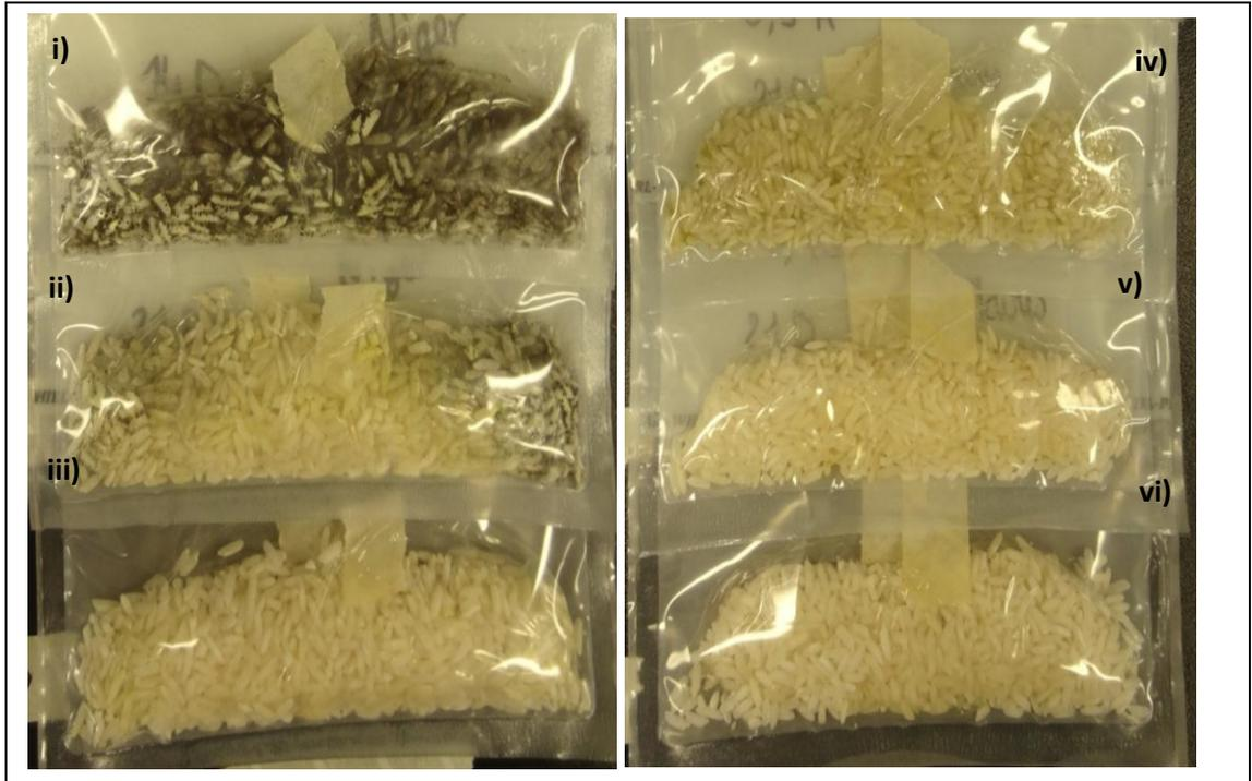
Figure 7.5. Photographic images of rice samples inoculated with *A. niger* with control samples i) CH-CNC (no EOs) ii) Bioactive film A ii) Bioactive film B. iv)  $\gamma$ -CH-CNC (no EOs) v)  $\gamma$  Bioactive film A vi)  $\gamma$  Bioactive film B after 8 weeks of storage.
