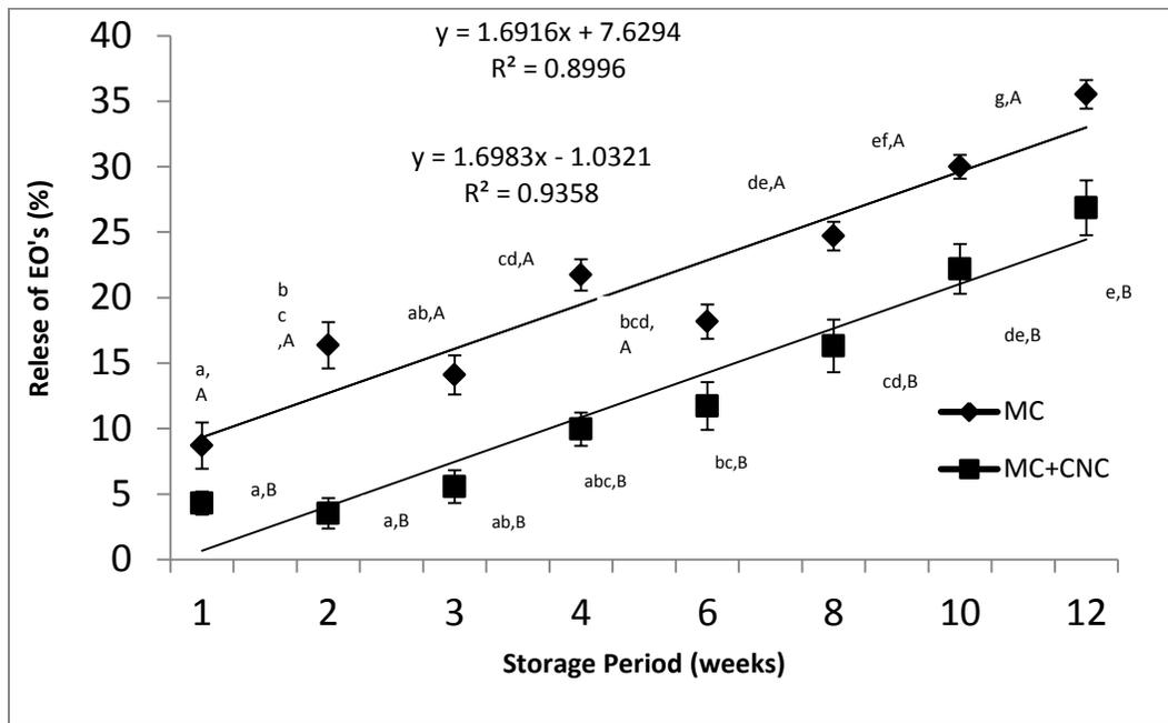
Figure 6.5. Release (%) of EO's from bioactive MC and MC+ CNC based films during storage
