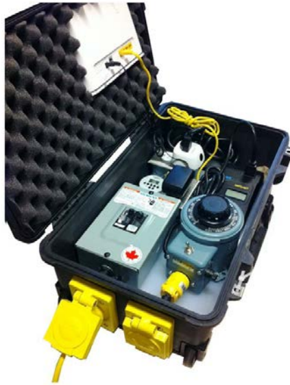
Figure 2.3. Junction box for TRT with a heating cable.
