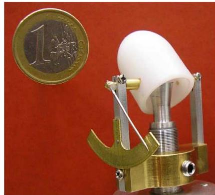
**Figure 1.2      A compact beam-steerable lens antenna [27].**
