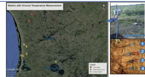
Fig.2. (a) Experimental sites, (b) Sensors installation
