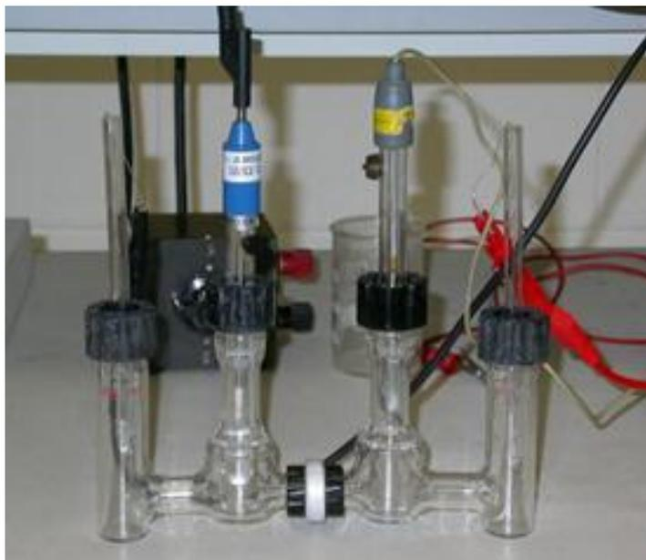
**Figure 3.14:** Four electrodes glass cell used for through-plane proton conductivity measurements.
