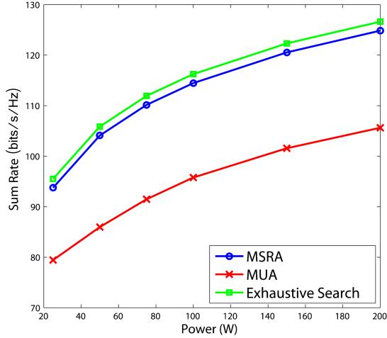
**Figure 3.2:** System sum rate versus satellite power
