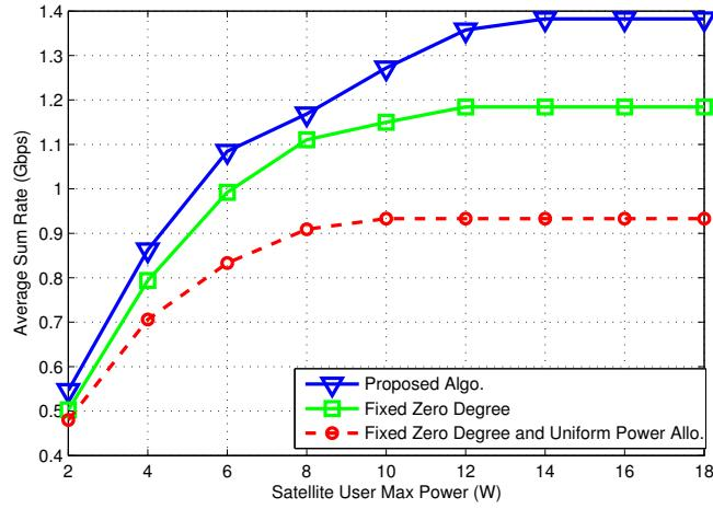
**Figure 4.4:** Average sum rate vs max power of satellite user for  $K=14$ ,  $J=7$ , average SNR=15dB,  $\bar{I}_{i,n}^{\text{TH}}$ 's are set randomly.
