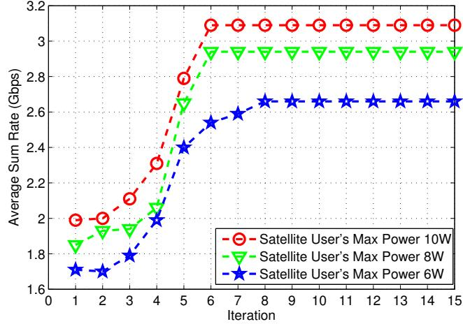
**Figure 4.2:** Convergence of ASRM alg. for  $K=14$  users,  $J=7$  beams, average SNR=15dB,  $I_{i,n}^{\text{TH}}$ 's are set randomly.
