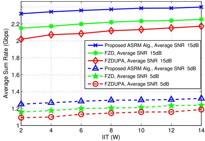
**Figure 4.3:** Average sum rate vs interference threshold increment for  $K=14$  users,  $J=7$  beams.
