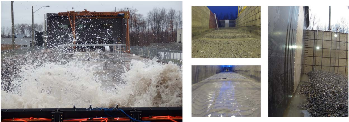
Figure 10. Suspended sediment, sediment transport, beach deformation and local scour (~20 cm/15 impacts).
