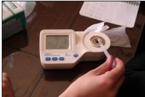
Figure 11 : Using the sea water refractometer to measure ice salinity.
