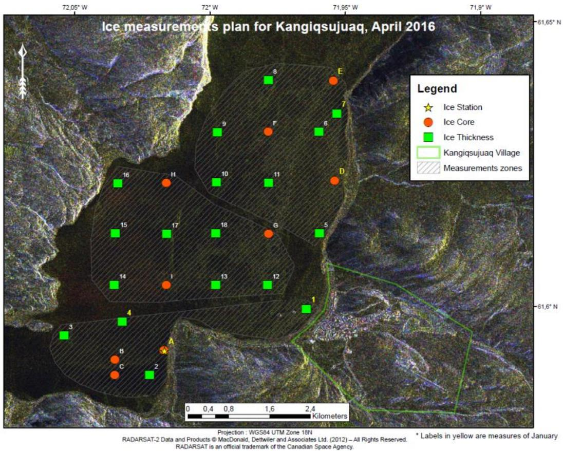
Figure 8 : Sampling pattern for the Kangiqsujuaq measurements.
