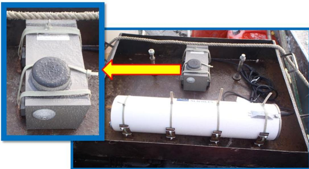
**Figure 21 : The SWIP (grey box), the battery (white cylinder) and the anchor.**
