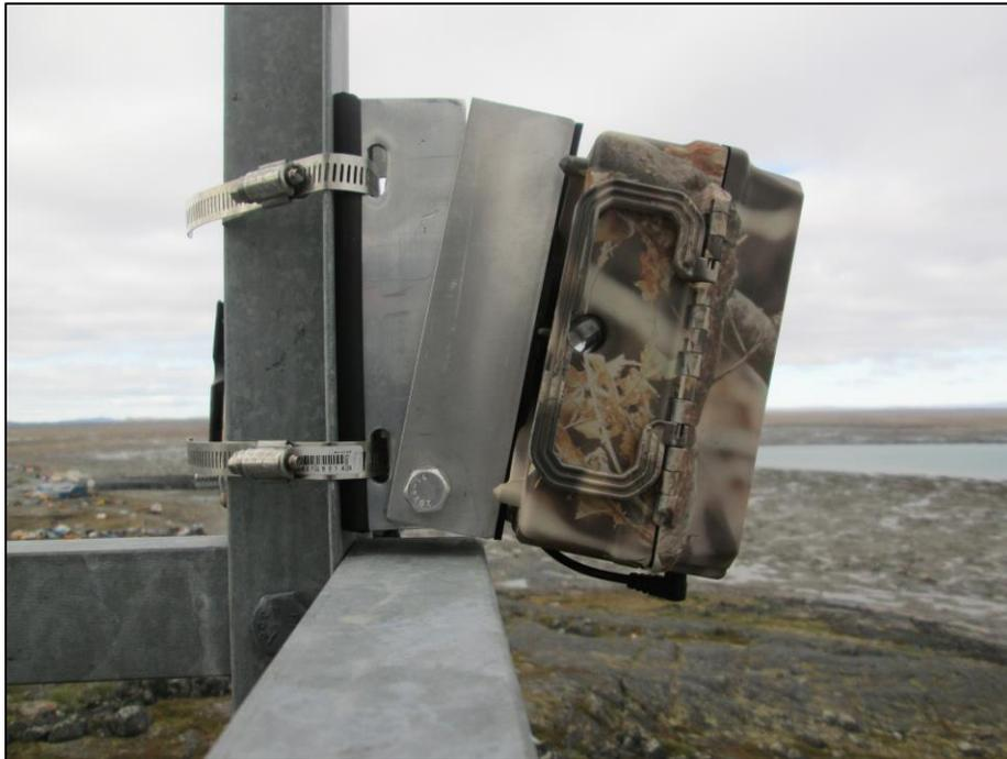
**Figure 30 : Support for Reconyx cameras (Photo from Aupaluk)**
