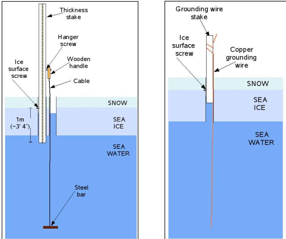
Figure 19 : Hot wire gauge (from Mahoney and Gearheard)
