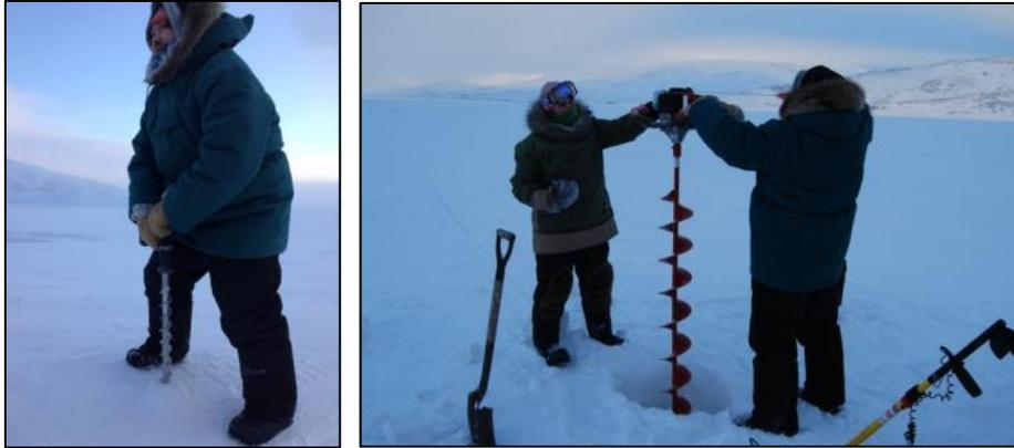
Figure 9 : Drilling with the Kovacs auger (left) and Jiffy auger (right)
