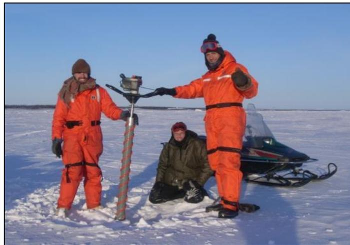
Figure 32: Use of a Kovacs ice corer for vertical ice profiling by INRS team (Koksoak River, 2009).
