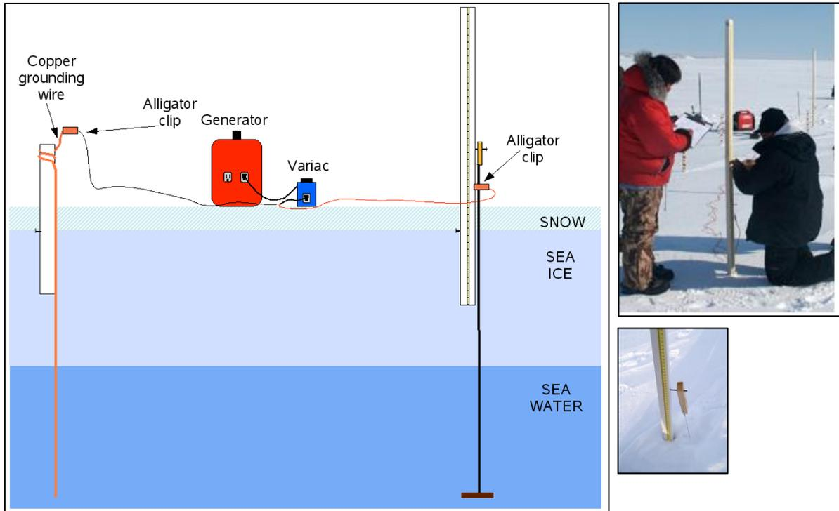
Figure 20 : Heating the Hotwire (from Mahoney and Gearheard)
