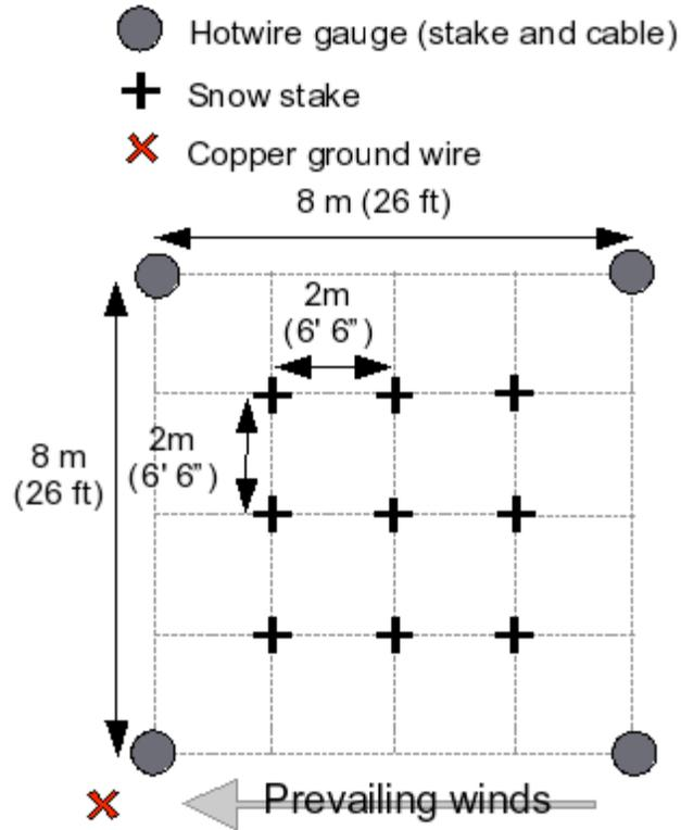
Figure 18 : Ice and snow measuring site (from Mahoney and Gearheard)
