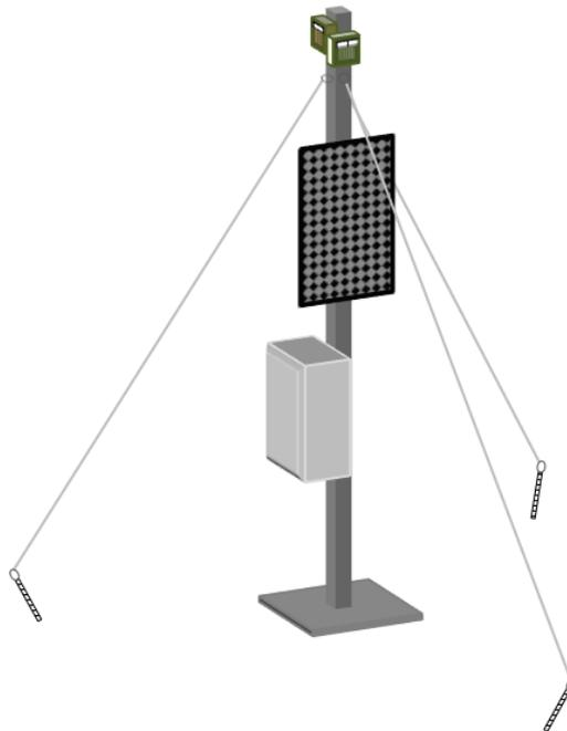
**Figure 13 : Supporting structure for the hunting type camera**
