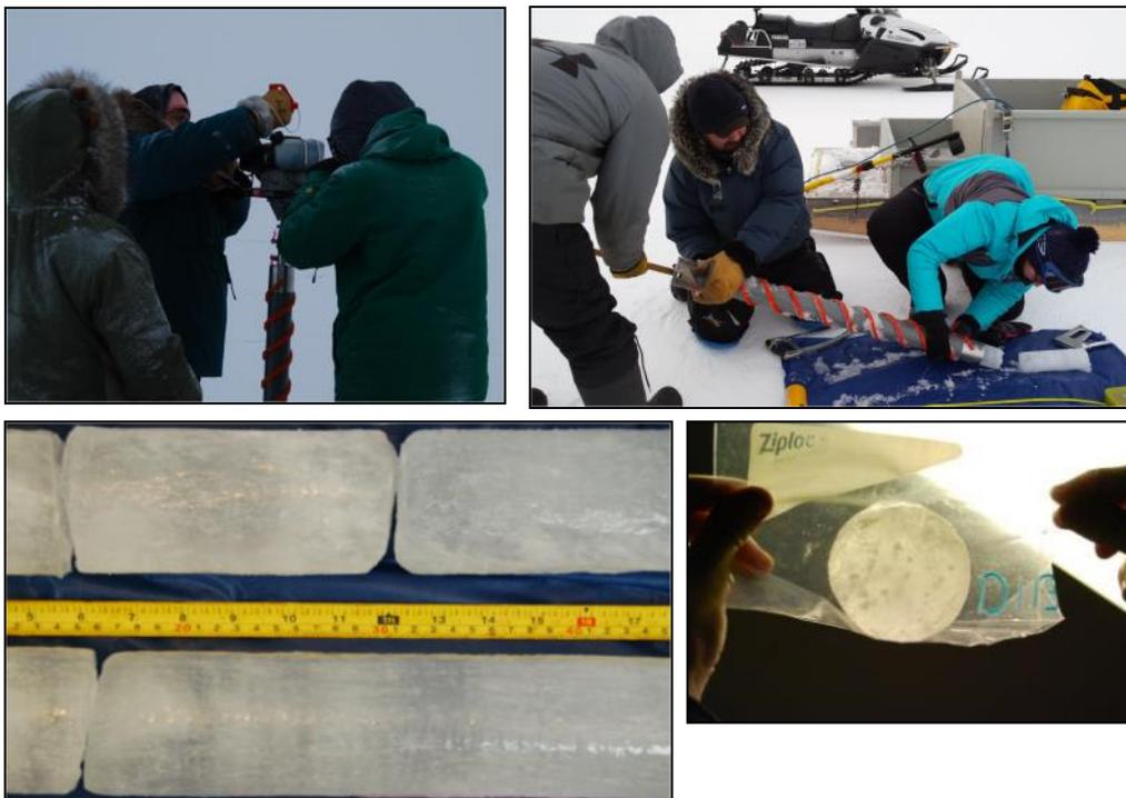
Figure 10 : Extracting ice cores
