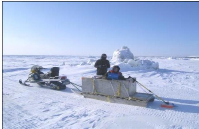
Figure 31: Use of a GPR for ice thickness measurements by INRS team (Koksoak River, 2008).
