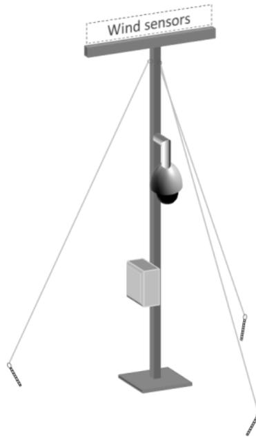
**Figure 12 : Supporting structure for the network camera**
