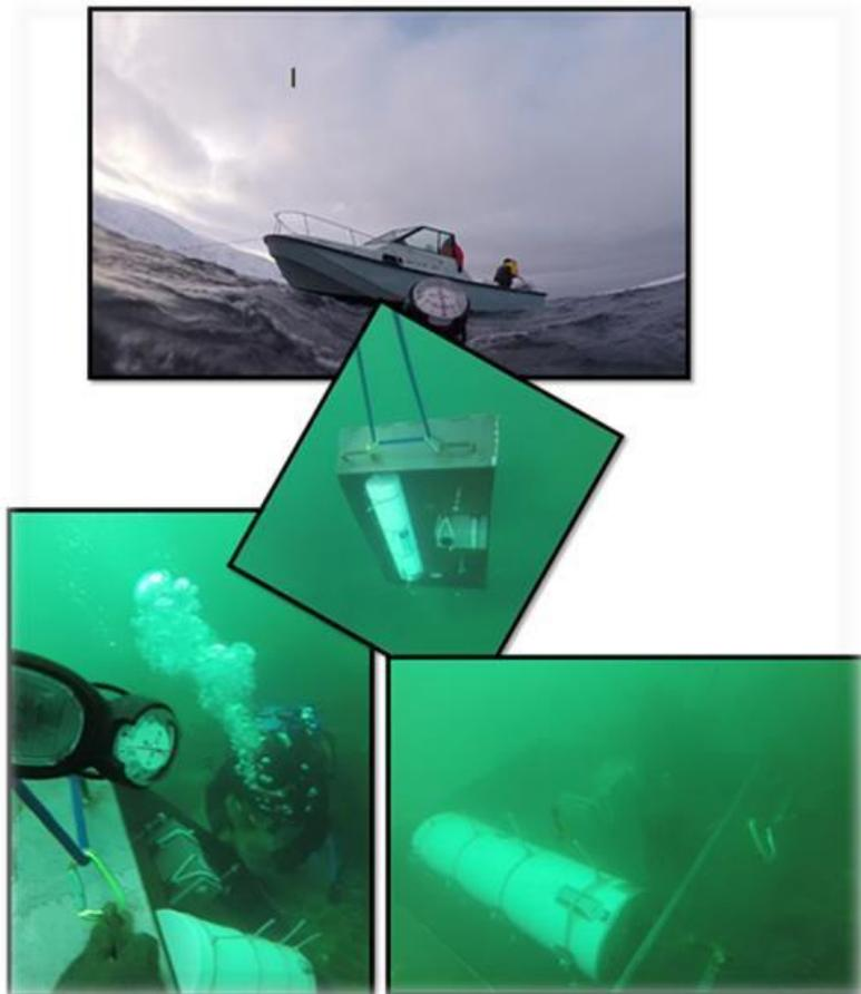
**Figure 24: Loading off the SWIP from the boat and divers installing it on the bottom of the bay**
