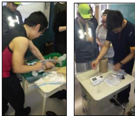
Figure 19 : Cutting samples from an ice core and measuring ice salinity in the classroom.
