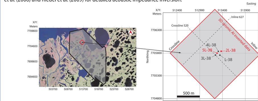
Figure 1: Disposition of the 3D seismic data and the wells 5L-38 and 2L-38 at Mallik.
