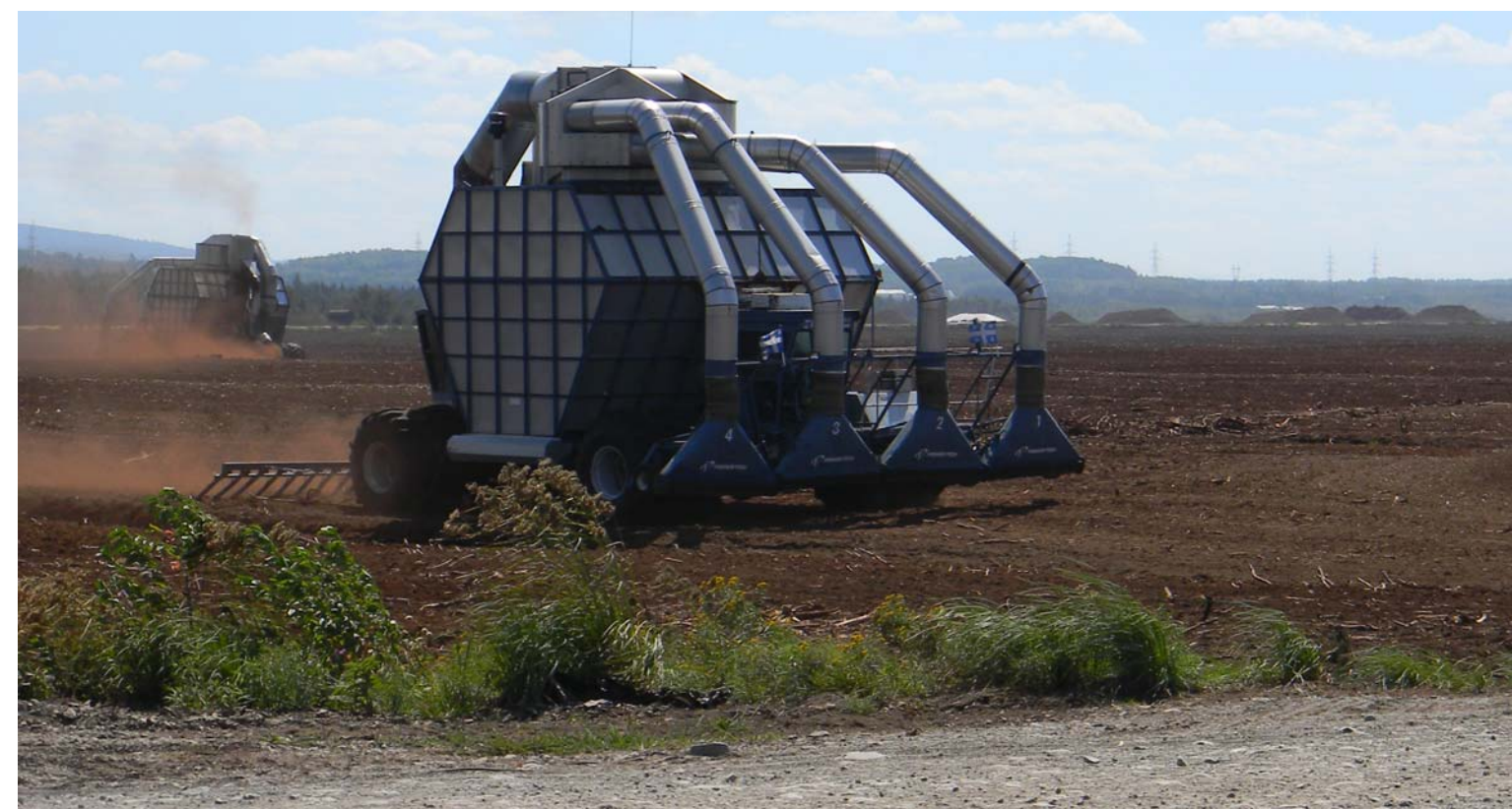
Figure 1. Tractor used to harvest peat by vacuuming
