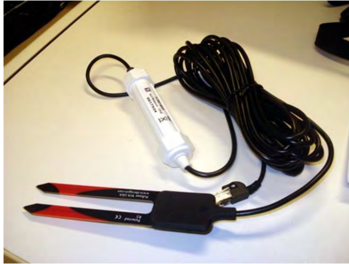
Figure 12. Frequency domain reflectometer (FDR sensor) Onset S-SMB-M005 with UTP connector cable.
