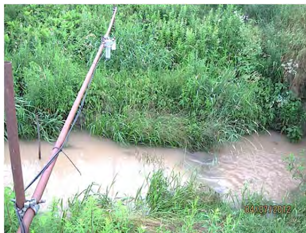
Figure 19. Ultrasonic module (module 710) used at the catchment outlet for measuring water height.
