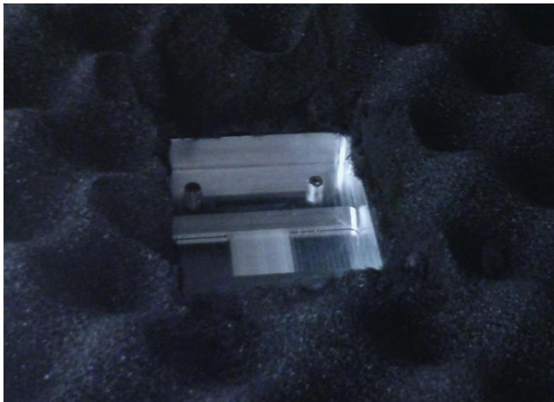
**Figure 98 Fixation holding the antenna, surrounded by absorber material**
