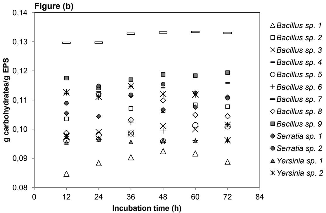
Figure 3.2.2 Protein Figure (a) and carbohydrate Figure (b) content present in the broth EPS synthesized by different bacterial strains in sterilized sludge at different incubation times
