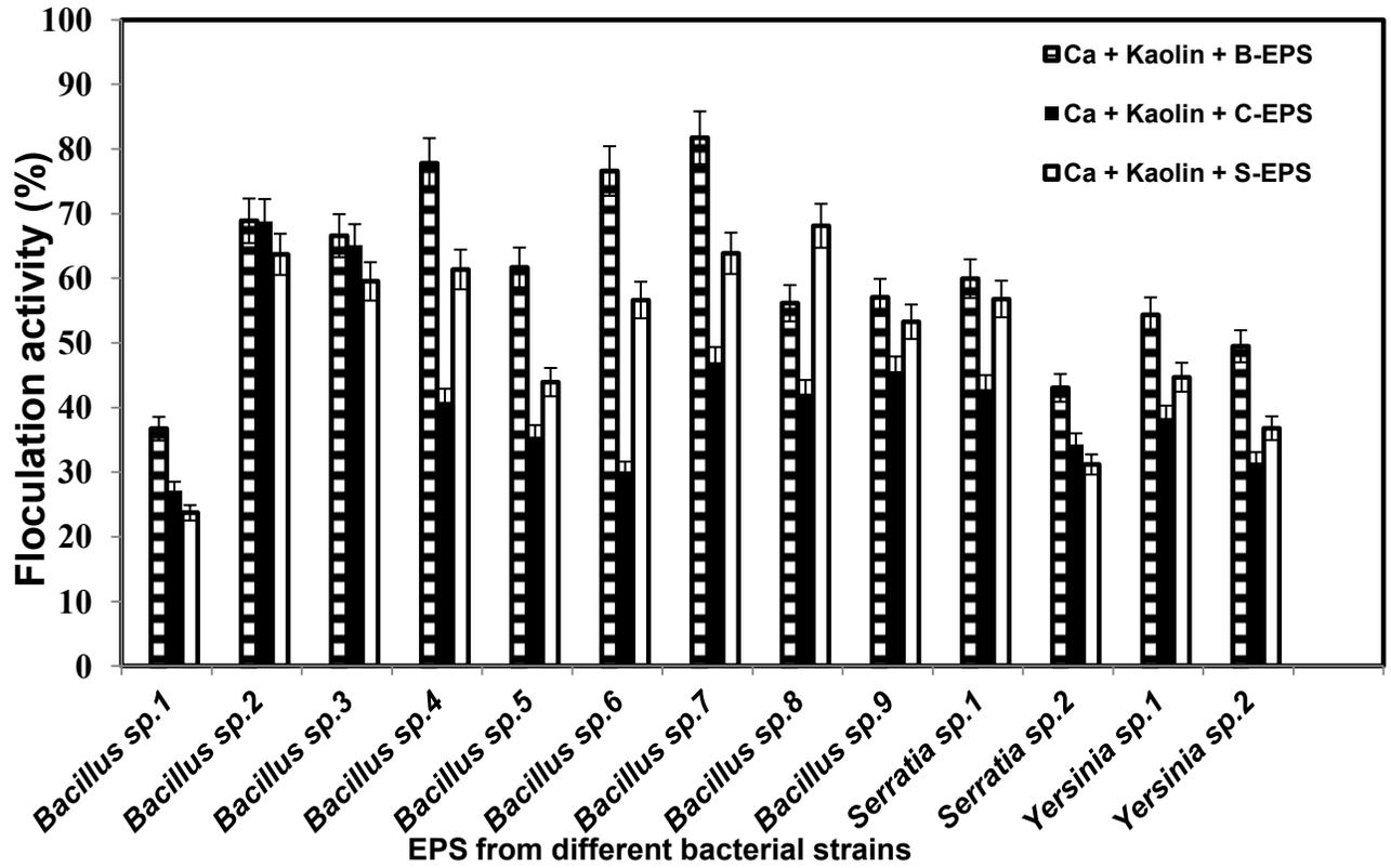
Figure 3.1.1 Variations in the kaolin flocculation activity due to addition of  $\text{Ca}^{2+}$  followed by different forms of the EPS produced in the sludge by different bacterial strains
