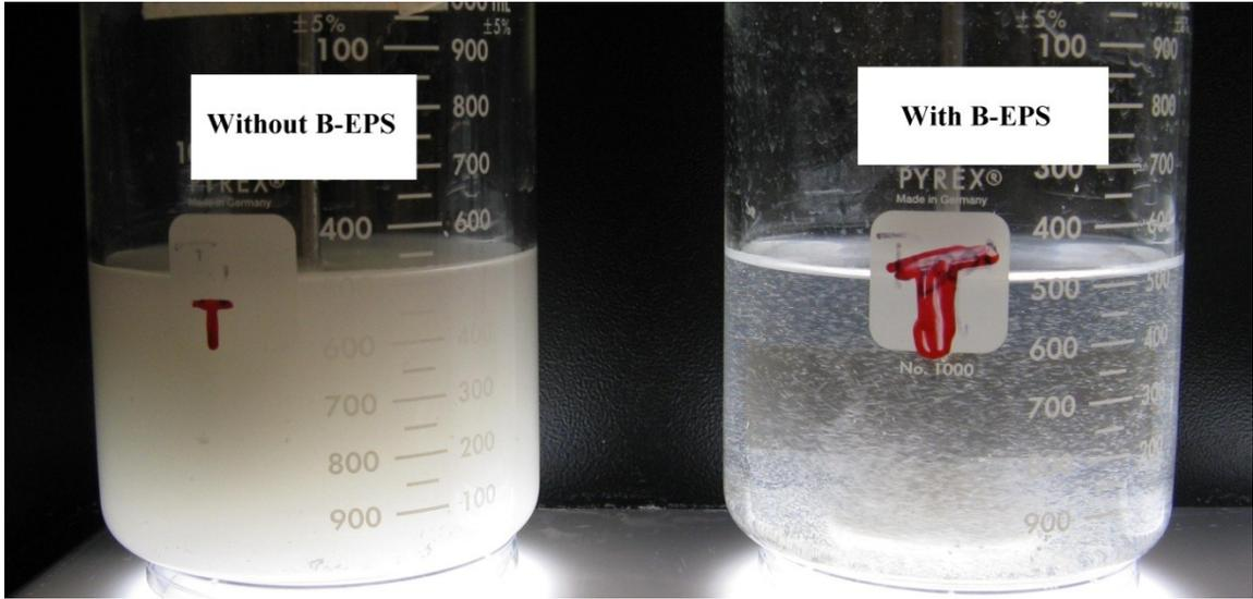
Figure 5.1.4 During Jar tests - kaolin suspension with and without addition of B-EPS (produced by mixed culture in sterilized sludge) combined with calcium
