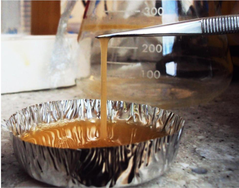
Figure 5.1.3 Viscous EPS produced by mixed culture in synthetic medium
