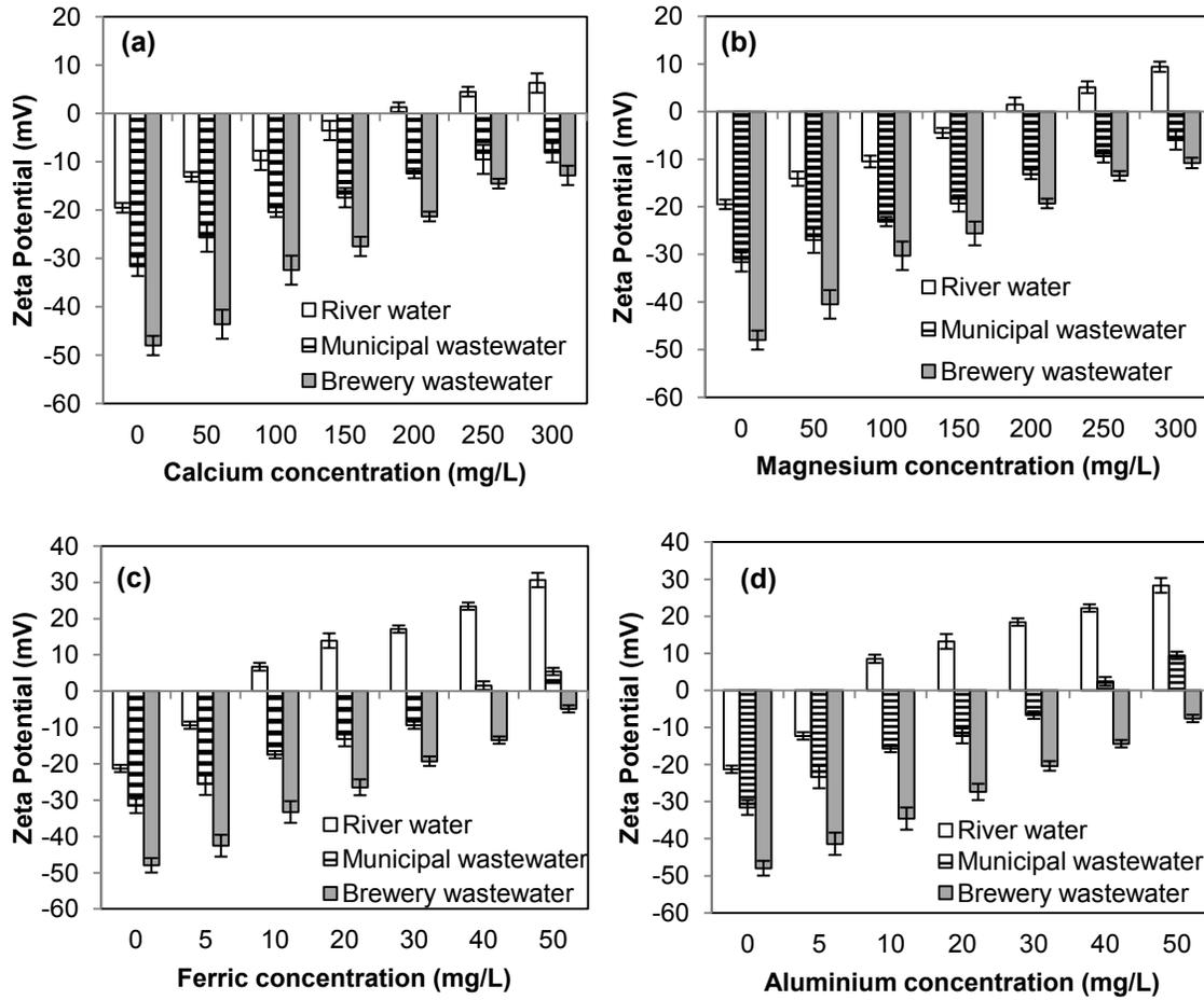
Figure 5.2.5 Zeta potential (mV) of river water, municipal and brewery wastewater at different cation concentrations respectively; a) Calcium ( $\text{Ca}^{2+}$ ), b) magnesium ( $\text{Mg}^{2+}$ ), c) Ferric ( $\text{Fe}^{3+}$ ) and d) Aluminum ( $\text{Al}^{3+}$ )
