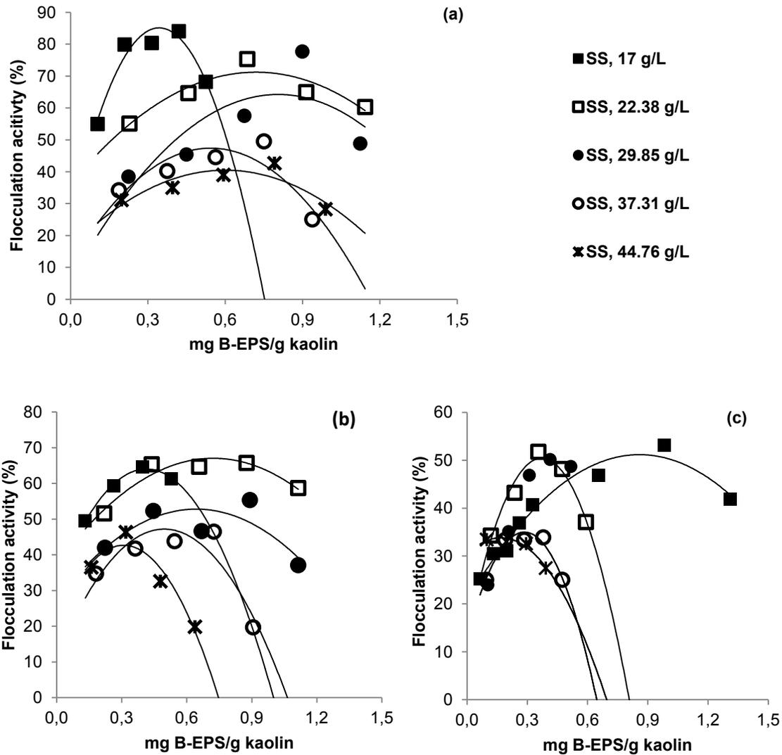
Figure A3.1: Flocculation activity of B-EPS produced in (a) sterilized sludge (b) alkaline-thermal treated sludge and (c) acid-thermal treated sludge at different sludge solids concentrations (SS: 17, 22.38, 29.85, 37.31 and 44.76 g/L).
