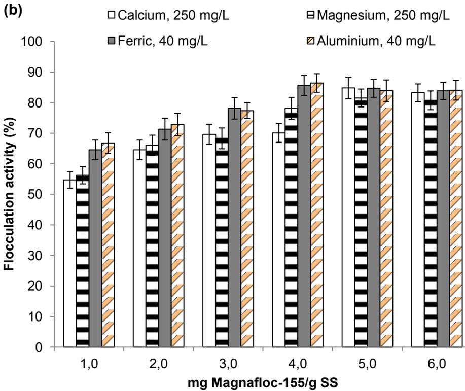
Figure 5.2.8 a) Effect of Broth EPS concentration (produced by mixed culture in sterilized sludge, 25 g/L) and different cations on brewery wastewater flocculation activity; b) Effect of Magnafloc-155 concentration and different cations on brewery wastewater flocculation activity
