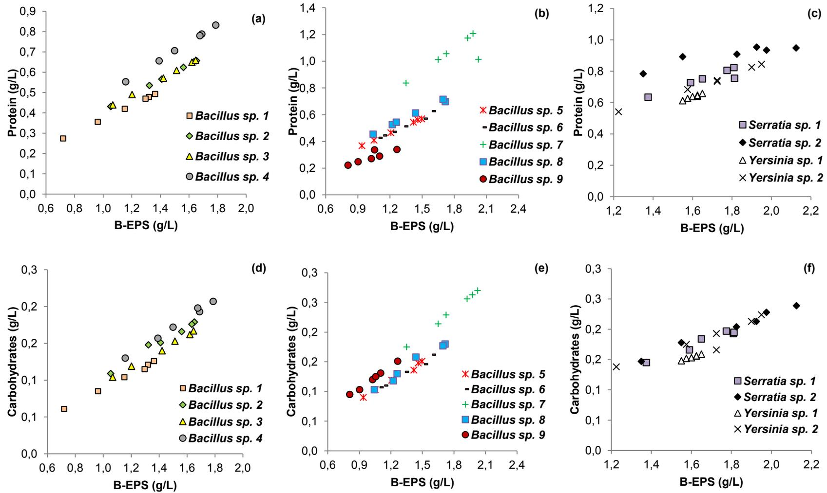
Figure A2.3: Proteins (a, b and c) and Carbohydrates (d, e and f) concentrations observed at different B-EPS concentrations for different bacterial strains.
