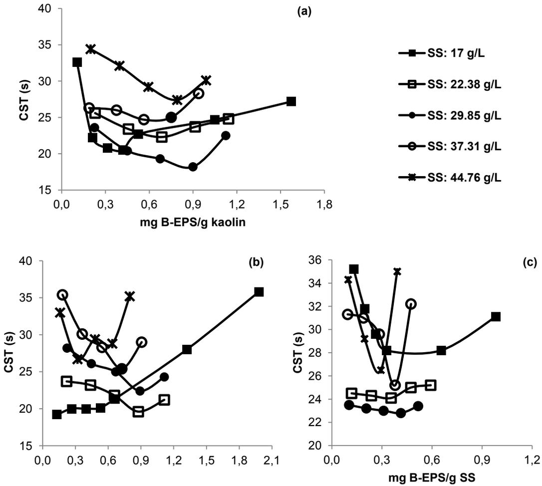
Figure A3.2: Change in CST of the B-EPS produced in (a) sterilized sludge, (b) alkaline-thermal treated sludge and (c) acid-thermal treated sludge at different sludge solids concentrations (SS, 17, 22.38, 29.85, 37.31 and 44.76 g/L).
