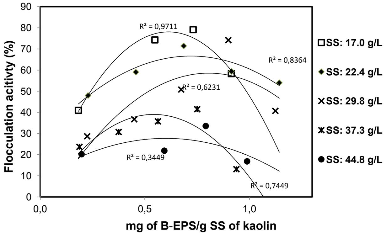
Figure 4.2 Variation in kaolin flocculation activity with different concentration of B-EPS (B-EPS produced in ST sludge at SS concentrations of 17.0, 22.4, 29.8, 37.3 and 44.8 g/L)
