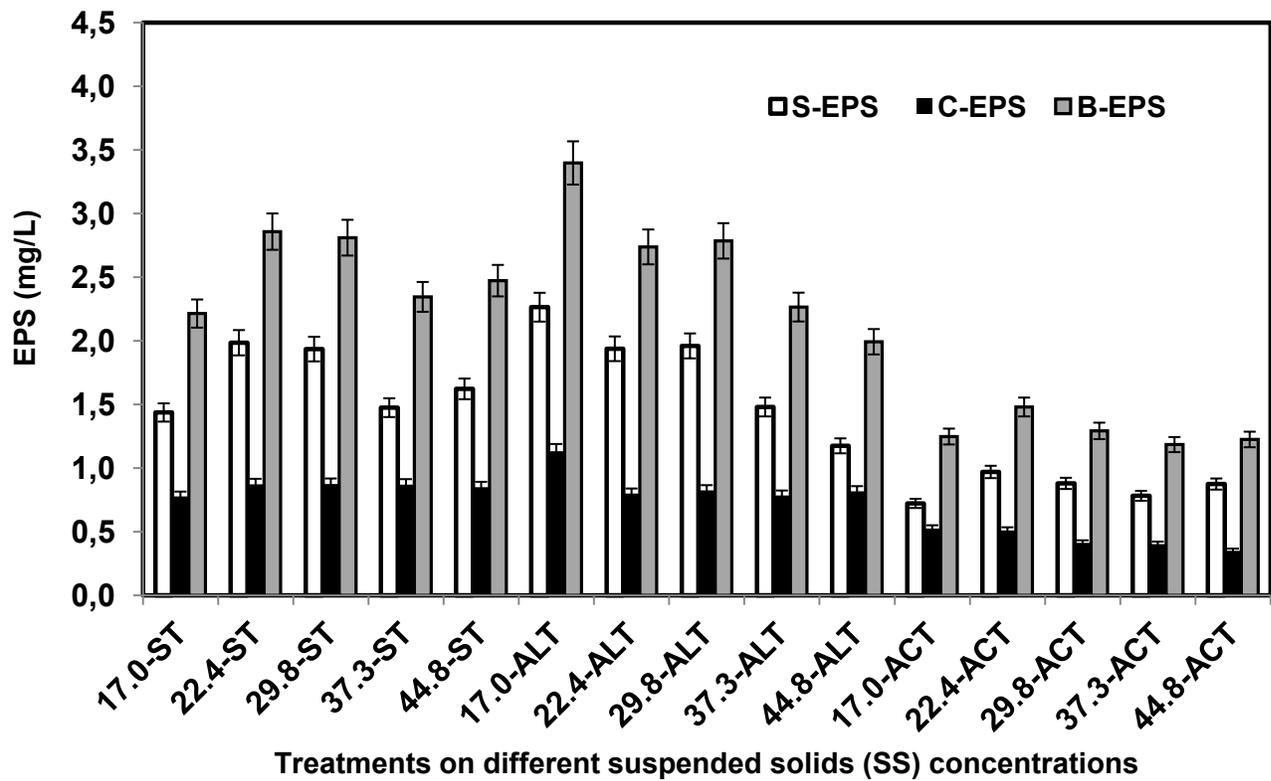
Figure 4.1 Production of EPS in treated (ST, ALT and ACT) sludge with different suspended solids concentration (SS: 17.0, 22.4, 29.8, 37.3 and 44.8 g/L)
