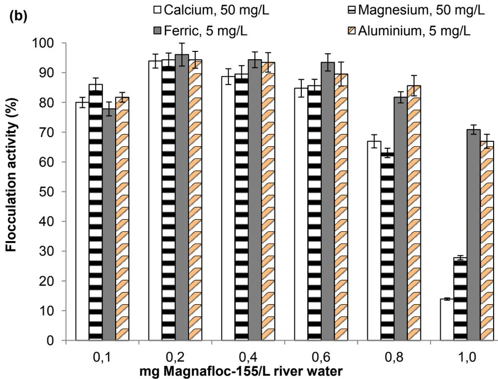
Figure 5.2.6 a) Effect of Broth EPS concentration (produced by mixed culture in sterilized sludge, 25 g/L) and different cations on river water flocculation activity; b) Effect of Magnafloc-155 and different cations on river water flocculation activity.
