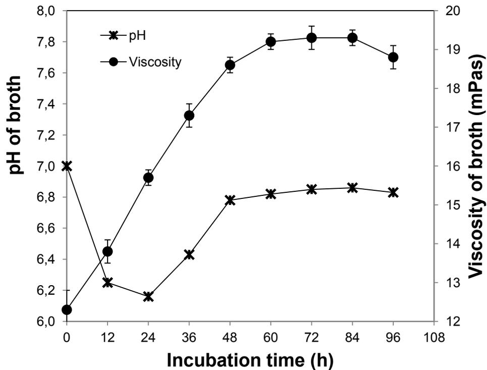
Figure 5.1.2 The pH and viscosity of the broth measured at different incubation time during growth of mixed culture in sterilized sludge
