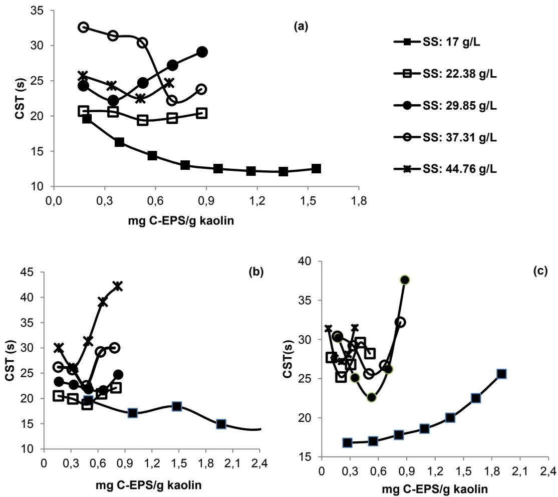
Figure A3.4: Change in CST of the B-EPS produced in (a) sterilized sludge, (b) alkaline-thermal treated sludge and (c) acid-thermal treated sludge at different sludge solids concentrations (SS, 17, 22.38, 29.85, 37.31 and 44.76 g/L).
