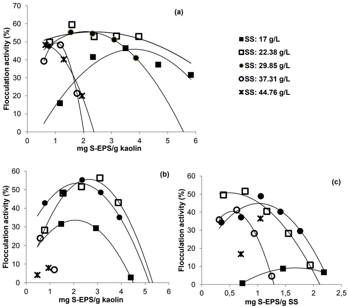
Figure A3.5: Flocculation activity of the S-EPS produced in (a) sterilized sludge, (b) alkaline-thermal treated sludge and (c) acid-thermal treated sludge at different sludge solids concentrations (SS, 17, 22.38, 29.85, 37.31 and 44.76 g/L).
