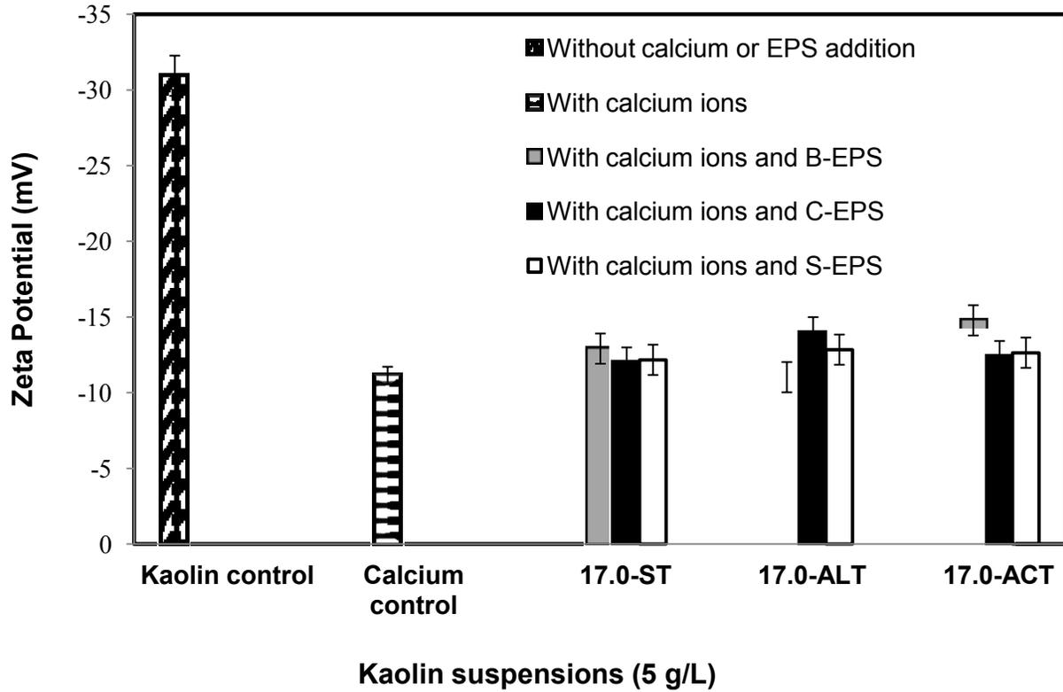
**Figure 4.4** Zeta potential of the kaolin suspension (kaolin control and calcium control) and kaolin suspension (combined with calcium) with the addition of different EPS types (B-EPS, C-EPS and S-EPS) produced with different treatments (ST, ALT and ACT) at SS concentration of 17.0 g/L. (Note: Zeta potential of the B-EPS, C-EPS and S-EPS was  $-28.9 \pm 0.3$  mV,  $-30.2 \pm 0.4$  mV and  $-27.7 \pm 0.9$  mV, respectively)
