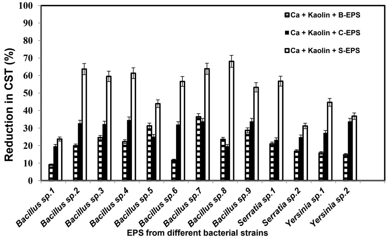
Figure 3.1.2 Reduction in the CST values of the kaolin suspension due to addition of  $\text{Ca}^{2+}$  followed by different forms of the EPS produced in the sludge using different bacterial strains
