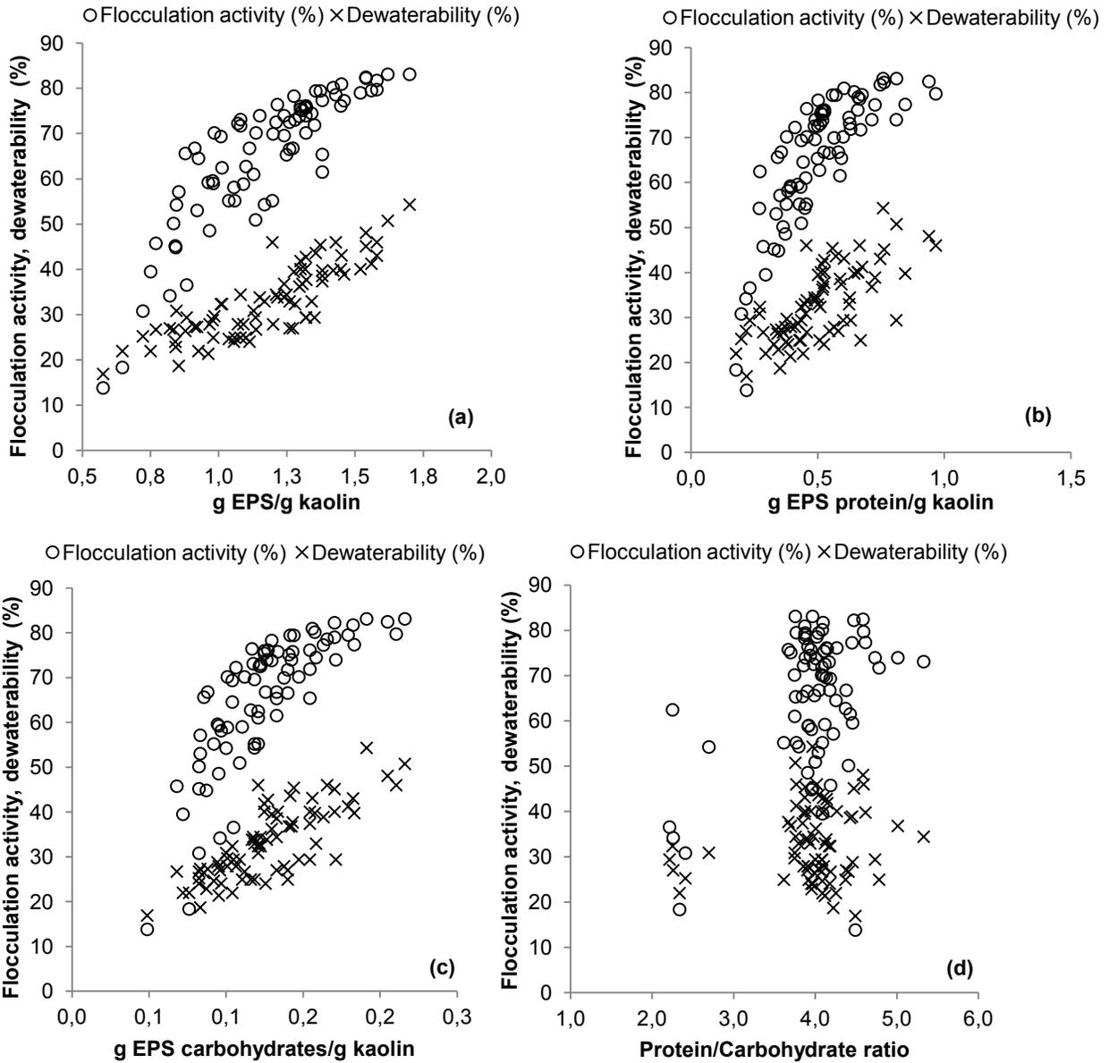
Figure A2.5: Flocculation activity and dewaterability (%) observed for (a) g EPS/g kaolin, (b) g EPS protein/g kaolin, (c) g EPS carbohydrates/g kaolin, (d) protein/carbohydrates, irrespective of the bacterial strains.
