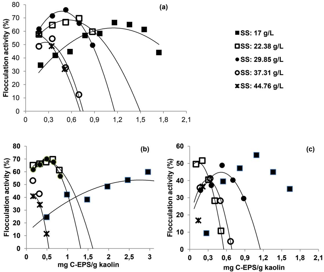
Figure A3.3: Flocculation activity of the B-EPS produced in (a) sterilized sludge, (b) alkaline-thermal treated sludge and (c) acid-thermal treated sludge at different sludge solids concentrations (SS: 17, 22.38, 29.85, 37.31 and 44.76 g/L).
