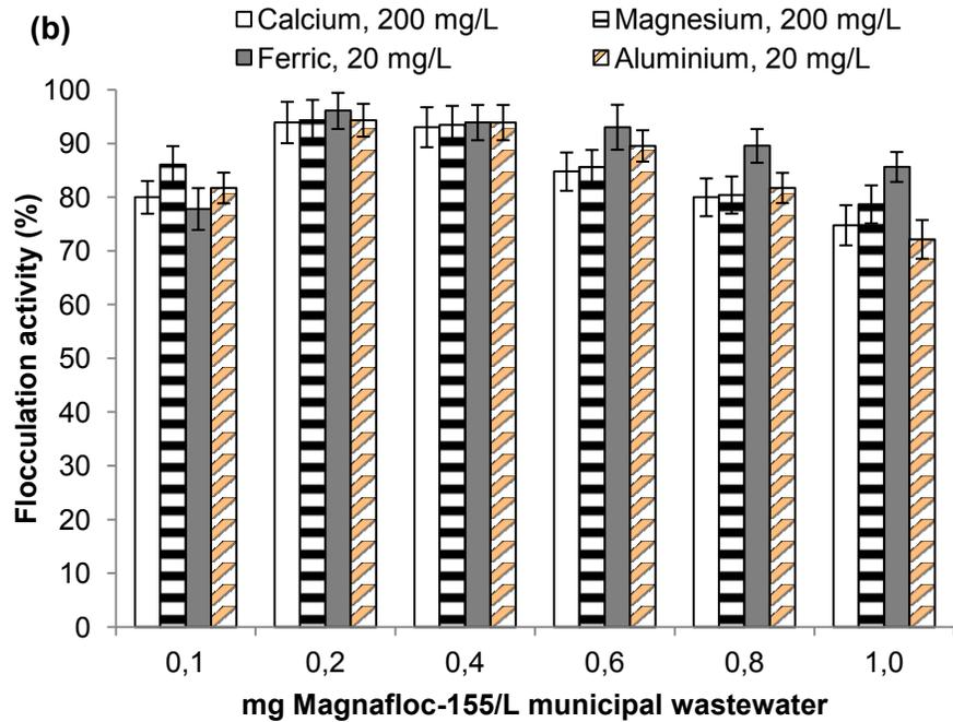
**Figure 5.2.7 a) Effect of Broth EPS concentration (produced by mixed culture in sterilized sludge, 25 g/L) and different cations on municipal wastewater flocculation activity; b) Effect of Magnafloc-155 and different cations on municipal wastewater flocculation activity**
