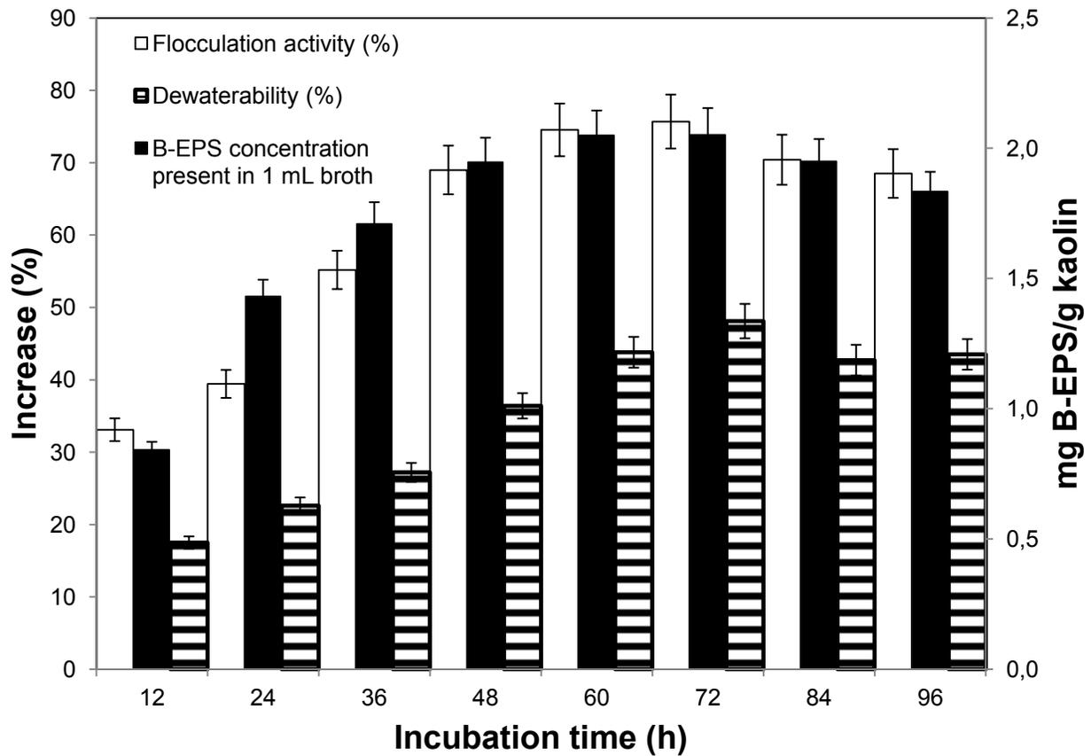
Figure 5.1.6 Variation in kaolin flocculation activity and dewaterability using B-EPS (1 mL broth) sampled at different incubation time during growth of mixed culture in sterilized sludge
