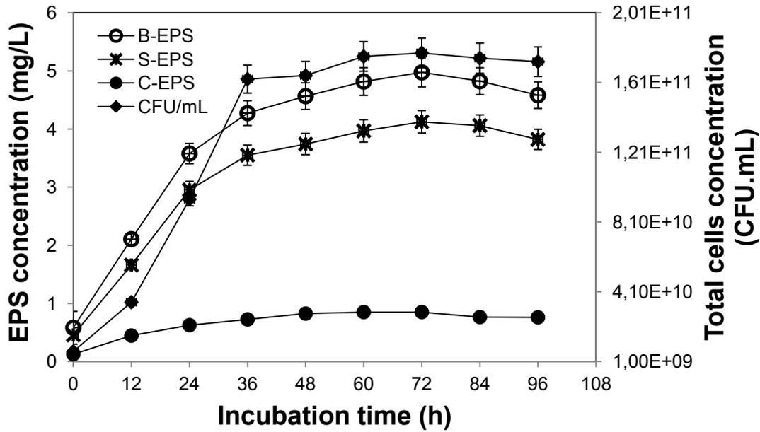
Figure 5.1.1 Variation of EPS concentrations (B-EPS, S-EPS, and C-EPS) and total cells concentrations (CFU/mL) during mixed culture growth (of 13 bacterial strains) in sterilized sludge
