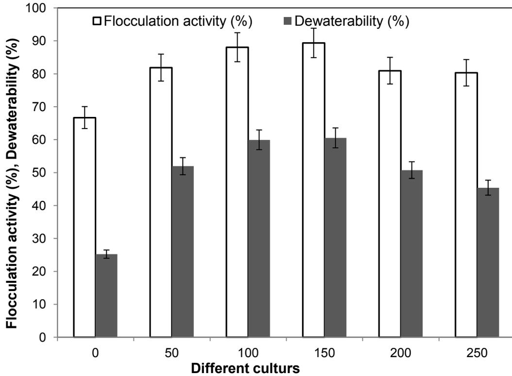
Figure 5.2.2 Kaolin flocculation activity and dewaterability of B-EPS (1 mL) produced by the mixed culture at 72 h of incubation
