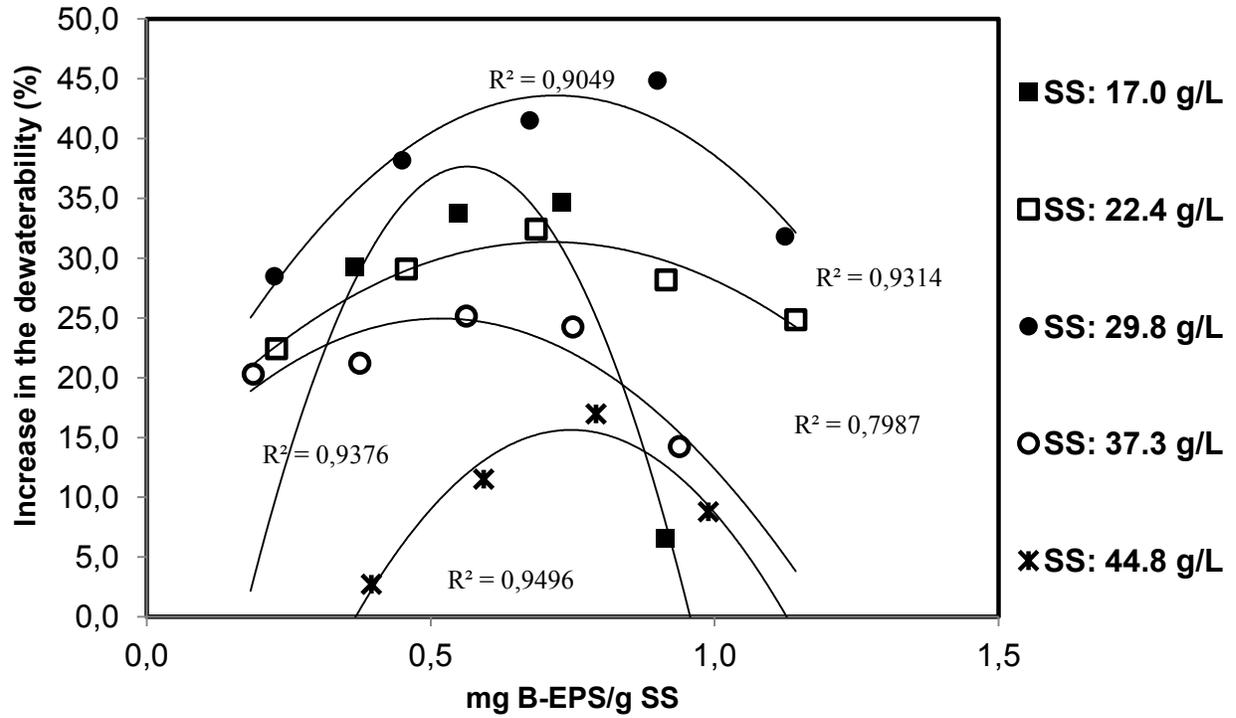
Figure 4.3 Variation of dewaterability (%) of the kaolin suspension with different concentration of B-EPS (B-EPS produced in ST sludge at SS concentrations of 17.0, 22.4, 29.8, 37.3 and 44.8 g/L)
