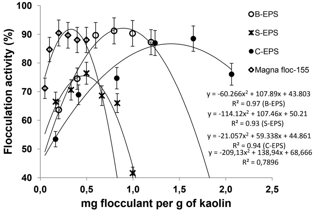
Figure 5.1.7 Effect of various flocculants (B-EPS, S-EPS, C-EPS and Magnafloc-155) concentration on kaolin flocculation activity
