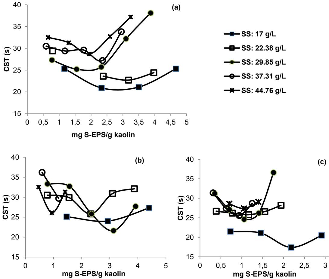
Figure A3.6: Change in CST of the B-EPS produced in (a) sterilized sludge, (b) alkaline-thermal treated sludge and (c) acid-thermal treated sludge at different sludge solids concentrations (SS, 17, 22.38, 29.85, 37.31 and 44.76 g/L).
