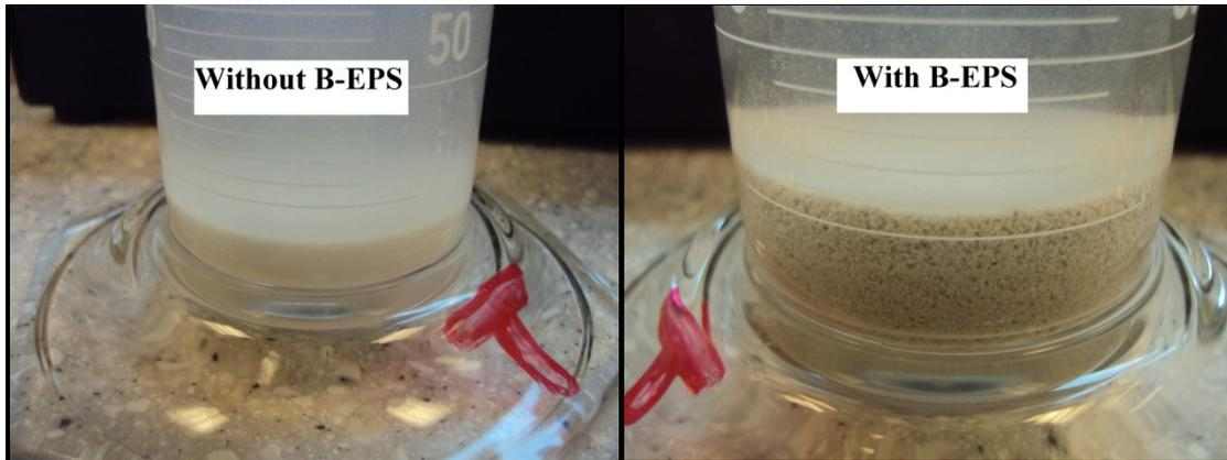
Figure 5.1.5 After jar tests - kaolin floccs with and without addition of B-EPS (produced by mixed culture in sterilized sludge) combined with calcium
