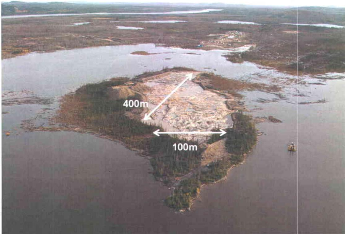
**Figure 8.1.2:** Bird's eye view of the large stripped outcrop that exhibits the core of Roberto's auriferous system. Photo courtesy of Peter Lauder (Opinaca Mines Ltd.).
