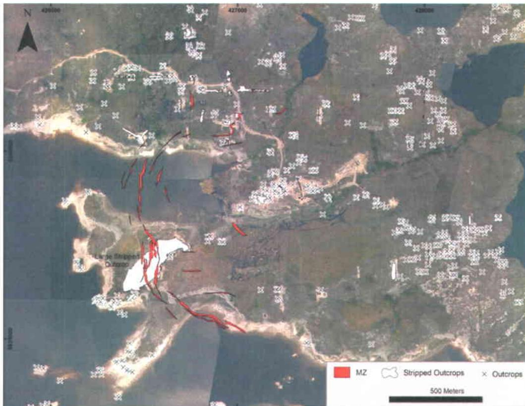
Figure 8.1.1: Map showing available outcrop exposures and localization of Roberto's auriferous zones. Aerial photograph in background courtesy of Opinaca Mines Ltd. Coordinates are in UTM Nad83.
