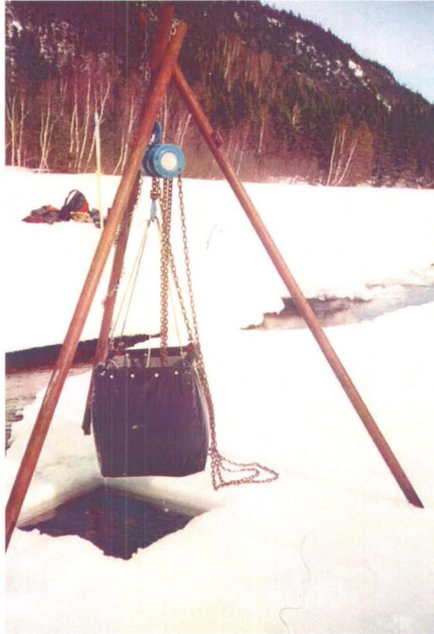
Figure 5.3 Infiltration cube extracted during the late winter period.
