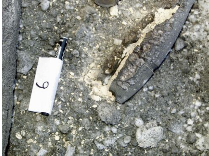
Figure 28. Projectile impacted by fragments from a mortar detonation 15 cm away (trial #6)
