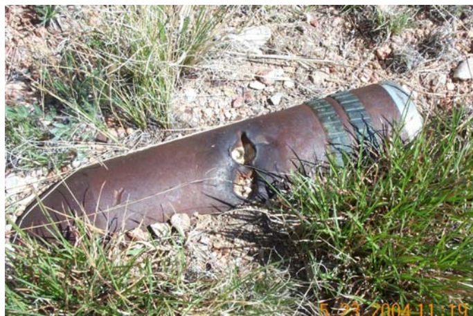
Figure 30. UXO found in impact area of Ft. Carson, CO showing similar damage pattern as in Fig. 28 (Photo courtesy of Alan Hewitt, CRREL)
