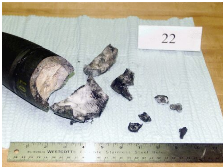
Figure 27. Cracked shell produced by 63.2 g C4 placed on the nose (trial # 22)
