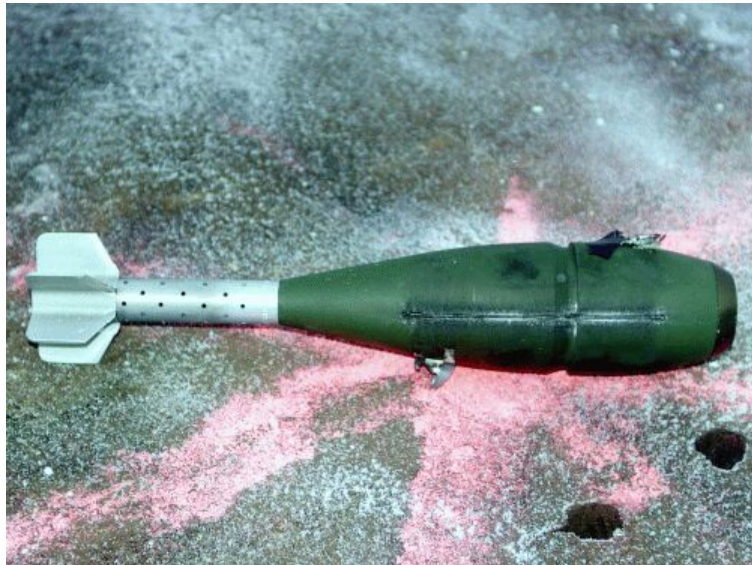
Figure 26. Effect of a 16.3 g C4 shaped charge with 5.7 g initiating C4 ball on projectile casing (trial #2)
