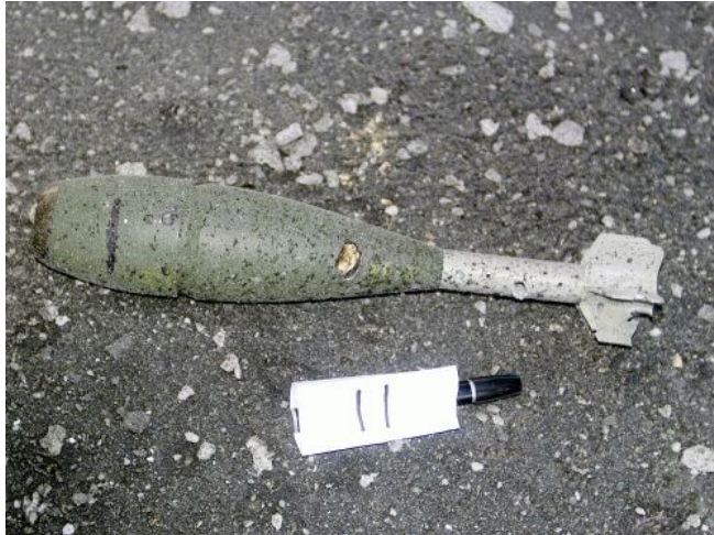
Figure 7: Projectile attacked by fragments at a long distance (trial # 11)
