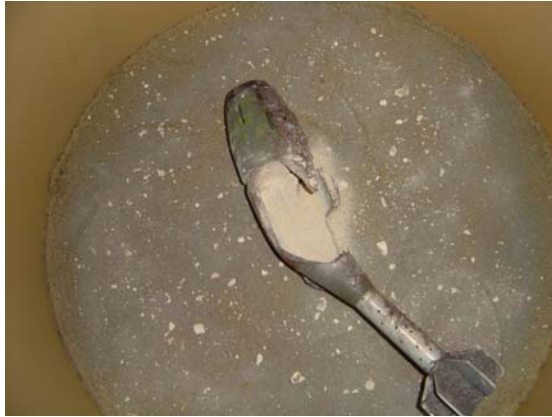
Figure 22. Column D surface prior of experiment Mortar with detonation residue
