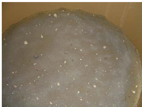
Figure 20. Column B surface prior to start of experiment Detonation residue
