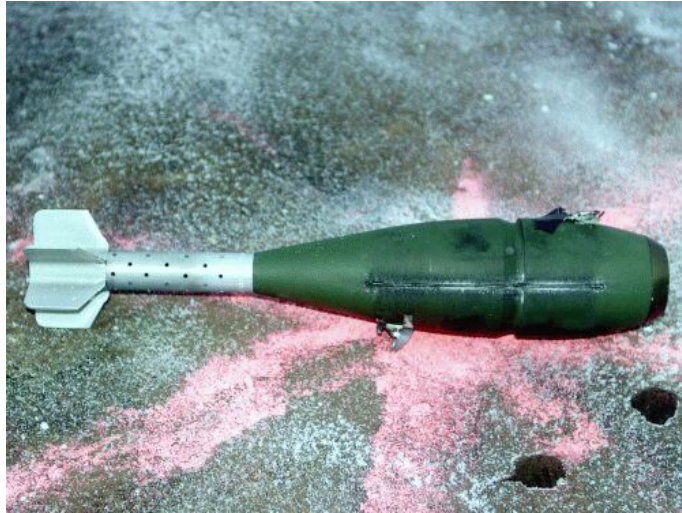
Figure 4: Effect of a shaped charge, showing groove blasted into projectile casing (trial #2)
