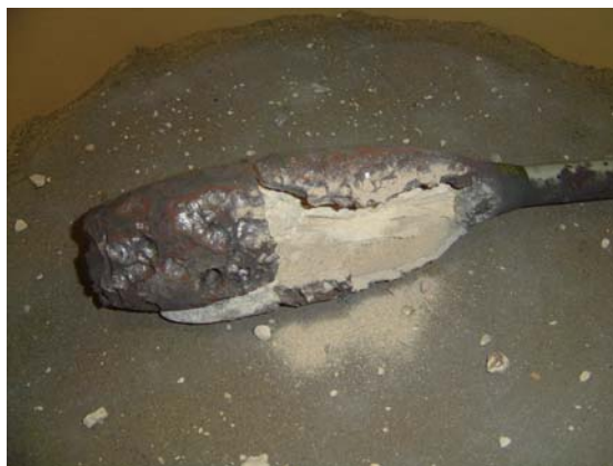
Figure 24. Column F surface prior to start of experiment Mortar with detonation residue
