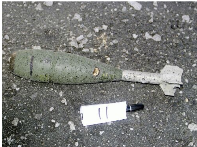
Figure 29. Projectile impacted by fragments from a mortar detonation 157 cm away (trial # 11)
