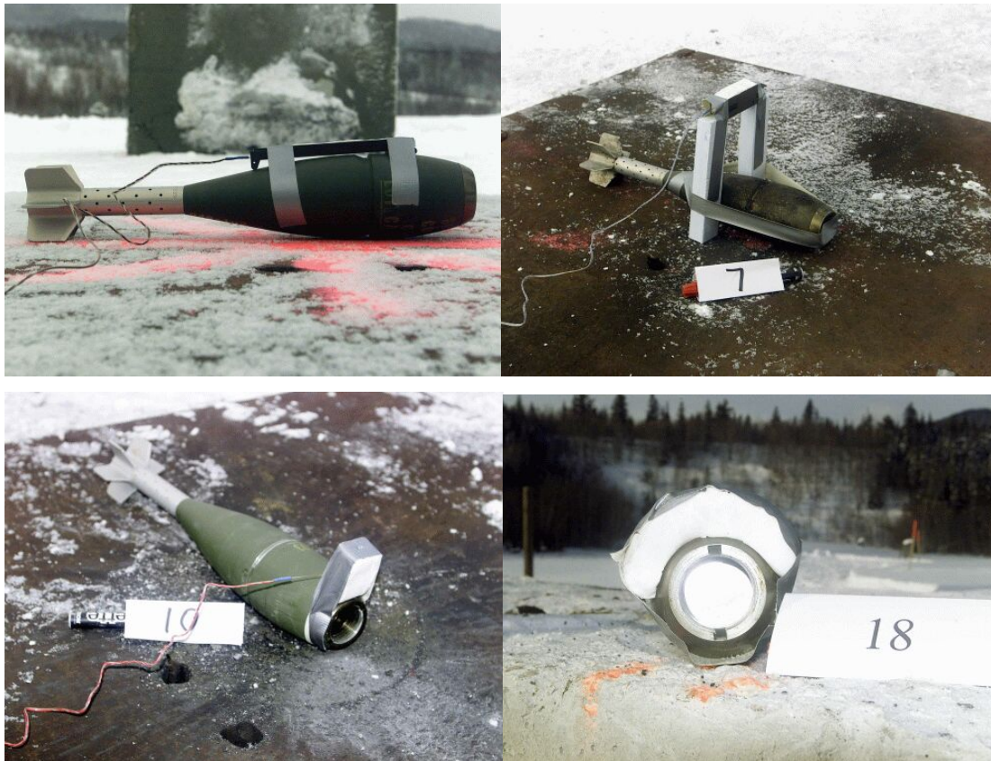
Figure 1: Configurations used in Method 1. Top left: small shaped charge longitudinal, minimal stand-off. Top right: larger shaped charge, large stand-off. Bottom left: Small block of C4 at the nose. Bottom right: Hemispherical configuration of C4 at the nose.
