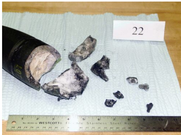
Figure 5: Cracked shell produced by C4 on the nose (trial # 22)
