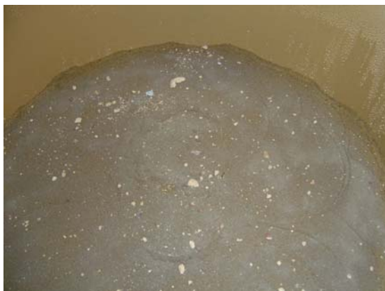
Figure 21. Column C surface prior to start of experiment Detonation residue
