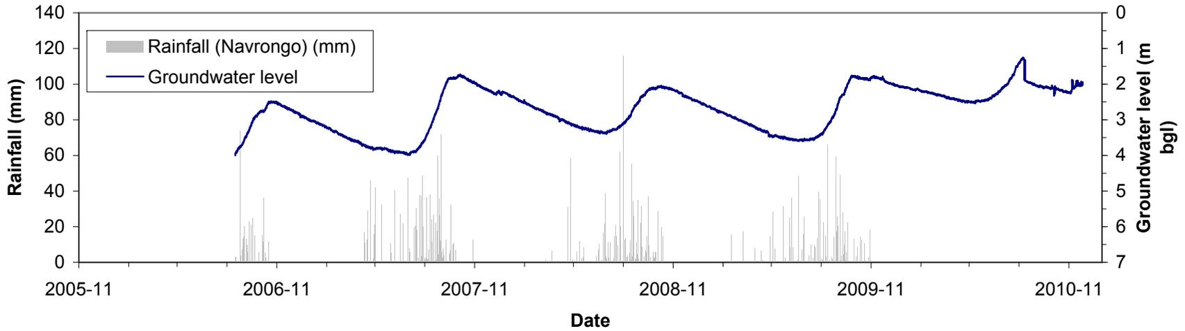
**Groundwater level-time plot from Ducie monitoring well (WVB 09)**
