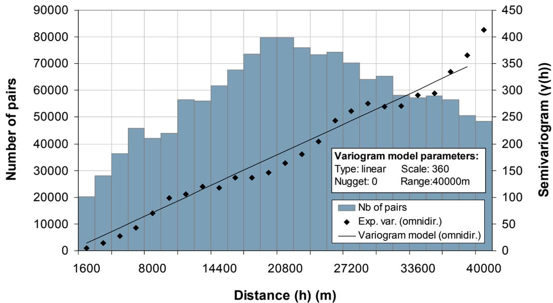
Figure 5-13 – Experimental and model variograms for kriging of groundwater levels with well and river water levels (Tamne basin)
