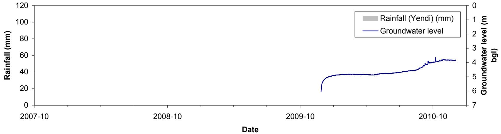
**Groundwater level-time plot from Tantuya monitoring well (HAP 21)**
