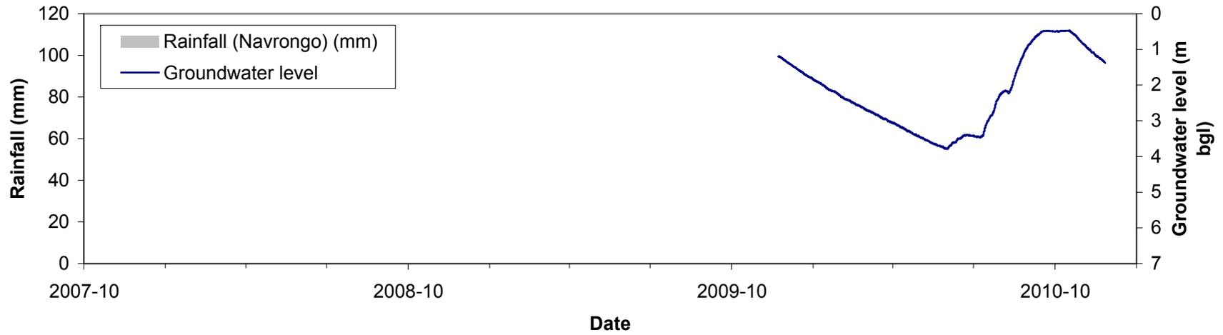
**Groundwater level-time plot from Tuuni monitoring well (HAP 14)**
