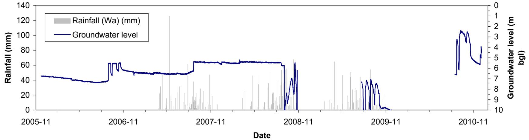
Groundwater level-time plot from Tinguri monitoring well (WVB 12)
