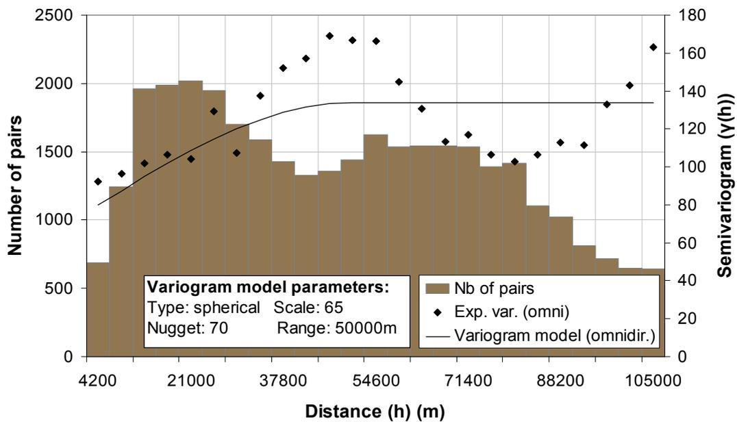
Figure 5-7 – Experimental and model variograms for kriging of regolith thickness (Voltaian sedimentary basin)
