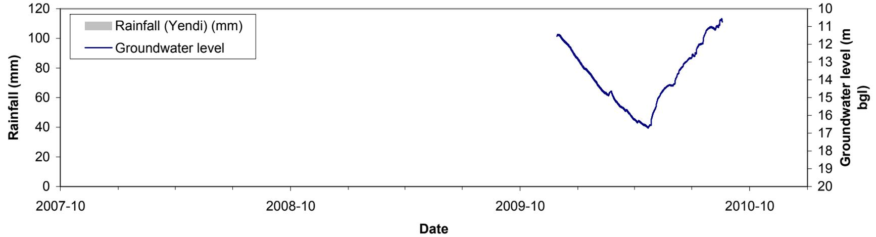
**Groundwater level-time plot from Nawuni monitoring well (HAP 19)**
