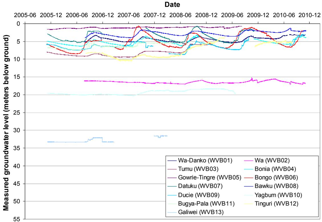
Figure 4-5 – Groundwater level fluctuations for the new monitoring wells
