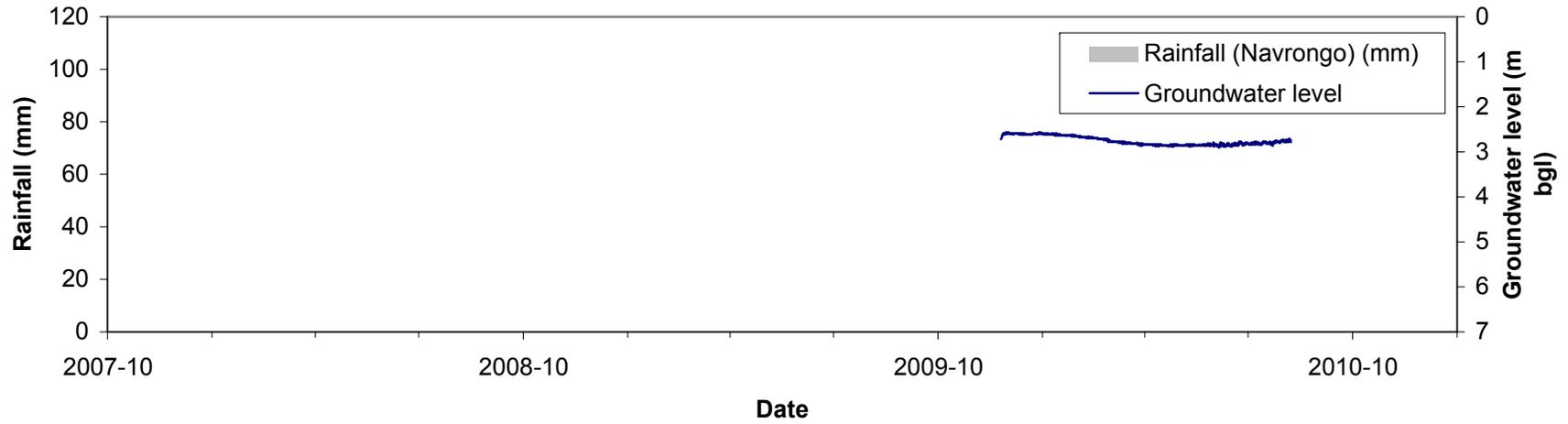
**Groundwater level-time plot from Lentinkpa monitoring well (HAP 15)**
