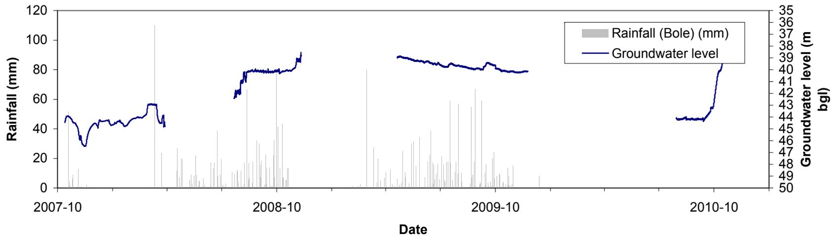
**Groundwater level-time plot from Kanshegu monitoring well (HAP 04)**
