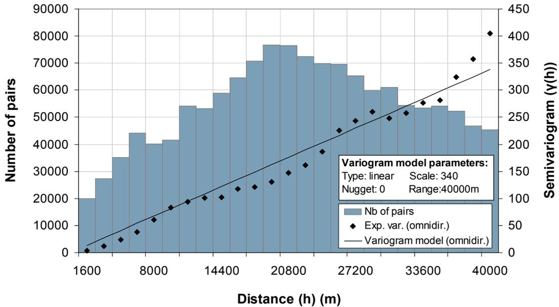
Figure 5-11 – Experimental and model variograms for kriging of groundwater levels with river data (Tamne basin)
