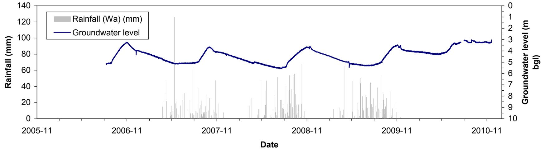
**Groundwater level-time plot from Wa monitoring well (WVB 02)**
