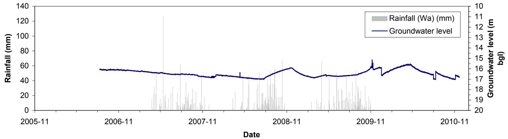
**Groundwater level-time plot from Tumu monitoring well (WVB 03)**
