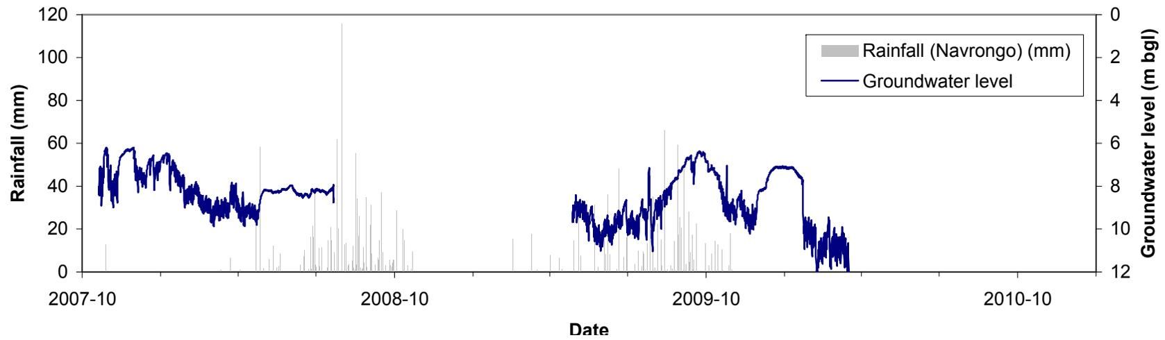
**Groundwater level-time plot from Nakpeuk monitoring well (HAP 12)**
