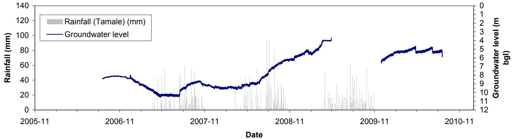
Groundwater level-time plot from Galiwei monitoring well (WVB 13)
