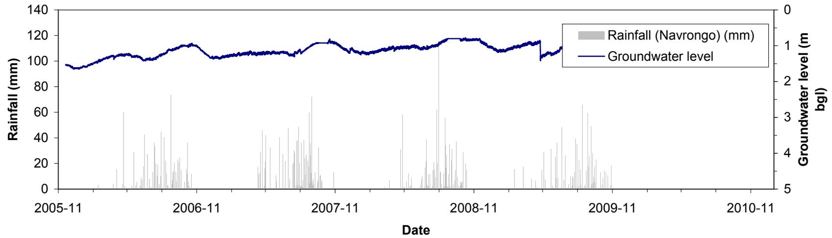
**Groundwater level-time plot from Bongo-Nayire monitoring well (WVB 06)**
