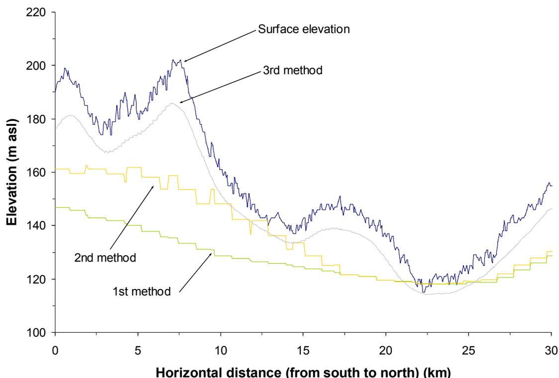
Figure 5-19 – Cross sections with estimated potentiometric surfaces (Tamne basin)
