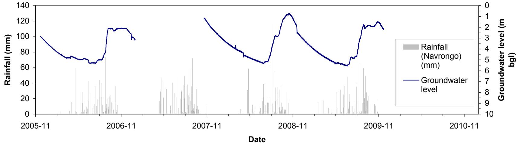
**Groundwater level-time plot from Bawku monitoring well (WVB 08)**
