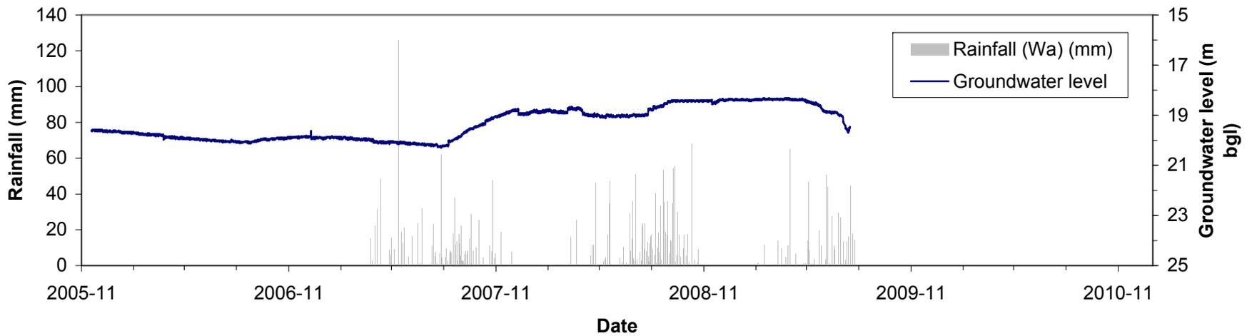
Groundwater level-time plot from Bugya-Pala monitoring well (WVB 11)
