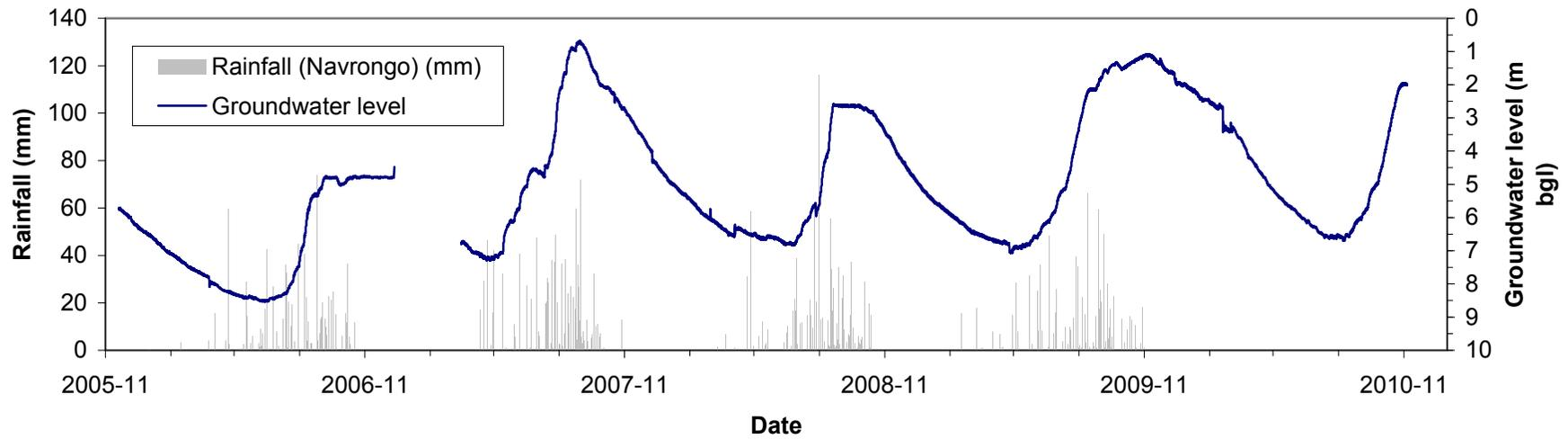
**Groundwater level-time plot from Datuku monitoring well (WVB 07)**
