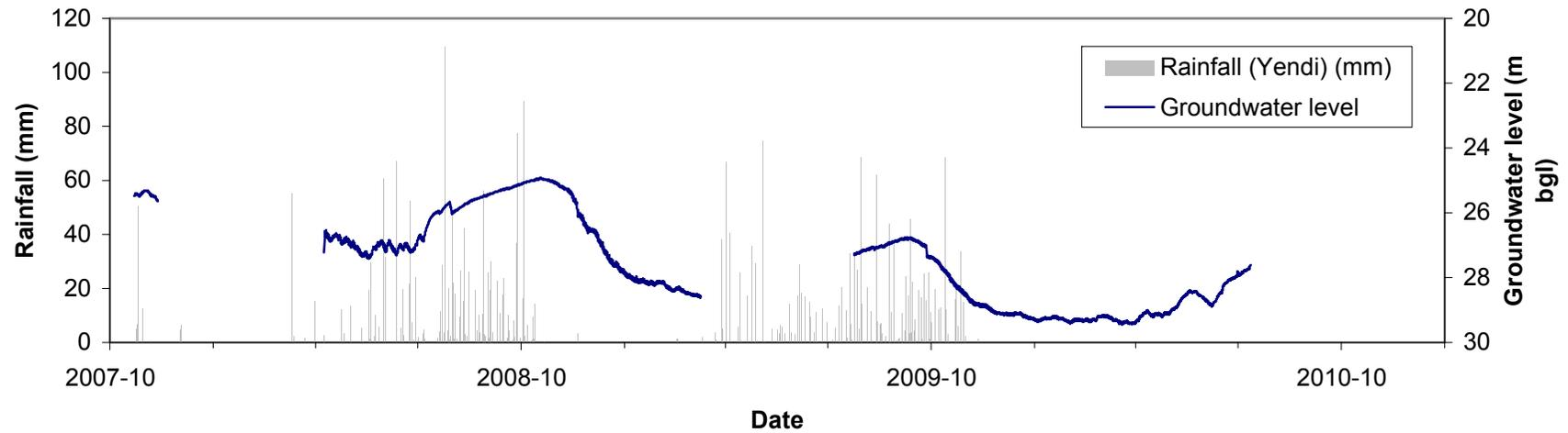
**Groundwater level-time plot from Tachecku monitoring well (HAP 10)**
