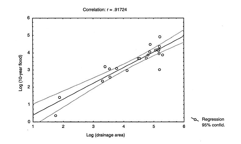
Figure 4. Regression between ten year flood discharge (F10) and drainage area (from El Jabi et al. 1994)
