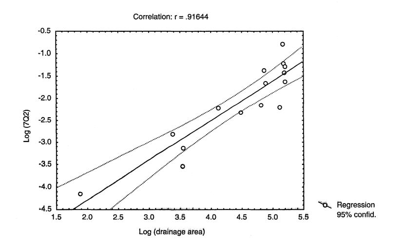
Figure 11. Regression between 10 year low flows with a seven-day duration (7Q10) and drainage areas (from El Jabi et al. 1994)
