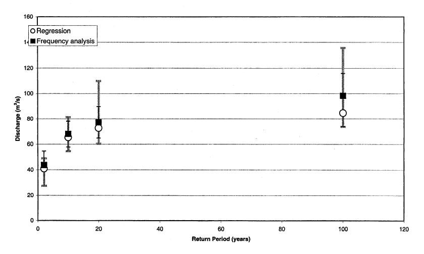
Figure 13. Comparison between flood quantiles evaluated by frequency analysis and by regression at station 01BS001 (Coal Branch at Beersveille). Lower and upper confidence intervals are represented by a dashed line for the regression results and by a full line for the frequency analysis.
