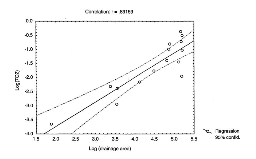
Figure 10. Regression between two year low flows with a seven-day duration (7Q2) and drainage areas (from El Jabi et al. 1994)
