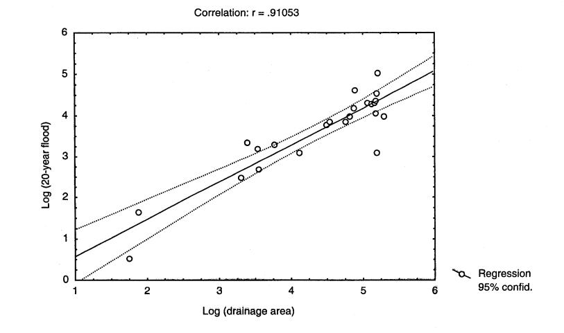
Figure 5. Regression between 20 year flood discharge (F20) and drainage area (from El Jabi et al. 1994)
