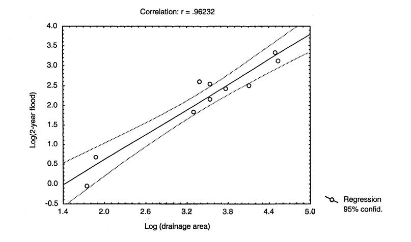
Figure 3. Regression between two year flood discharge (F2) and drainage area (from El Jabi et al. 1994)
