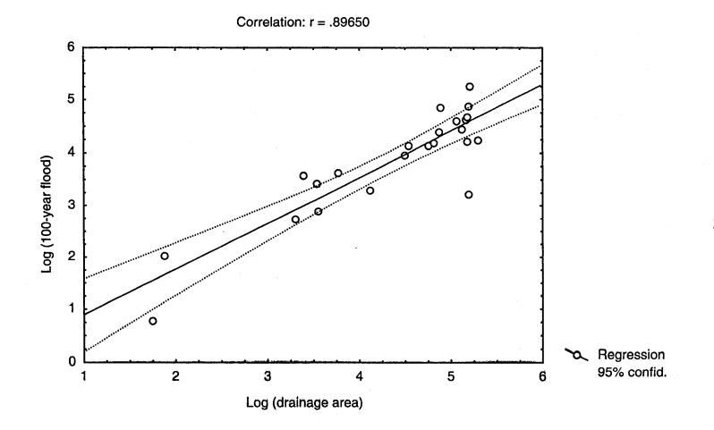
Figure 6. Regression between 100 year flood discharge (F100) and drainage area (from El Jabi et al. 1994)
