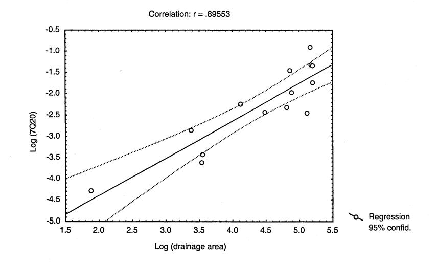
Figure 12. Regression between 20 year low flows with a seven-day duration (7Q20) and drainage areas (from El Jabi et al. 1994)
