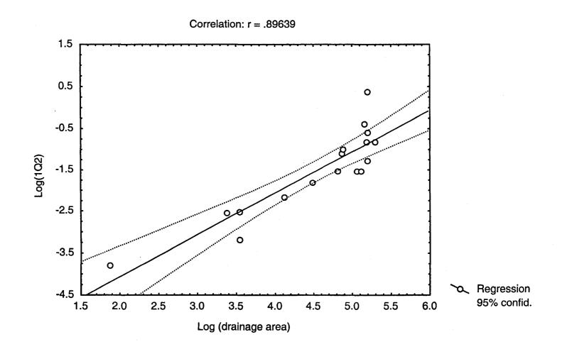
Figure 7. Regression between two year low flow with a one-day duration (1Q2) and drainage area (from El Jabi et al. 1994)
