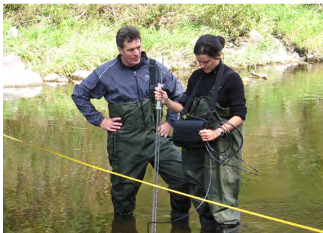
André Saint-Hilaire and Anik Daigle, Rouge stream temperature and flow measurements, Beauport, Quebec
