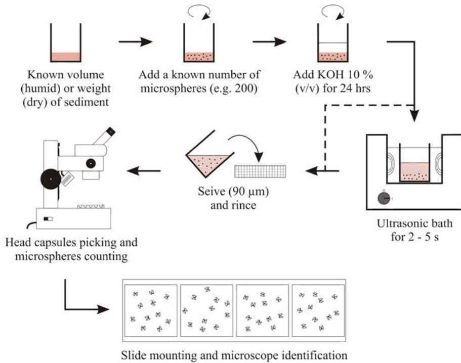
*Figure 3.3. Sample preparation with microspheres*
