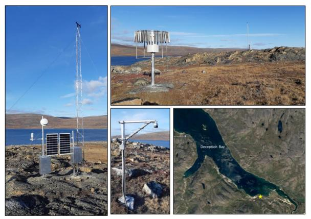
Figure 8 : Weather station installed in Deception Bay (Bombardier beach)
