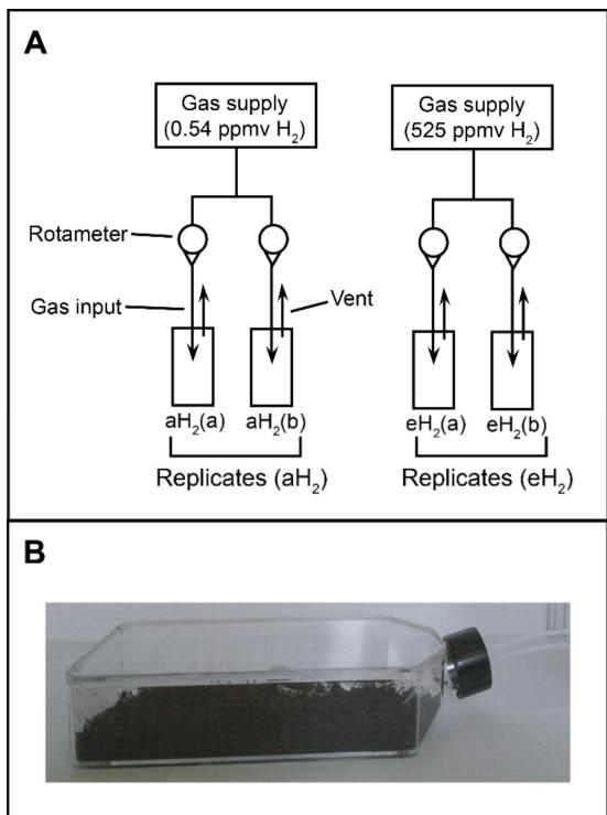
**Figure 3.7** Schematic representation of the dynamic microcosm chambers. (A) Schematic representation of the dynamic microcosm chambers utilized in this study to expose soil to aH<sub>2</sub> or eH<sub>2</sub> levels. (B) Photograph of one soil microcosm.
