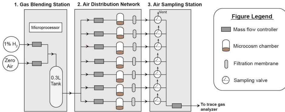
**Figure 4.7 Schematic of the dynamic microcosm chamber unit setup**
