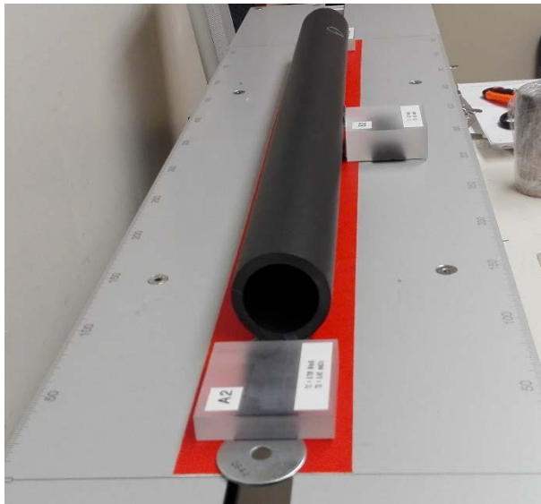
Pipe sample during a thermal conductivity measurement
