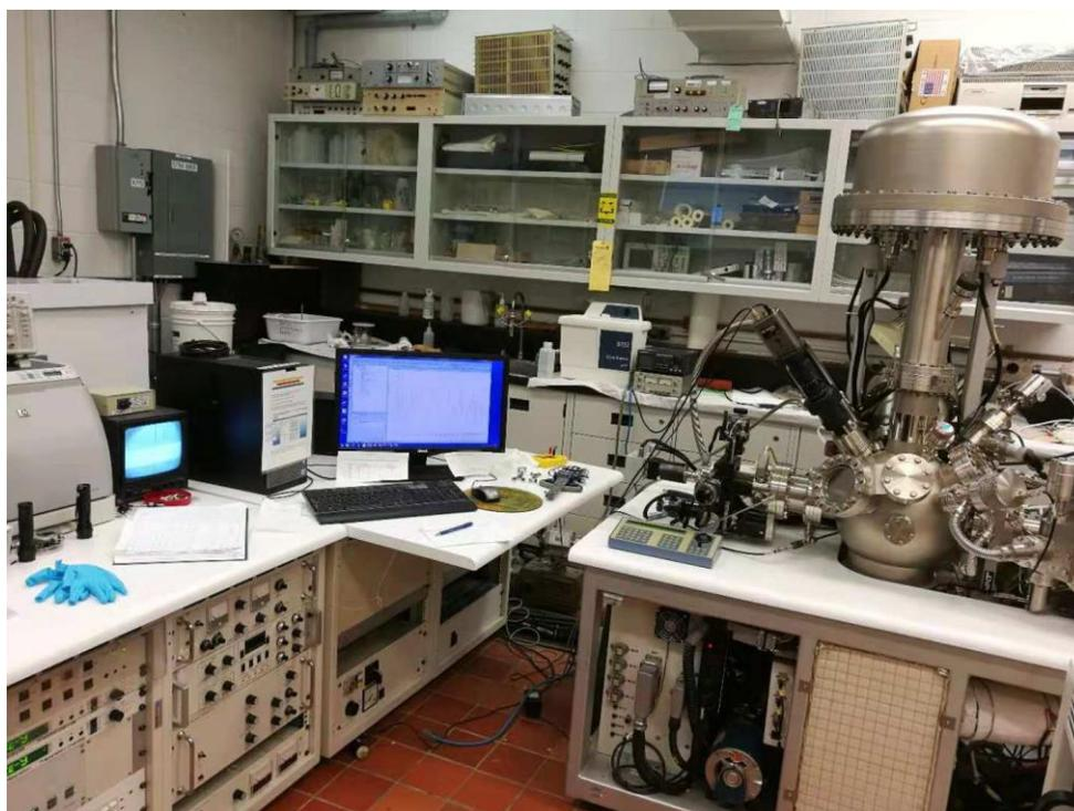
**Figure 2.3** The XPS equipment at INRS-EMT.
