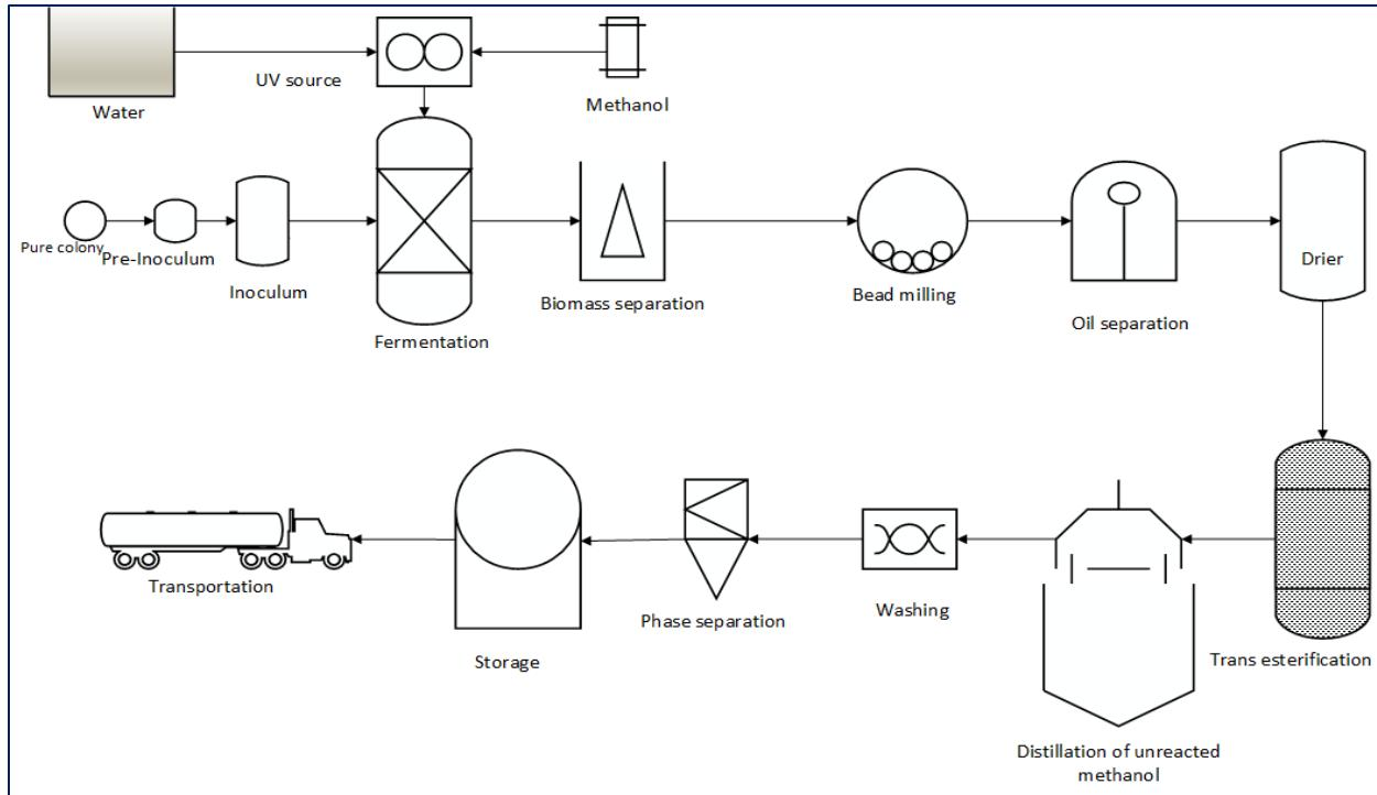
Figure 36 The flow diagram of lipid and biomass production on UV treated tap water with methanol supplementation
