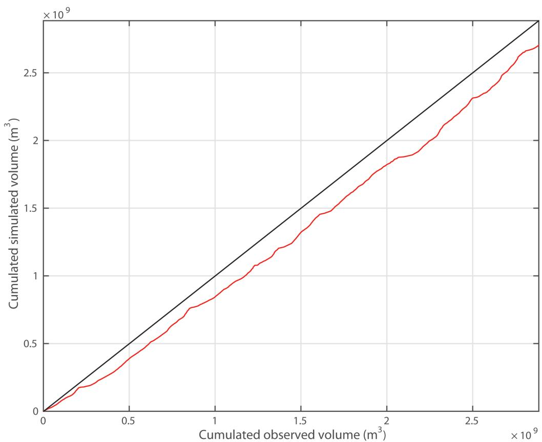
Figure 4.17. Cumulated simulated volume versus observed volume during the calibration period.
