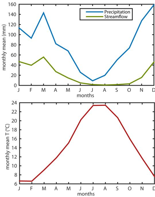
Figure 2.6. Mean monthly precipitation (P), discharge (Q), and temperature (T) for the Flumendosa basin during the period 1926-1937.
