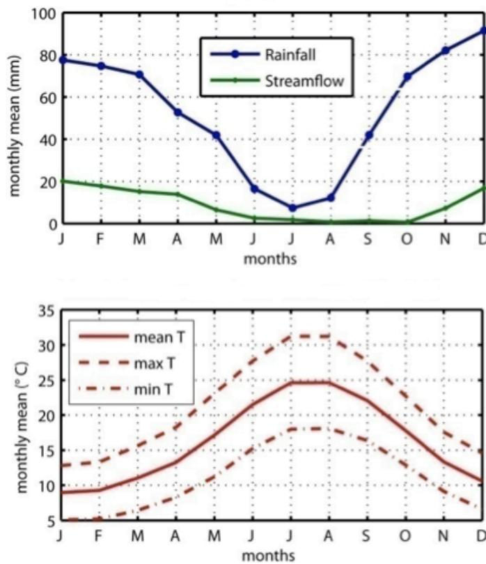
Figure 2.2. Mean monthly precipitation discharge and temperature in Rio Mannu catchment computed in different periods in which daily data were available.
