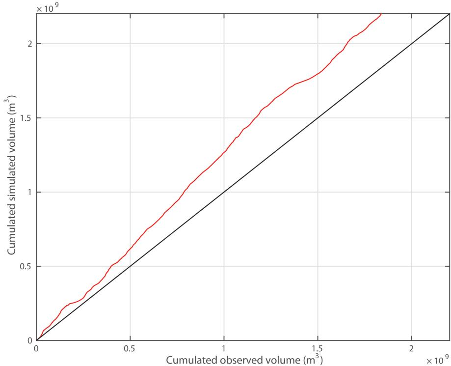
Figure 4.19. Cumulated simulated volume versus observed volume during the validation period.
