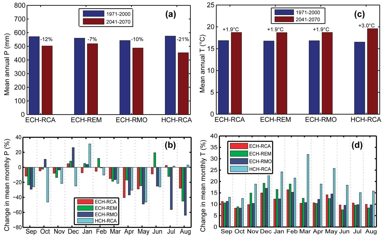
Figure 4.7. Mean annual precipitation P (a) and temperature T (c) predicted by the four climate models for the reference (1971-2000), blue bars, and future (2041-2070), red bars, periods. Relative change in mean monthly precipitation P (b) and temperature T (d) between the reference and future periods for the four climate models.
