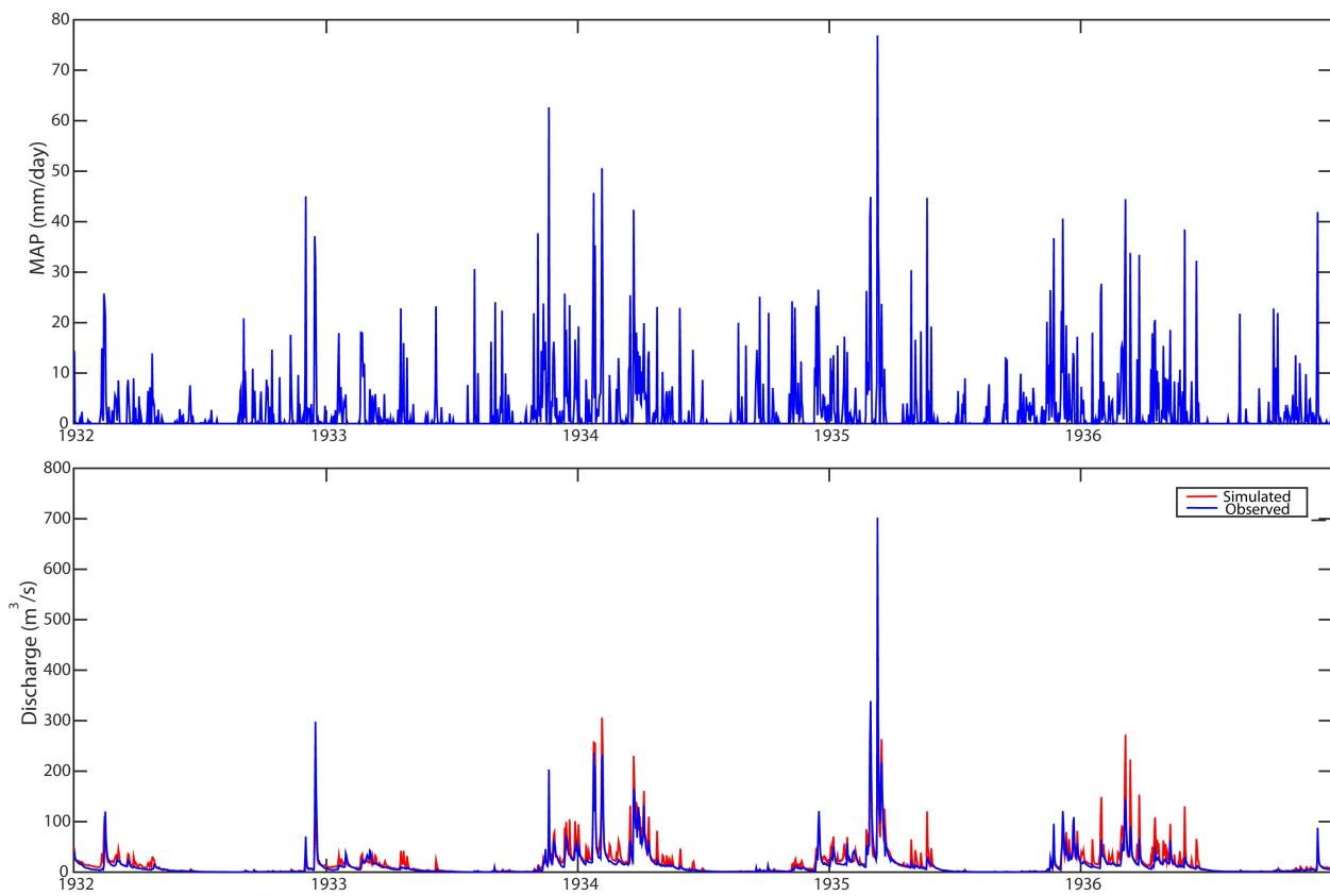
Figure 4.18. Validation simulation for the TOPKAPI-X hydrologic model applied to the Flumendosa basin. Observed discharge is compared against simulated one. In the top panel the mean areal precipitation time series computed from the 14 rain gages during the period 1932-1936 is reported.
