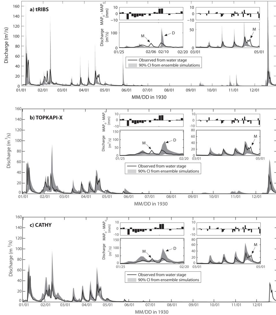
Figure 4.1. Calibration simulation for the tRIBS (a), TOPKAPI-X (b), and CATHY (c) hydrologic models applied to the Rio Mannu catchment. Observed discharge is compared against 90% confidence intervals (CI) derived from 50 ensemble simulations for each of the models. In the insets, a zoom on two periods with significant flood events is shown in order to better
