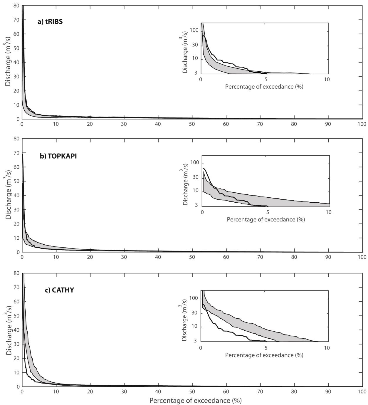
Figure 4.5. Comparison between the observed flow duration curve (FDC) and the 90% confidence intervals from the 50 ensemble simulations for the tRIBS (a), TOPKAPI-X (b), and CATHY (c) hydrologic models during the validation period (years 1931-1932).
