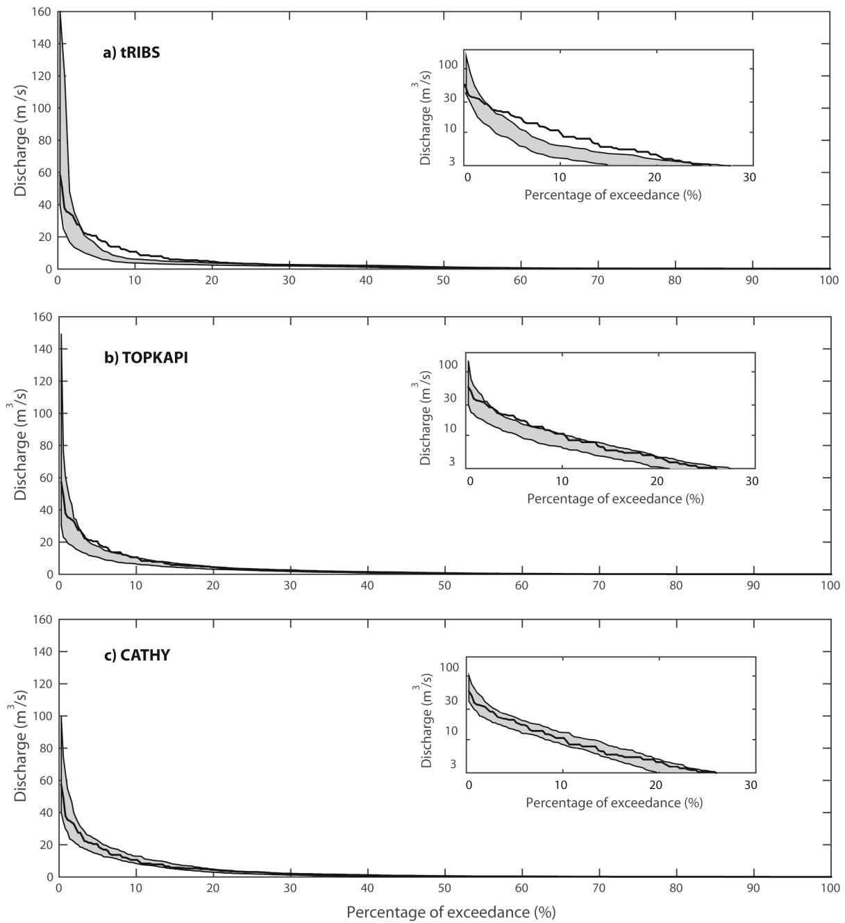
Figure 4.2. Comparison between the observed flow duration curve (FDC) and the 90% confidence intervals from the 50 ensemble simulations for the tRIBS (a), TOPKAPI-X (b), and CATHY (c) hydrologic models, during the calibration period (year 1930).
