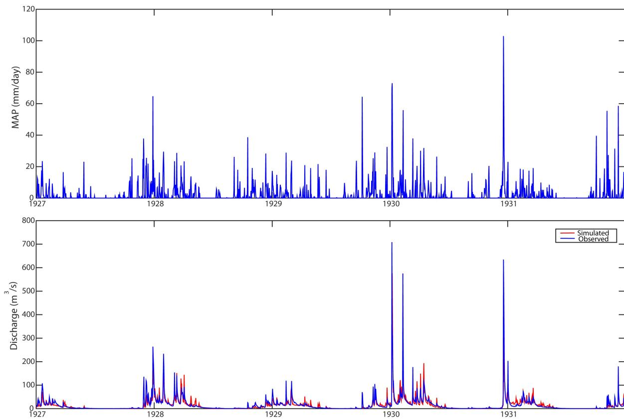
Figure 4.16. Calibration simulation for the TOPKAPI-X hydrologic model applied to the Flumendosa basin. Observed discharge is compared against simulated one. In the top panel the mean areal precipitation time series computed from the 14 rain gages during the period 1927-1931 is reported.
