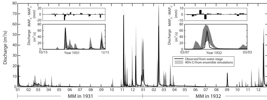
Figure 4.4. Results for the CATHY model during validation years 1931-1932 with a soil crusting assumption.
