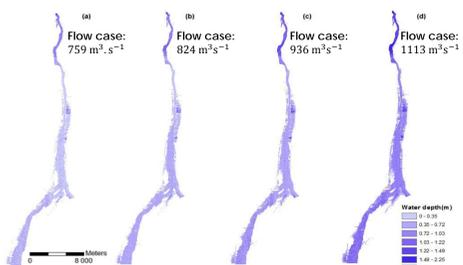
Predicted water depth with the 2D hydraulic model for four flow rates
