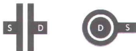
Figure 2.4: Linear and circular source and drain electrodes
